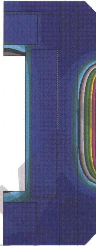
Figure 3-121. Load Case 111 – Fire at 30 Minutes, 1,475°F Ambient, Maximum Decay Heat, Cask Model – Model AOS-165
