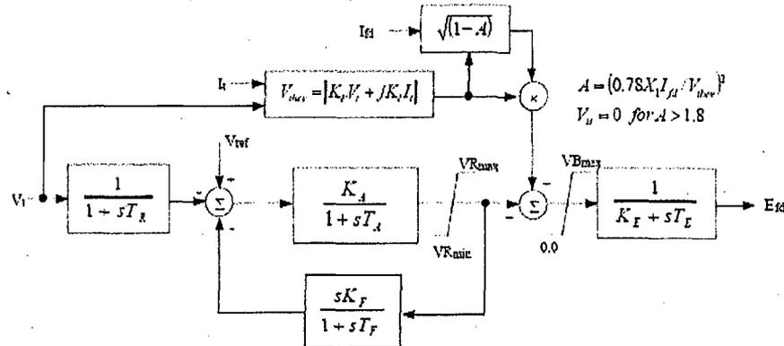
IEEE Type 3 - Static System with Terminal Potential and Current Supplies (3)
