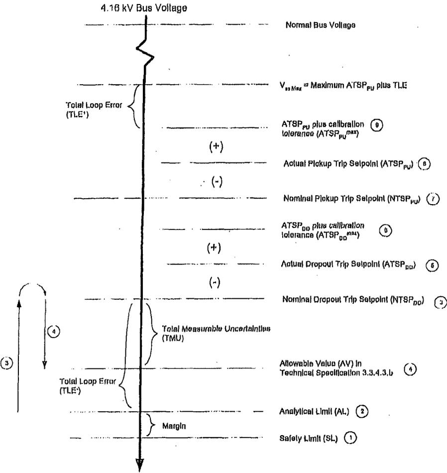
Note: The A'TSP and NTSP values shown on this Figure will be determined at the low voltage (120V) signal level in this calculation, rather than at the high voltage (4160V) signal level.
