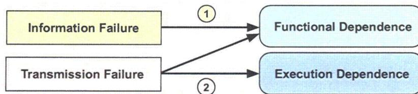
Fig. 6.2. Simple evaluation approach for safety systems communications.
