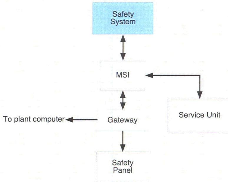
**Fig. 3.10. The MSI forms a logical boundary between the rest of the safety system and the nonsafety interfaces.**
