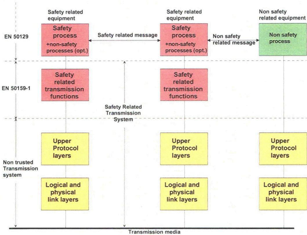
**Fig. G.4. Communication model using nontrusted closed transmission system.** *Source:* J. Alanen et al., *Safety of Digital Communications in Machines*, VTT Research Notes 2265, October 2004. Permission to use this copyrighted material is granted by J. Alanen.
