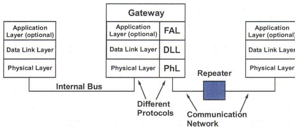
Fig. 2.5. Example of three-layer model applied to a safety system network. Gateway and repeater are present as example network features. (Adapted from IEC 61784; see Ref 41).
