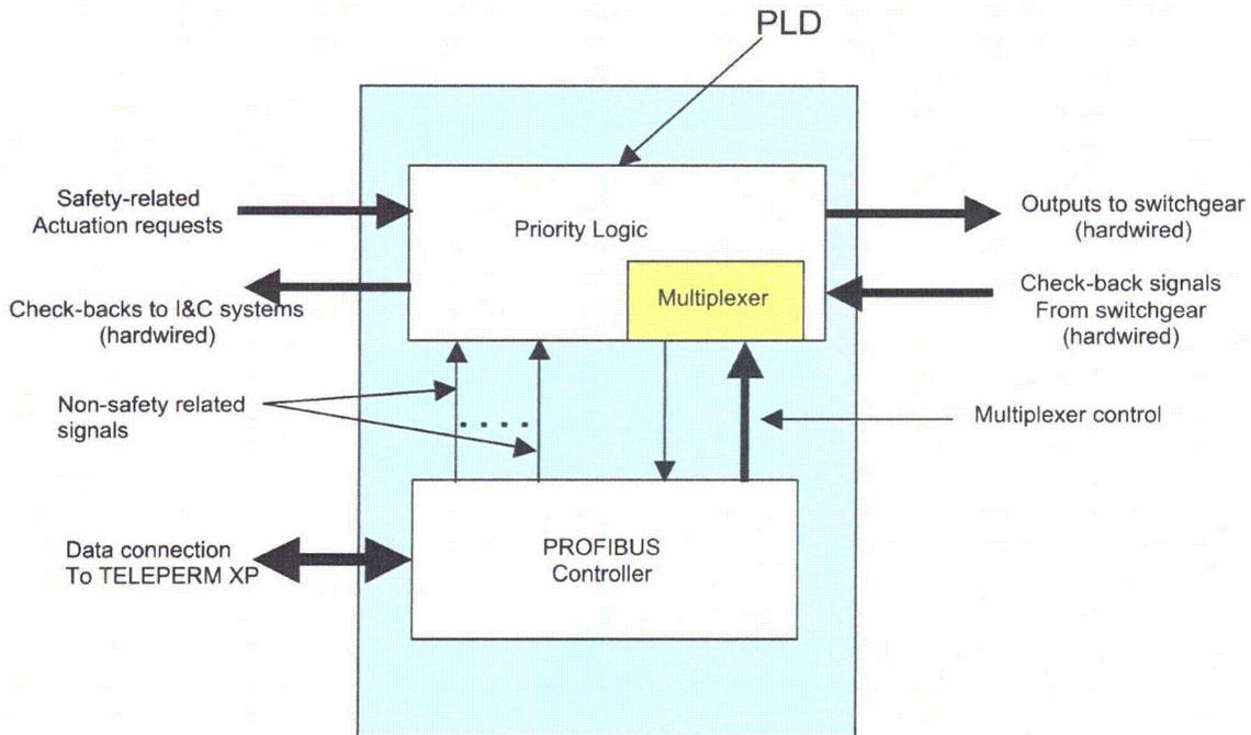
Fig. 3.9. Block diagram of Olkiluoto 3 priority and actuation module (based on Ref. 32).
