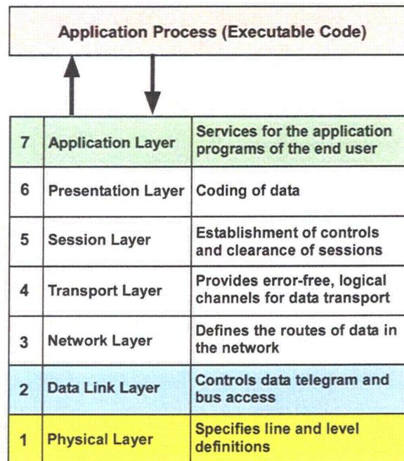
Fig. 2.3. OSI model layers and their relation to executable code.
