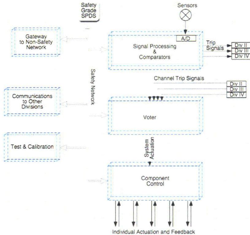
Fig. 2.2. A representative arrangement of modules in a digital protection system.
