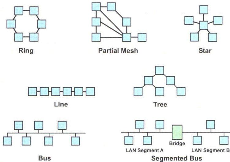
Fig. 2.4. Typical communications network topologies.
