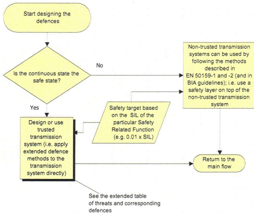
**Fig. G.3. Detail of design section of analysis flow chart.** Source: J. Alanen et al., *Safety of Digital Communications in Machines*, VTT Research Notes 2265, October 2004. Permission to use this copyrighted material is granted by J. Alanen.
