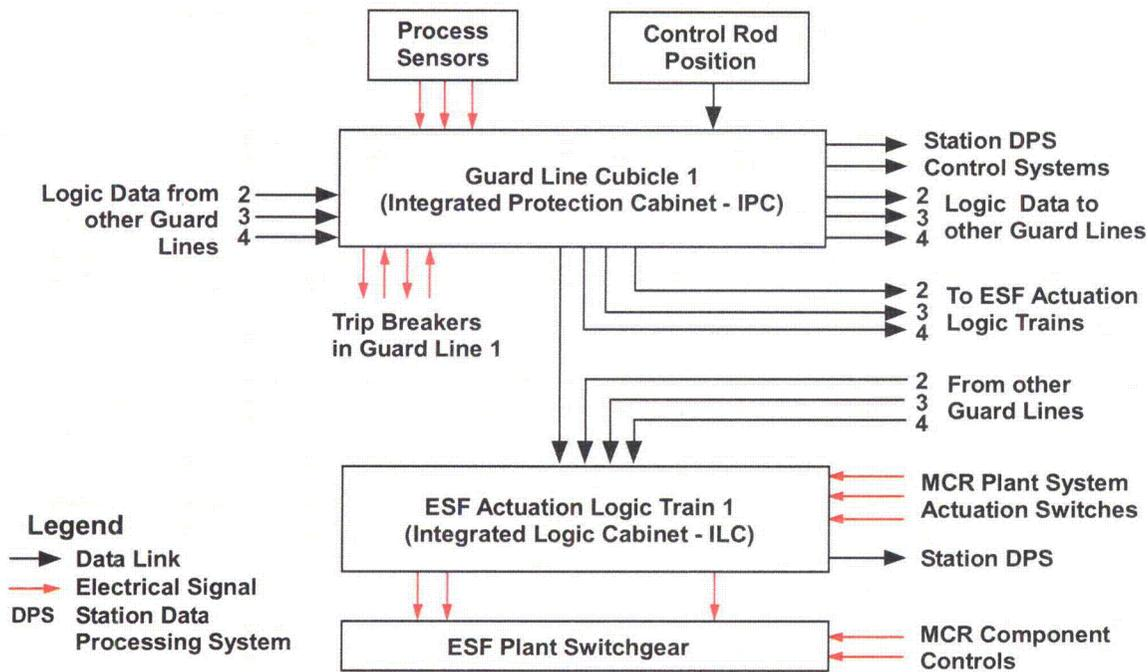
Fig. 3.2. Sizewell B protection system diagram illustrating communications within a division. Adapted from G. B. Moutrey and G. Remley, “Sizewell B power station primary protection system design application overview: Electrical and Control Aspects of the Sizewell B PWR,” International Conference on 14–15 September 1992, p. 221–231.
