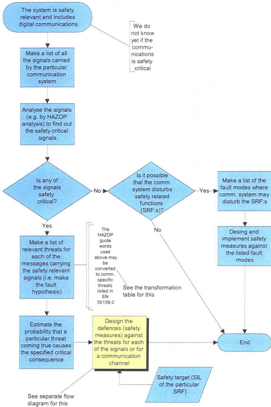
**Fig. G.2. Flow chart illustrating safety analysis of digital communications network.** Source: J. Alanen et al., *Safety of Digital Communications in Machines*, VTT Research Notes 2265, October 2004. Permission to use this copyrighted material is granted by J. Alanen.
