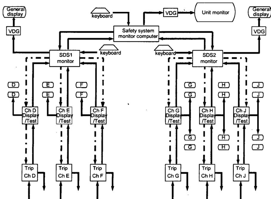
Fig. 3.4. Reactor protection system architecture.
