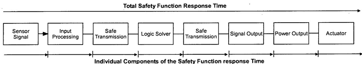
Fig. 4.3. Example of safety-function response time components.
