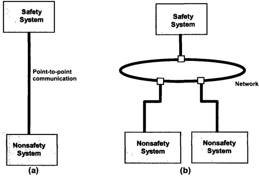
Fig. 1.1. Typical communication structures within the scope of this document.
