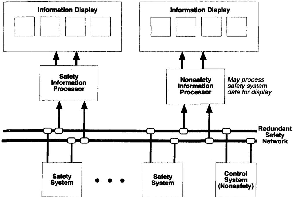
Fig. 1.2. Simplified generic I&C architecture for sending safety system information to multidivisional display stations.
