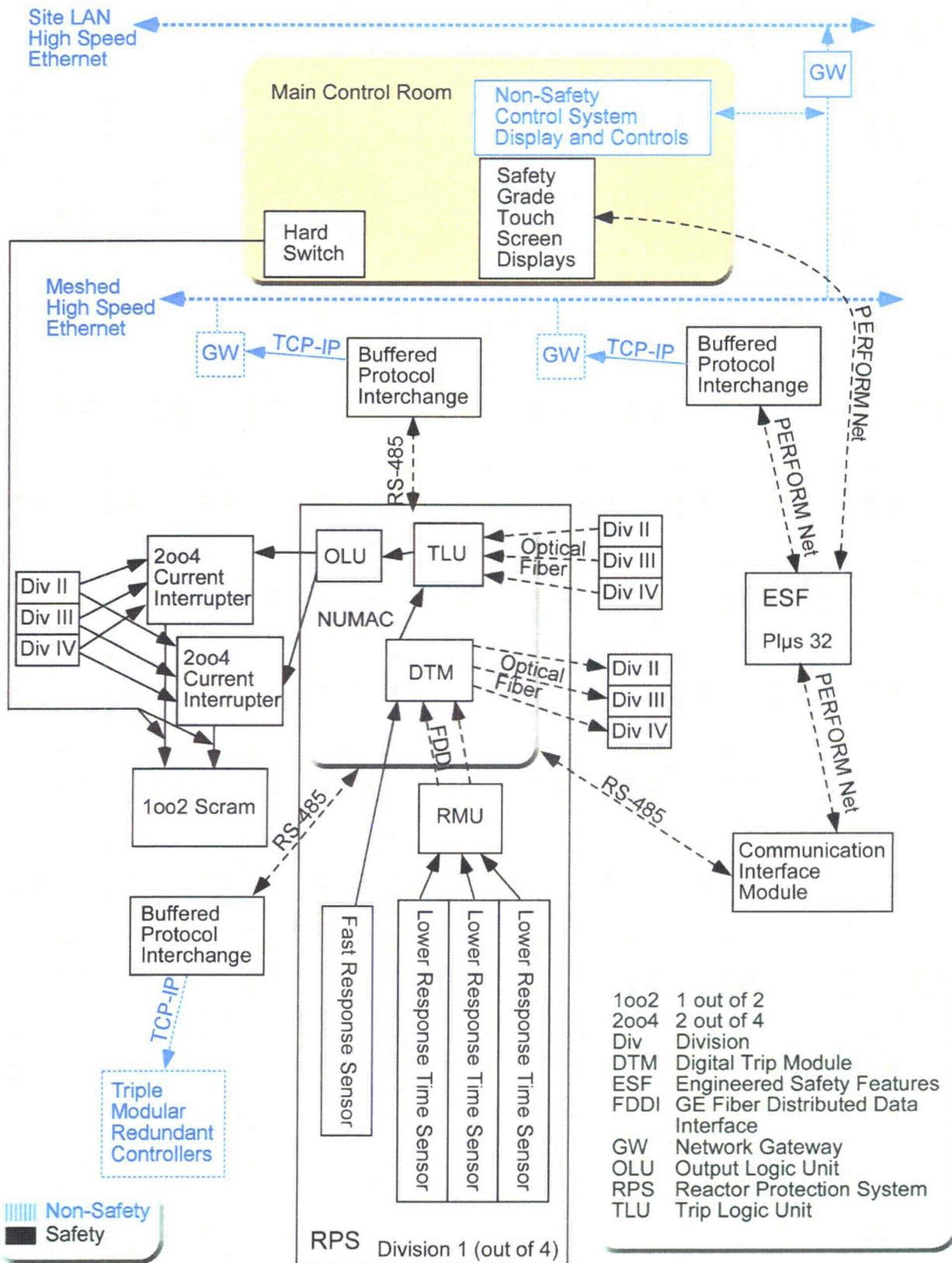
Fig. 3.5. Lungmen reactor protection system communications paths and protocols.
