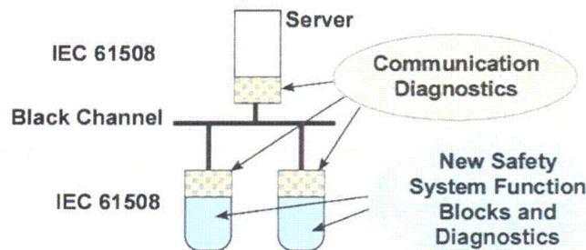
Fig. 4.5. Illustration of black channel implementation.
