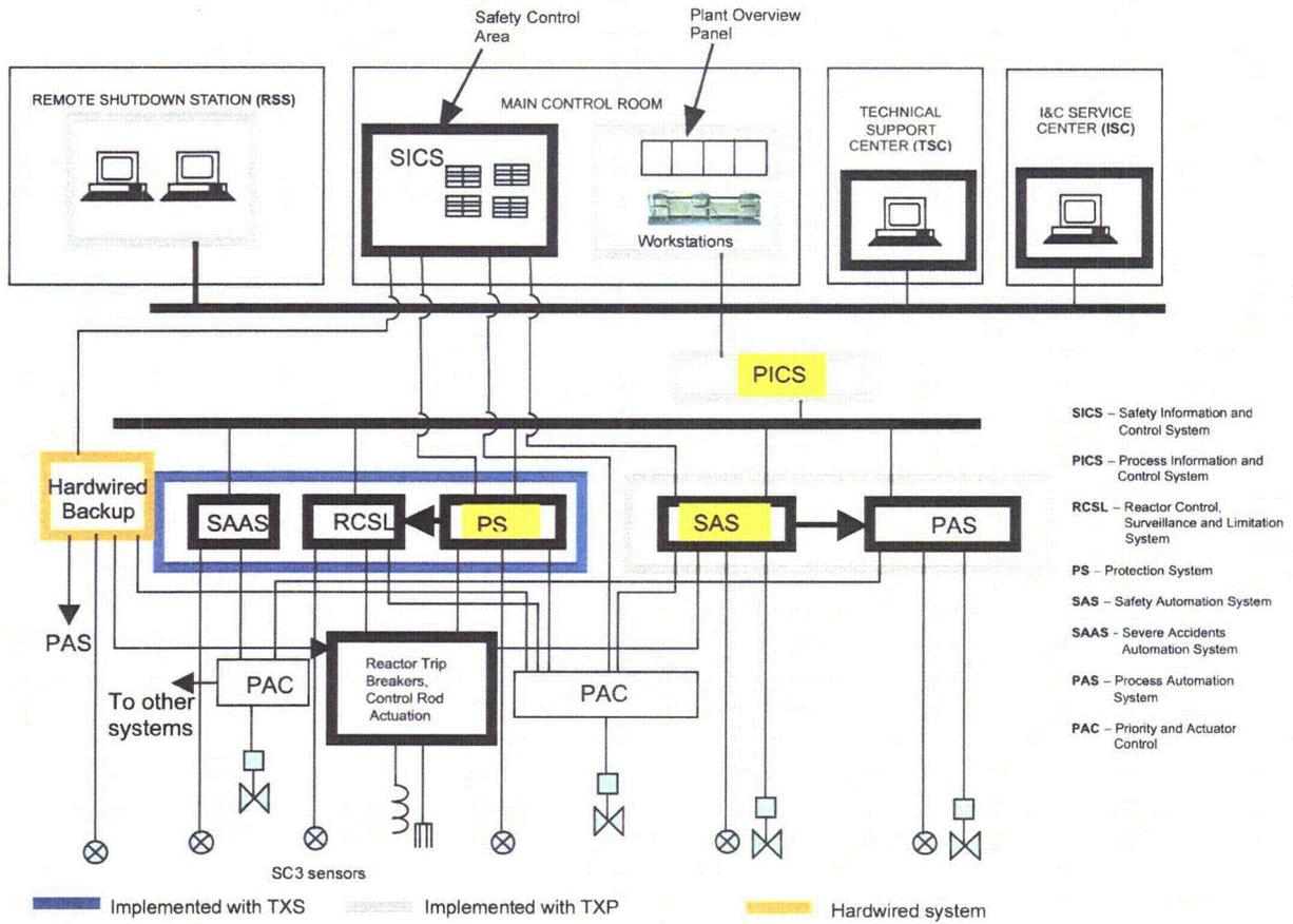
Fig. 3.8. Olkiluoto 3 I&C architecture. Adapted from J. Hyvarinen, STUK (see Ref. 32).
