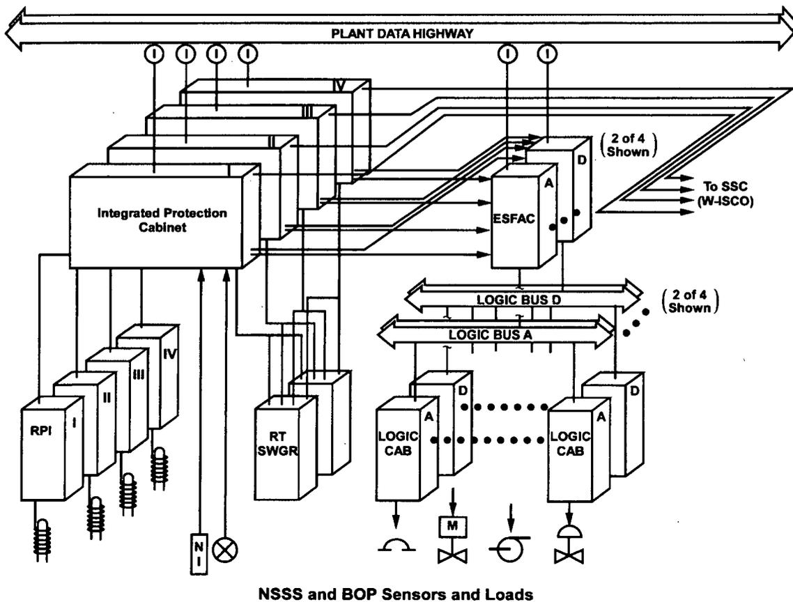
**Fig. 3.3. Sizewell B primary protection system.** Adapted from G. W. Remley, B. M. Cook, and P. A. Loftus, "Sizewell B Integrated Control and Instrumentation System: A Vision Becomes Reality," IEEE 0-7803-0883-2/93.
