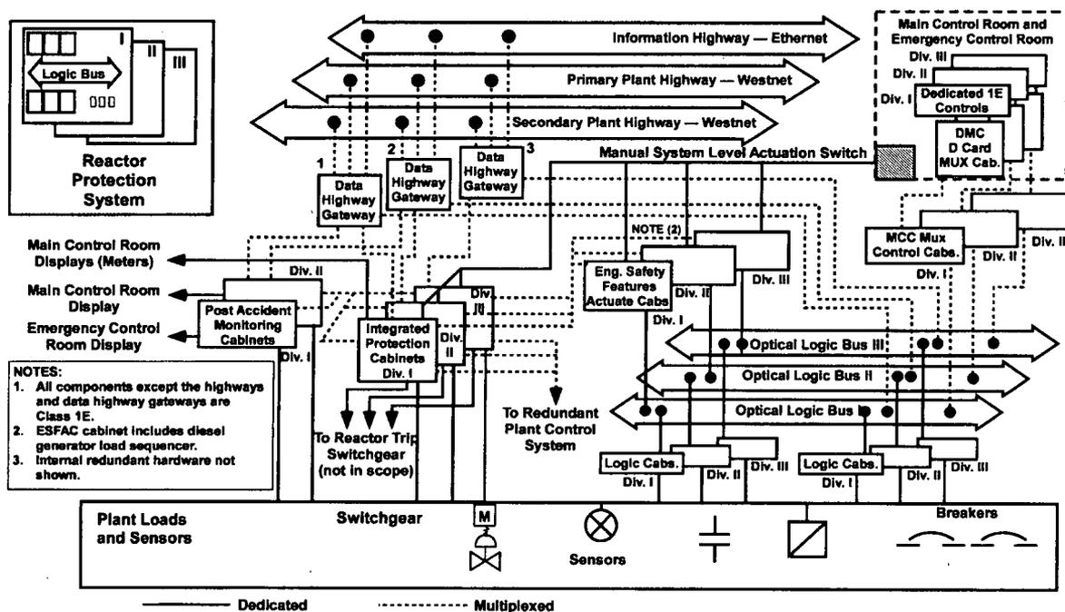
Fig. 3.7. Temelin reactor protection system. Adapted from W. C. Gangloff and C. L. Werner, "I&C Modernization for VVER Reactors," *IEEE Transactions on Nuclear Science* 40(4), 819-825 (August 1993).
