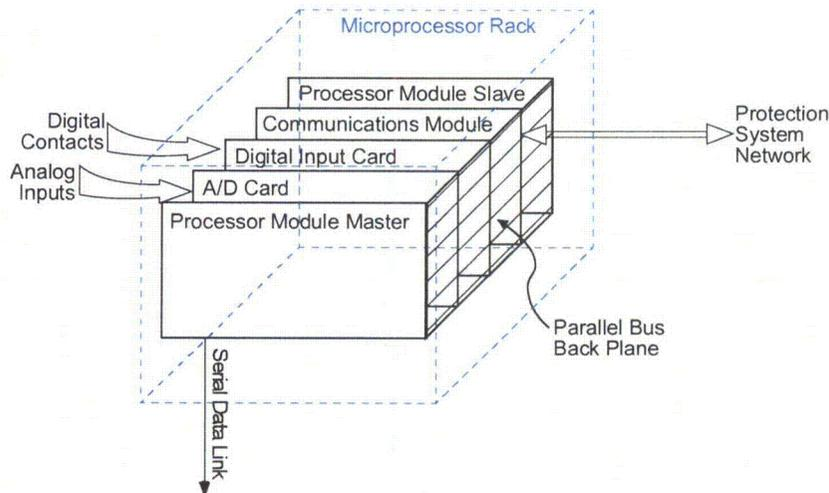
**Fig. 2.1. Generic microprocessor-based rack.**
