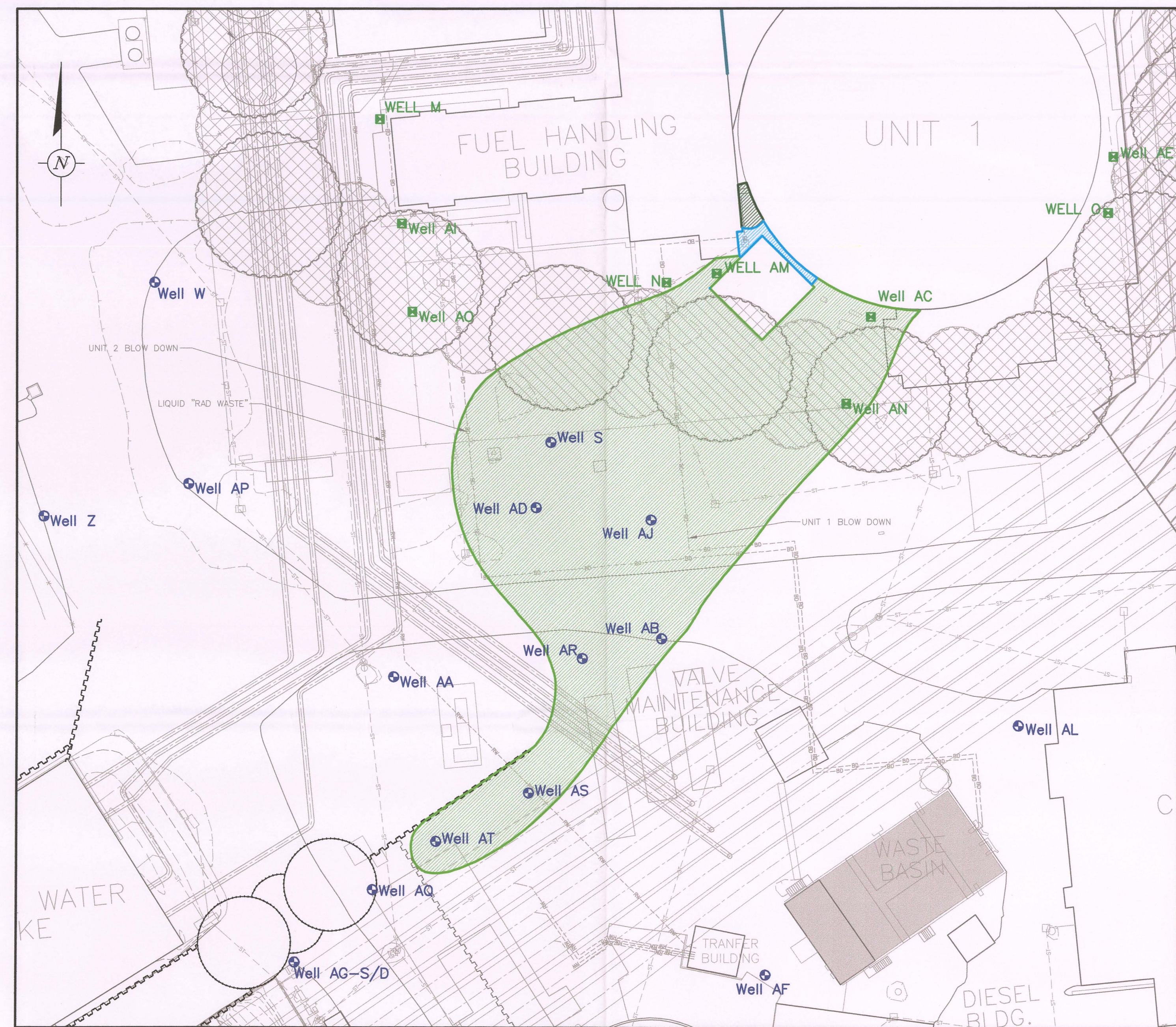
TRITIUM PLUME - MARCH 2008 FULL SCALE SYSTEM IN SERVICE SCALE: 1"=30'
