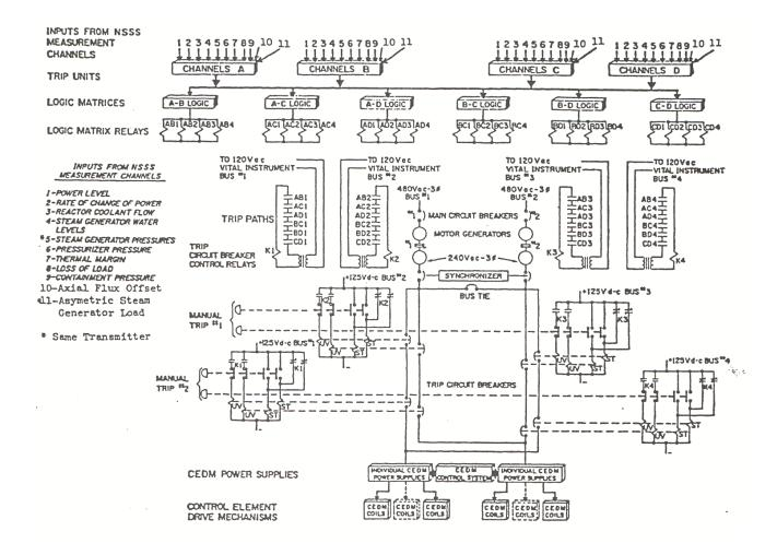
Figure B 3.3.1-1 Functional Diagram of the Two-Out-of-Four Logic and RTCB Configuration
