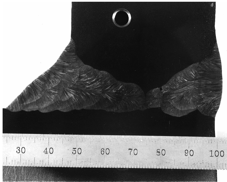
Figure 4.3.1.4-2. Cross section of Weld in Mockup BWRVIP-B
