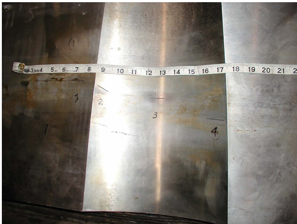
Figure 4.3.1.8-2. Mockup BWRVIP-SSC1; Detail of Notches 1-4
