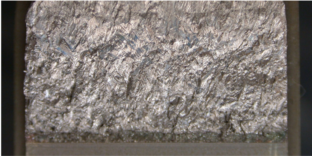
Figure 11. Macro photograph of Alloy 22 CT-String defect specimen CTS 13. To achieve 20 ksi√in, the fatigue precrack length is quite short ( a/W=0.420 ), and the crack exposed to the test environment is the thin area just above the smooth machined notch. The specimen width is 0.5 inch.
