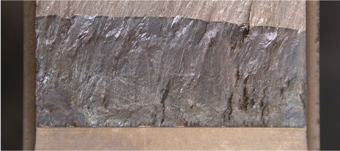
Figure 9. Macro photograph of Alloy 22 CT-String defect specimen CTS 05. To achieve 30 ksi√in, the fatigue precrack length is quite long ( a/W=0.554 ), and the crack exposed to the test environment is the large tinted area just above the smooth machined notch. The specimen width is 0.5 inch.
