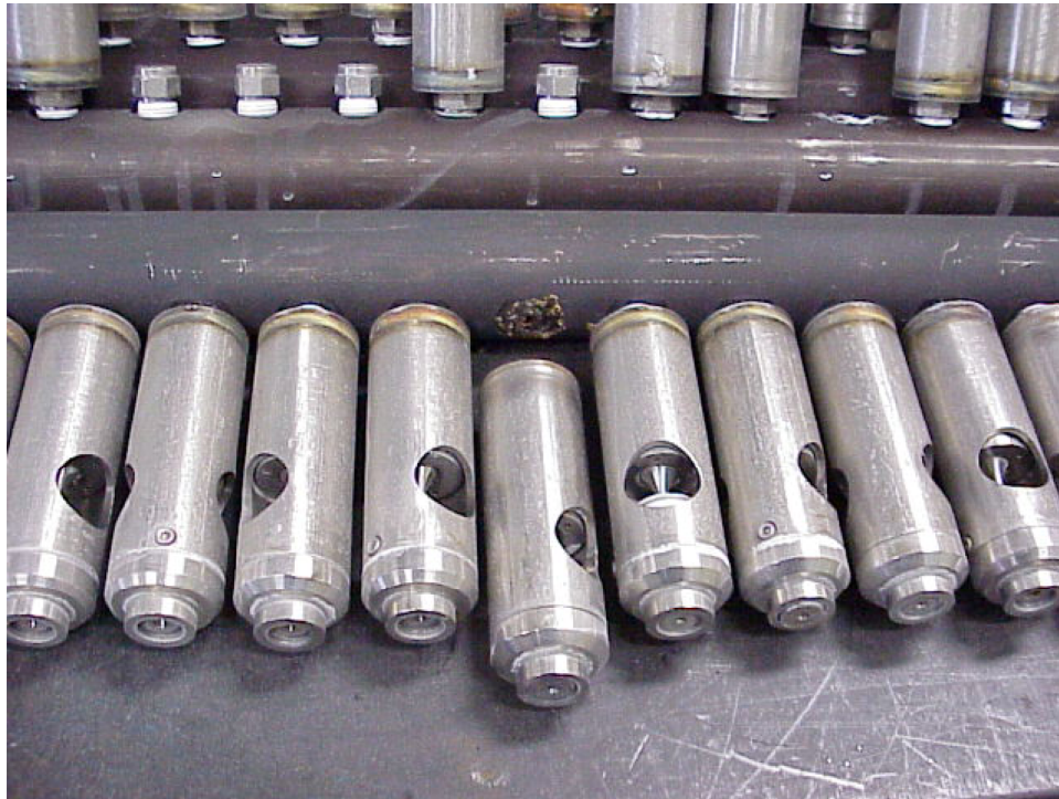
Figure 8. Corroded and fractured threads at the module/manifold interface produced unacceptably high leakage rates from the Keno autoclave. Three 316L stainless steel manifolds were ordered and manufactured to replace the 304 stainless steel manifolds damaged by corrosion during Keno Run 2, and subsequently Alloy 825 has been used.
