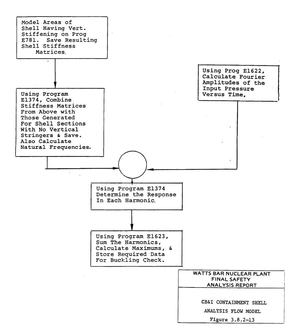
Figure 3.8.2-13 CB & I Containment Shell Analysis Flow Model
