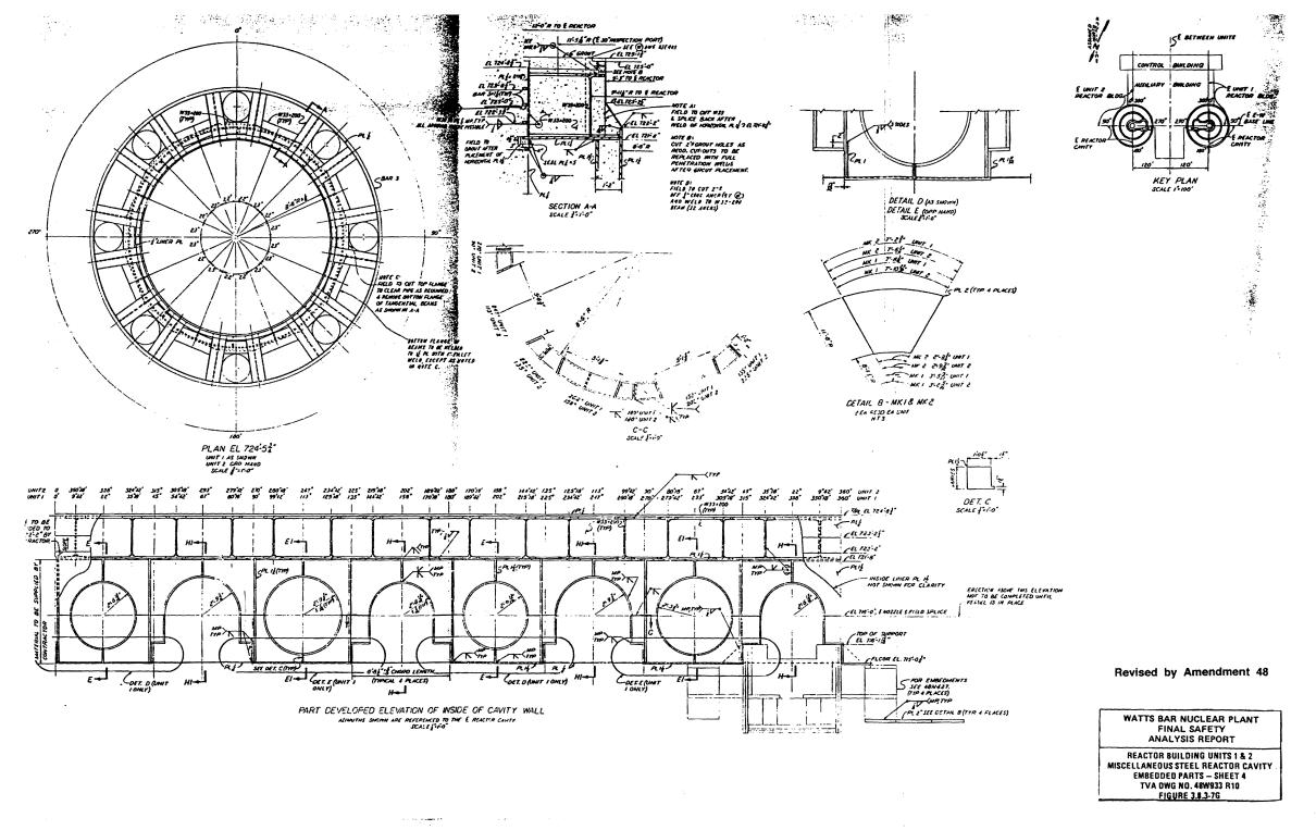
Figure 3.8.3-7g Reactor Building Units 1 & 2 - Miscellaneous Steel Reactor Cavity Embedded Parts - Sheet 4
