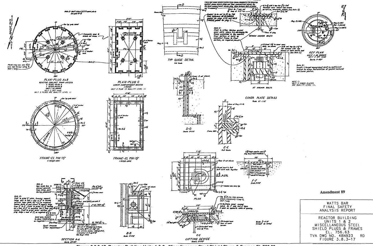
Figure 3.8.3-17 Reactor Building Units 1 & 2 - Miscellaneous Steel Shield Plugs & Frames El. 756.63
