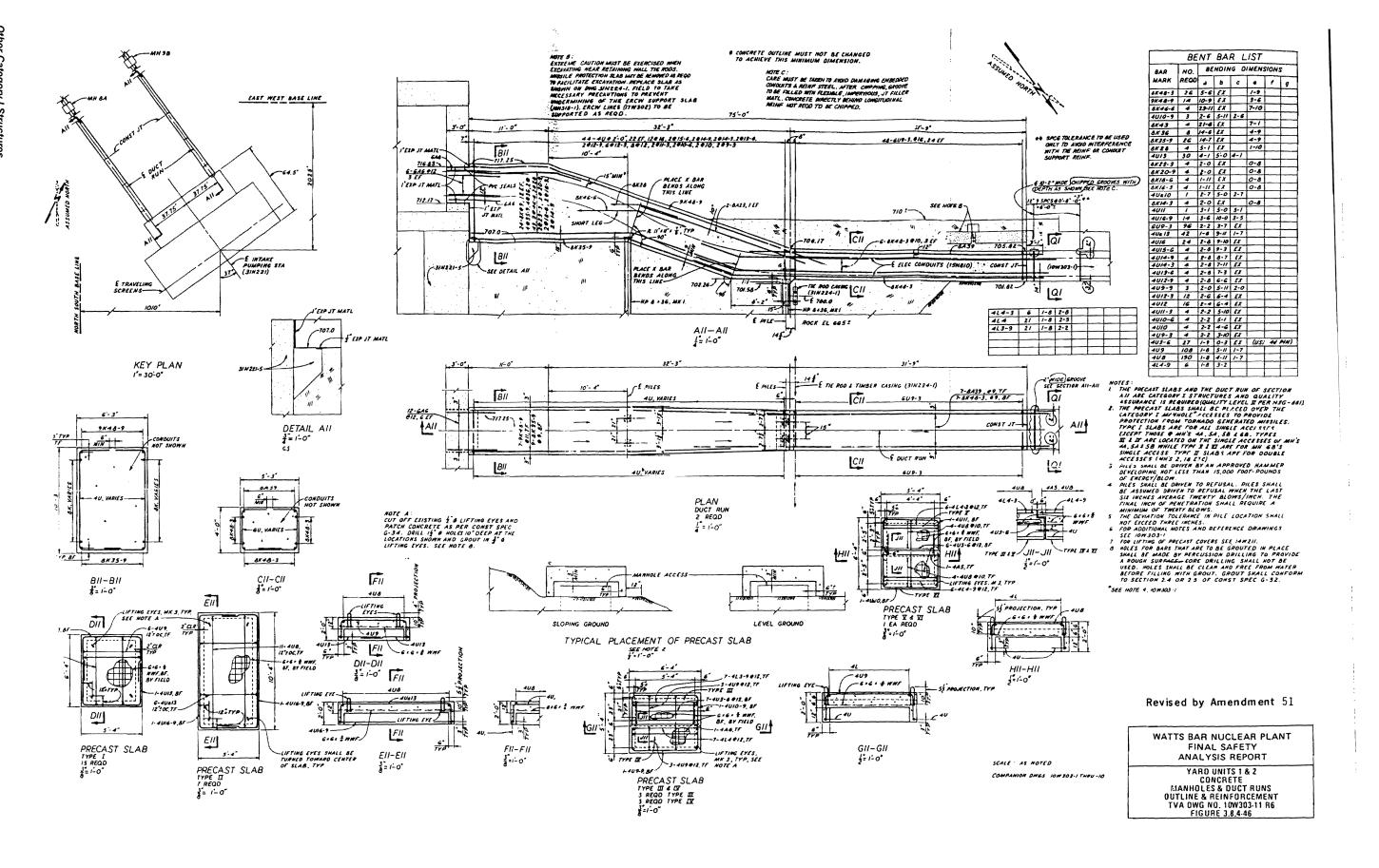
Figure 3.8.4-46 Yard Units 1 & 2 Concrete Manholes & Duct Runs Outline & Reinforcement
