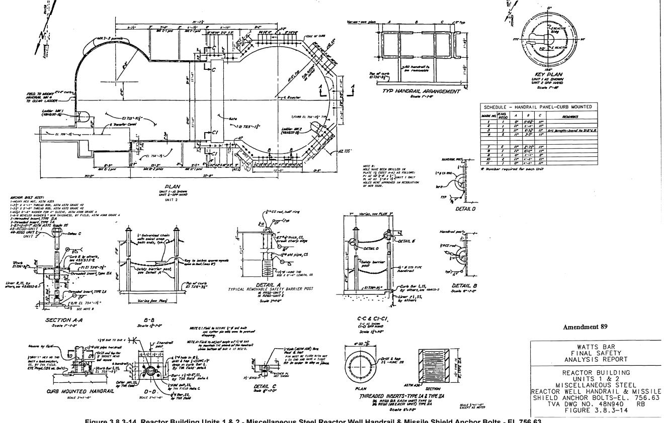
Figure 3.8.3-14 Reactor Building Units 1 & 2 - Miscellaneous Steel Reactor Well Handrail & Missile Shield Anchor Bolts - EL 756.63
