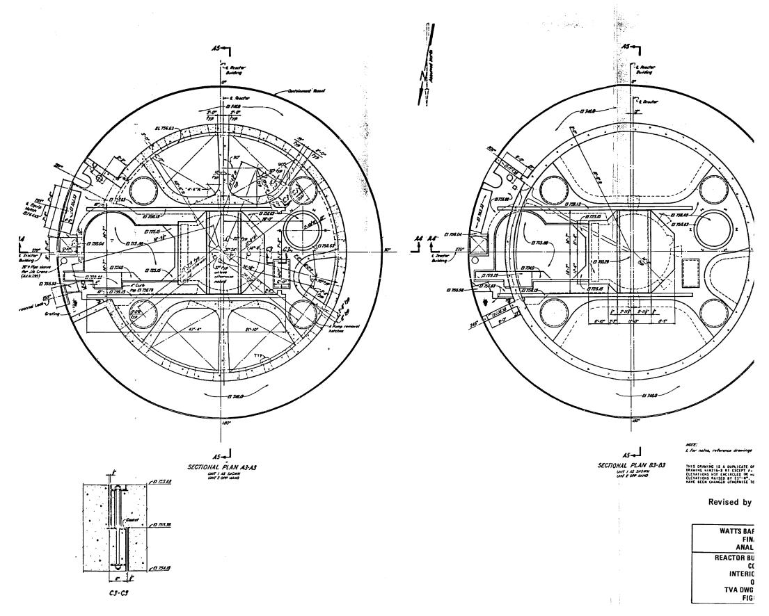
Figure 3.8.3-3 Reactor Building Units 1 & 2; Concrete Interior Structure Outline
