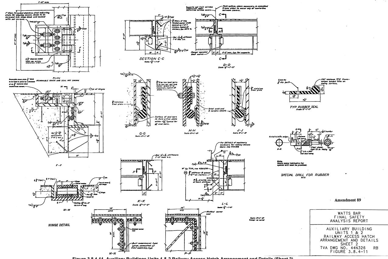
Figure 3.8.4-11 Auxiliary Buildings Units 1 & 2 Railway Access Hatch Arrangement and Details (Sheet 2)
