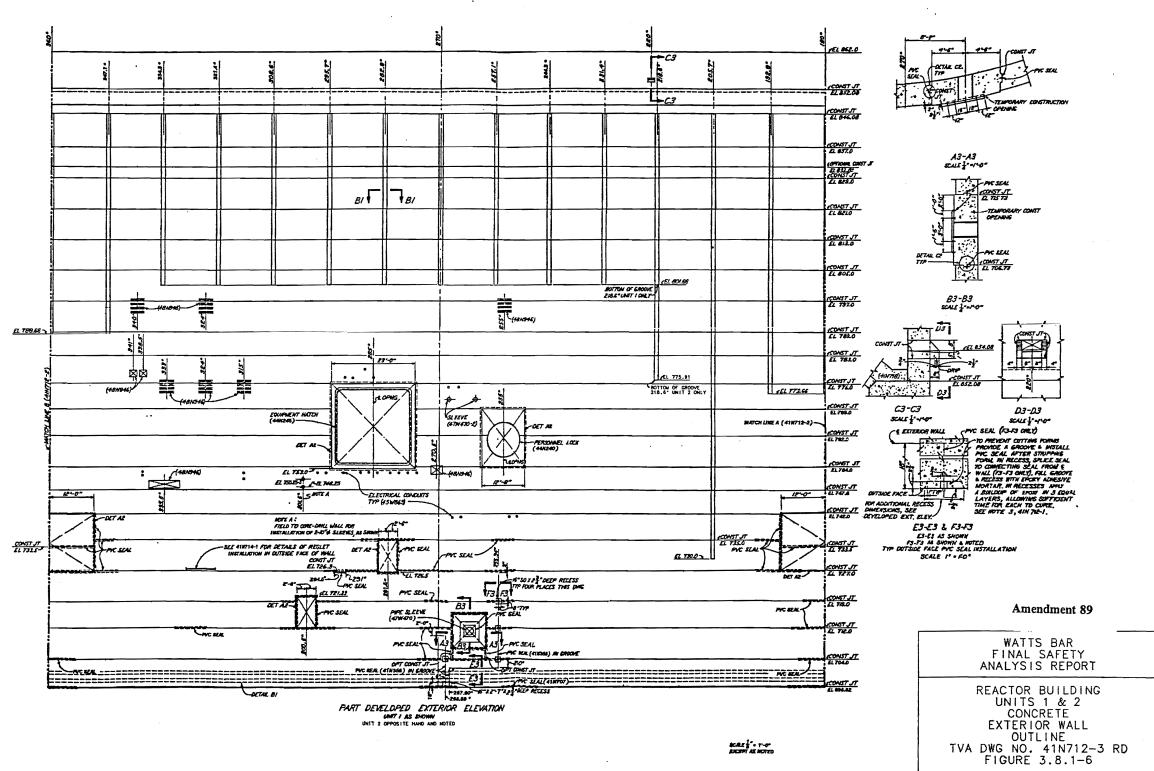
Figure 3.8.1-6 Concrete Exterior Wall Outline
