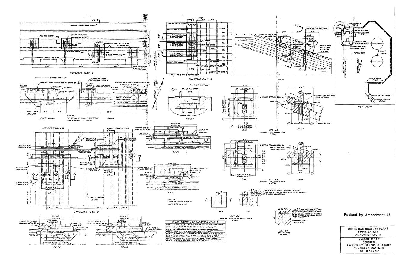
Figure 3.8.4-56c Yard Units 1 & 2 Concrete ERCW Structures Outline & Reinforcement
