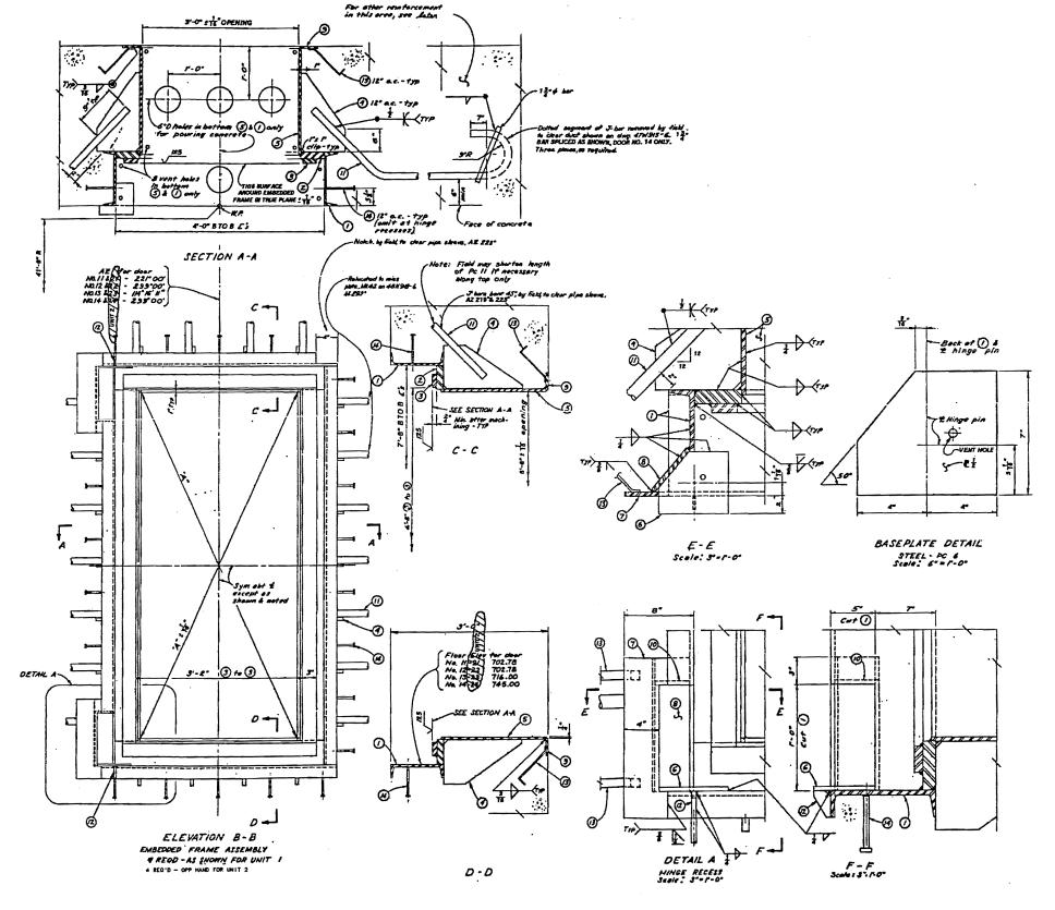
Figure 3.8.3-11 Reactor Building Units 1 & 2 - Personnel Access Doors Thru Crane Wall Embedded Frame
