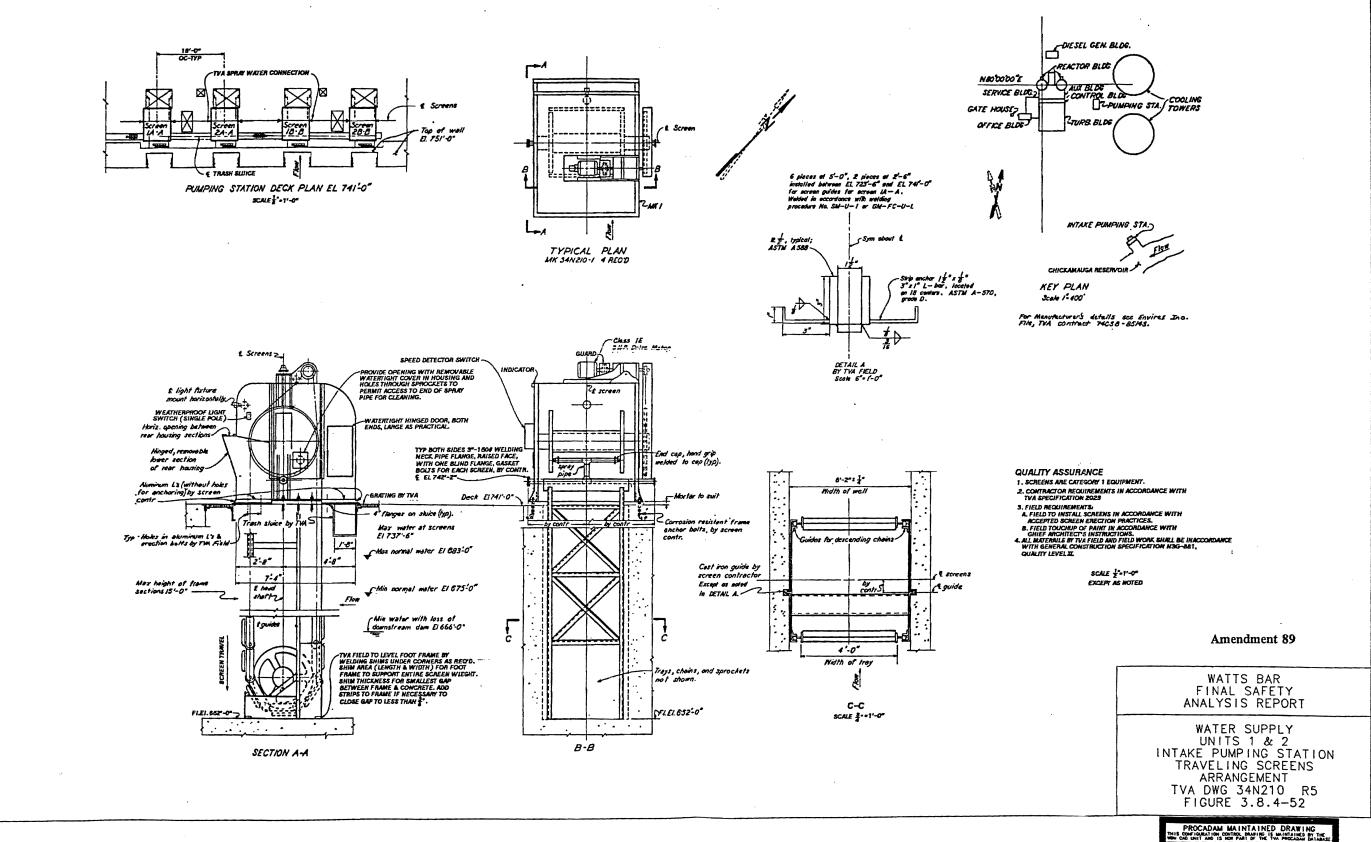
Figure 3.8.4-52 Water Supply Units 1 & 2 Intake Pumping Station Traveling Screens Arrangement
