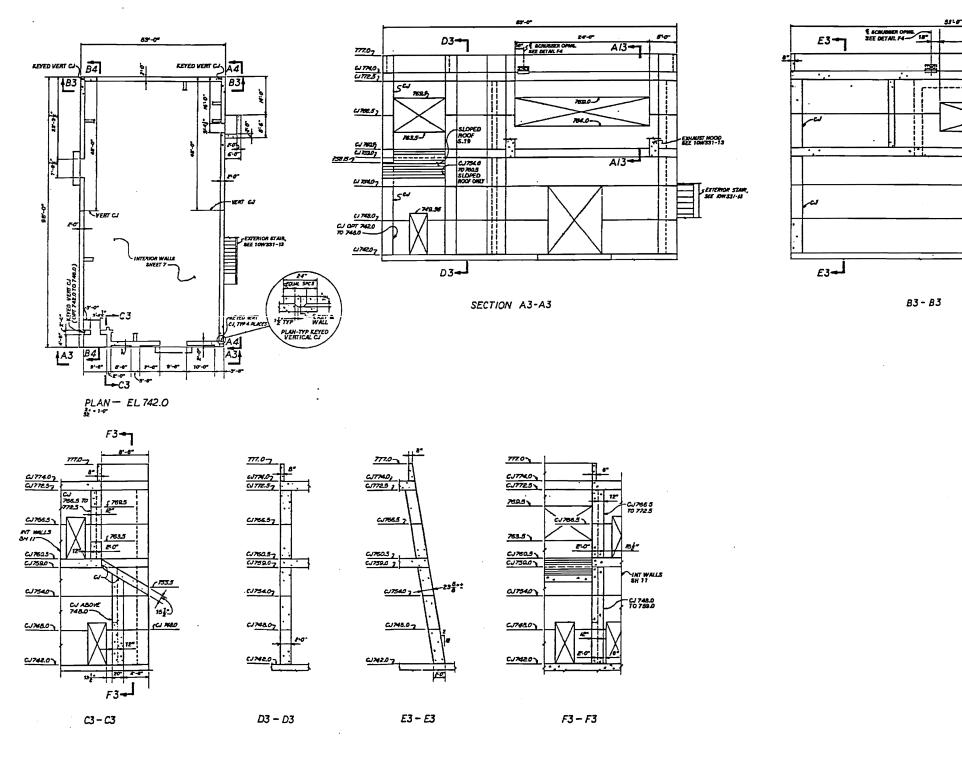
Figure 3.8.4-74 Yard Additional Diesel Generator Building Concrete Exterior Walls Outline
