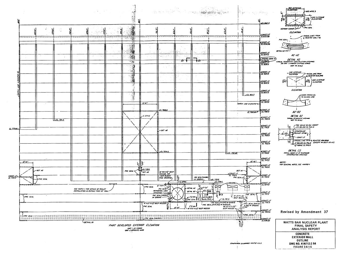
Figure 3.8.1-5 Concrete Exterior Wall Outline
