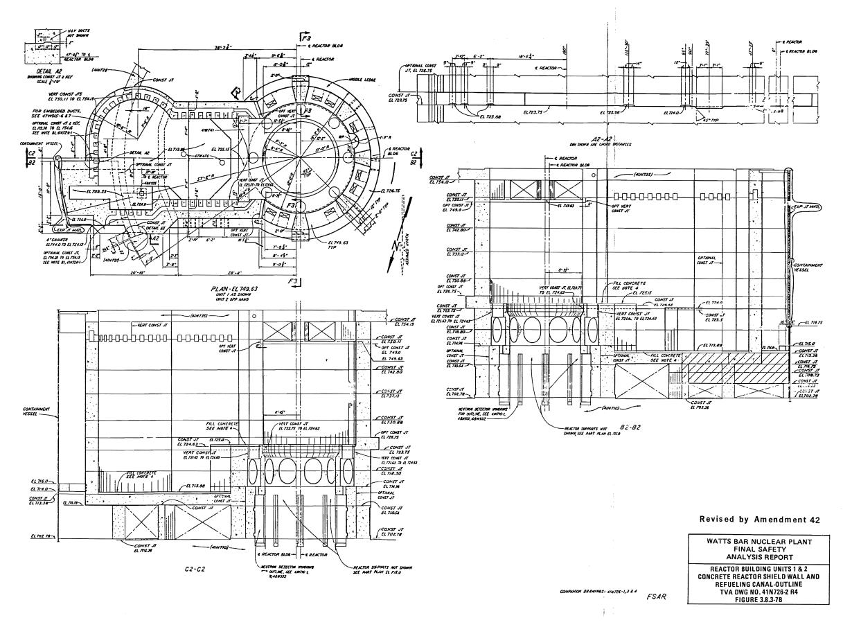
Figure 3.8.3-7b Reactor Building Units 1 & 2 - Concrete Reactor Shield Wall and Refueling Canal - Outline
