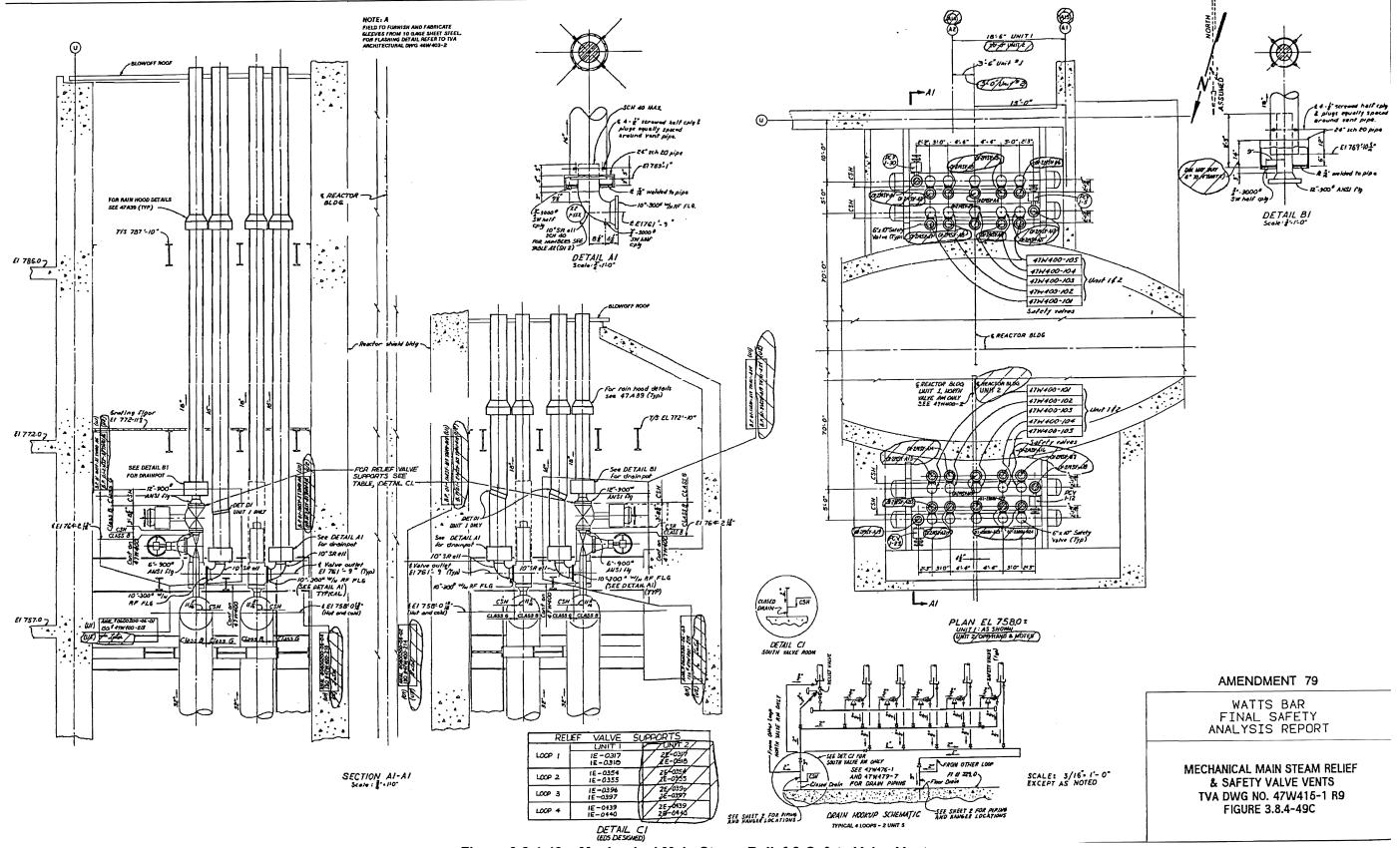
Figure 3.8.4-49c Mechanical Main Steam Relief & Safety Valve Vents
