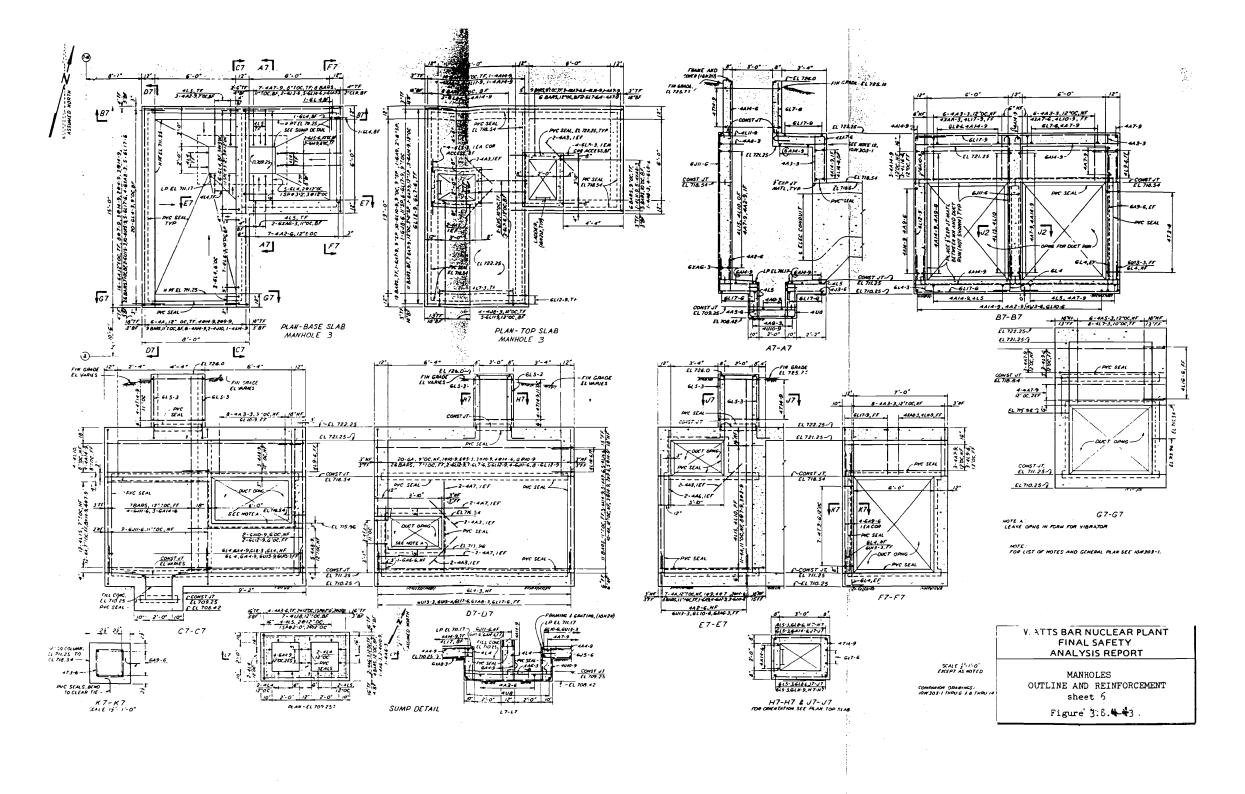
Figure 3.8.4-43 Manholes Outline and Reinforcement (Sheet 6)
