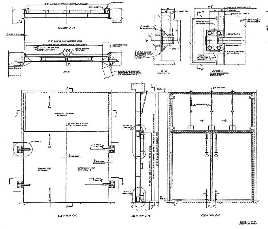
Figure 3.8.4-30 Diesel Generator Building Units 1 & 2 Doors & Bulkhead Arrangement
