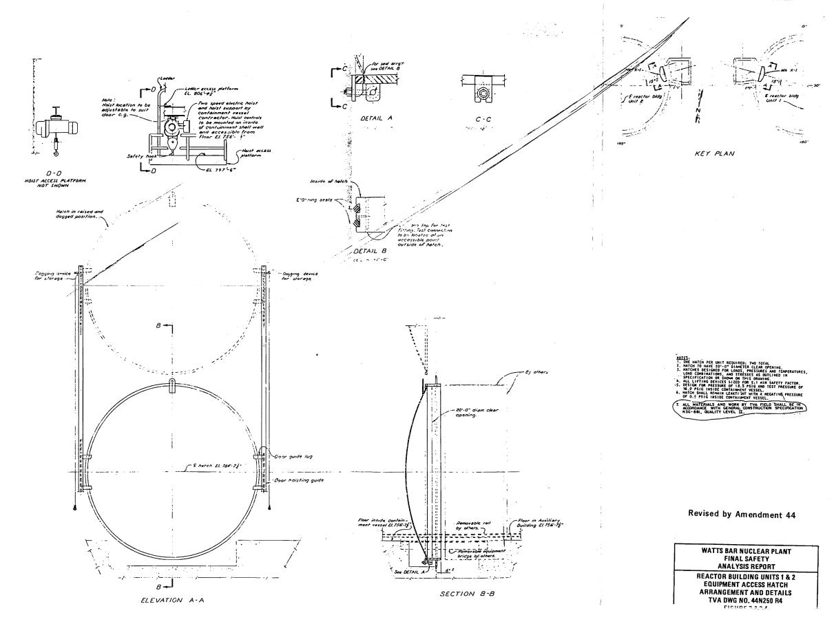
Figure 3.8.2-4 Equipment Access Hatch Arrangement and Details
