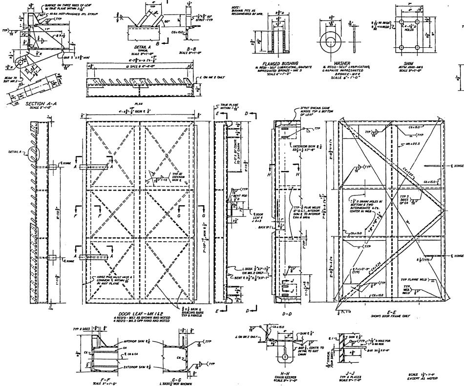
Figure 3.8.4-31 Diesel Generator Building Units 1 & 2 Doors and Bulkhead Details (Sheet 1)
