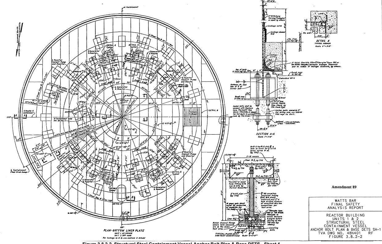
Figure 3.8.2-2 Structural Steel Containment Vessel-Anchor Bolt Plan & Base DETS - Sheet 1
