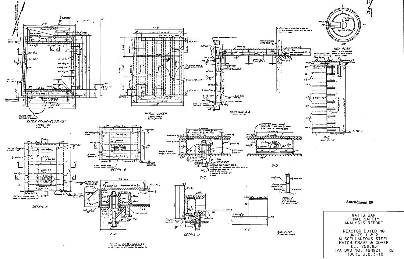
Figure 3.8.3-18 Reactor Building Units 1 & 2 - Miscellaneous Steel Hatch Frame and Cover EL. 756.63
