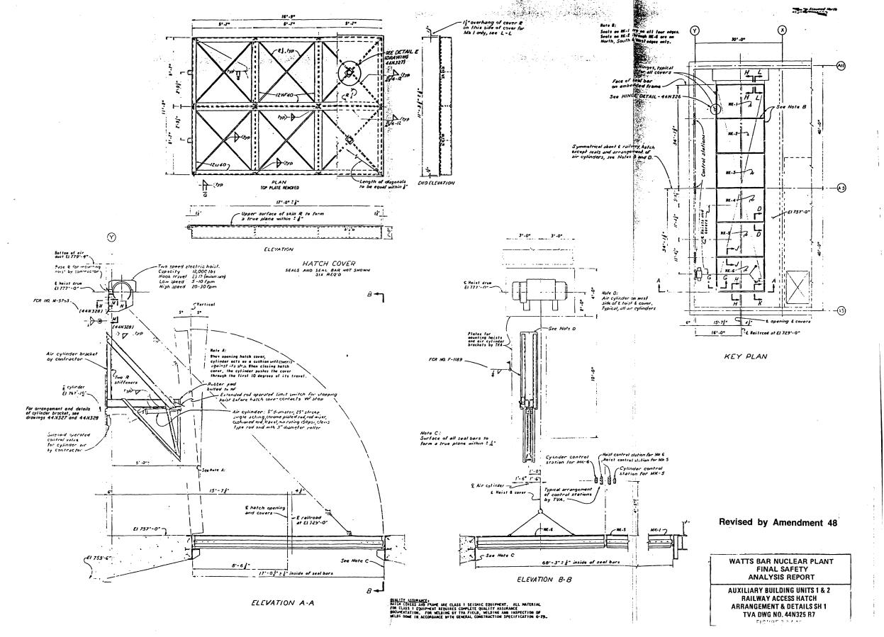
Figure 3.8.4-10 Auxiliary Buildings Units 1 & 2 Railway Access Hatch Arrangement & Details (Sheet 1)
