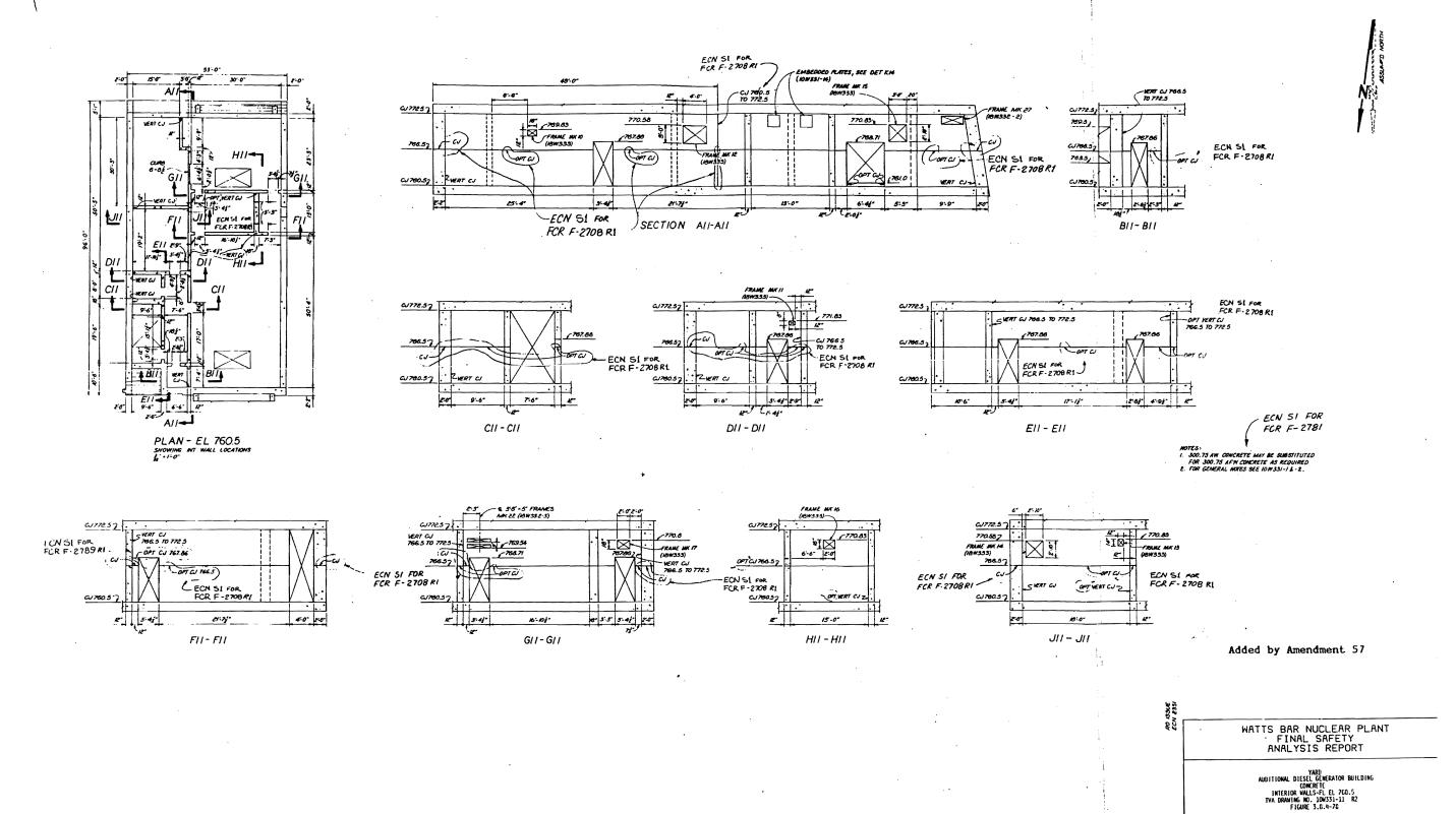
Figure 3.8.4-78 Yard Additional Diesel Generator Building Concrete Interior Walls-FL EL. 760.5
