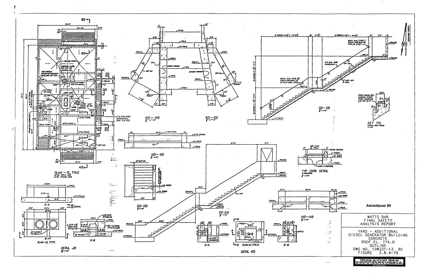
Figure 3.8.4-79 Yard Additional Diesel Generator Building Concrete Roof EL. 774.0 Outline
