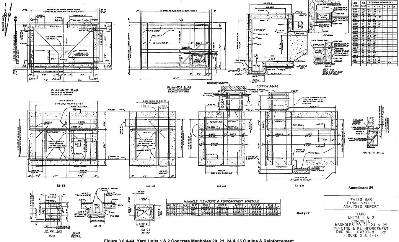
Figure 3.8.4-44 Yard Units 1 & 2 Concrete Manholes 20, 21, 24 & 25 Outline & Reinforcement
