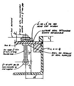
SECTION A-A NR SUPPLY Scale 6"=1"-0"
