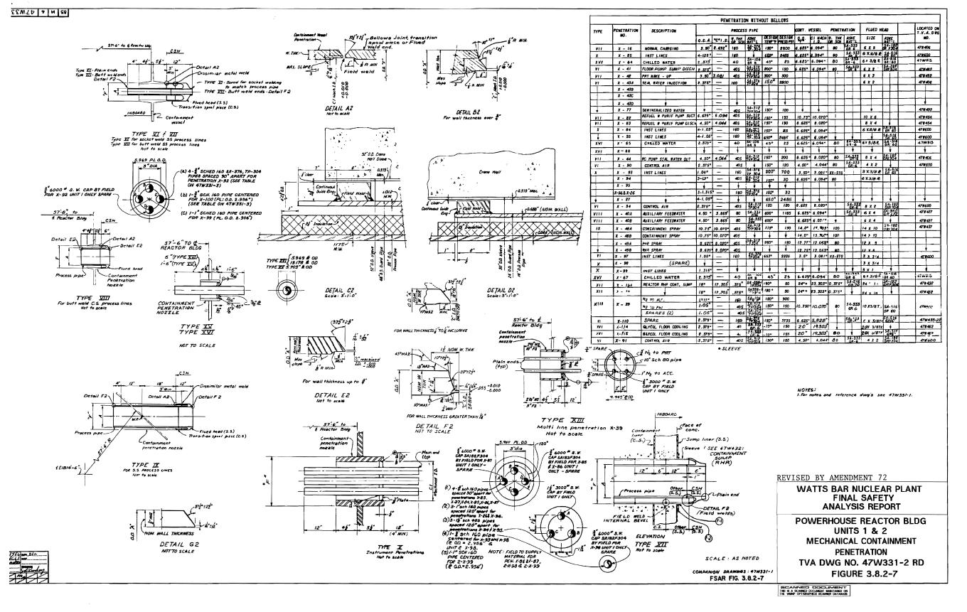
Figure 3.8.2-7 Mechanical Containment Penetration
