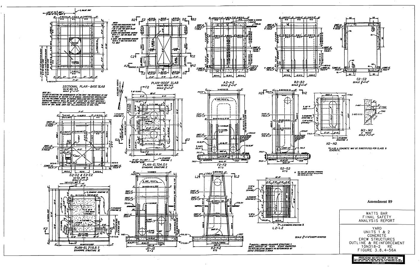
Figure 3.8.4-56a Yard Units 1 & 2 Concrete ERCW Structures Outline & Reinforcement
