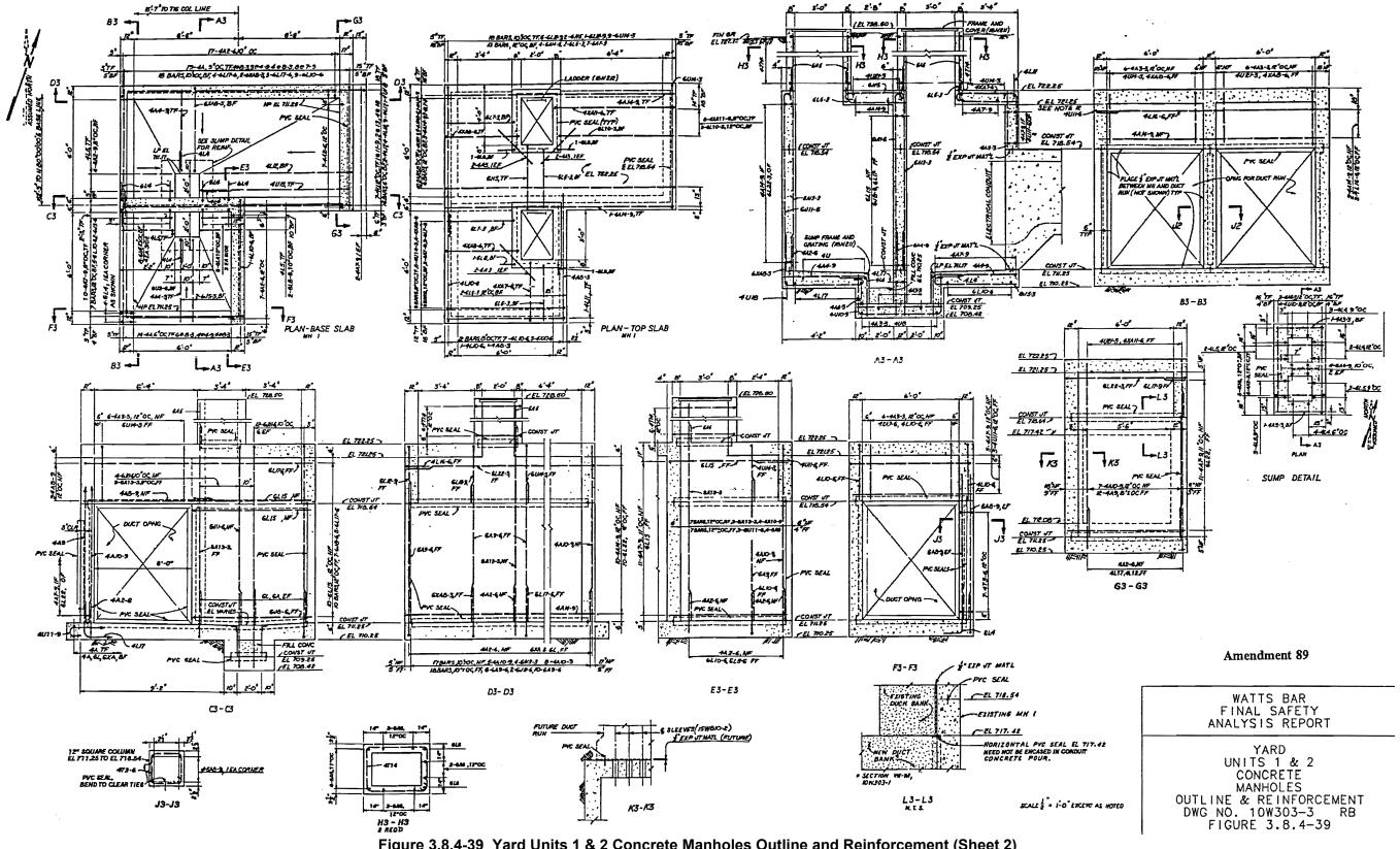
Figure 3.8.4-39 Yard Units 1 & 2 Concrete Manholes Outline and Reinforcement (Sheet 2)
