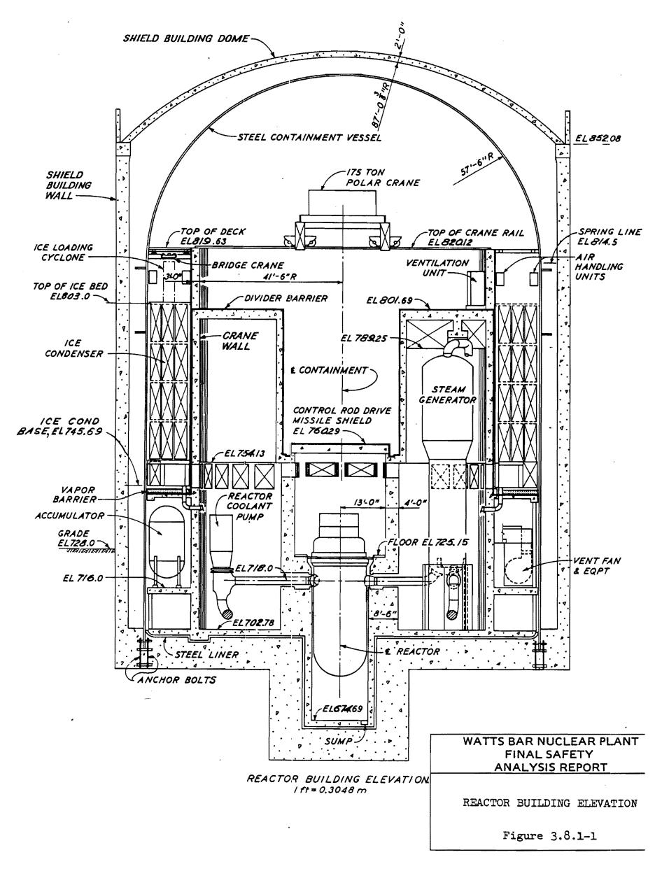
Figure 3.8.1-1 Reactor Building Elevation
