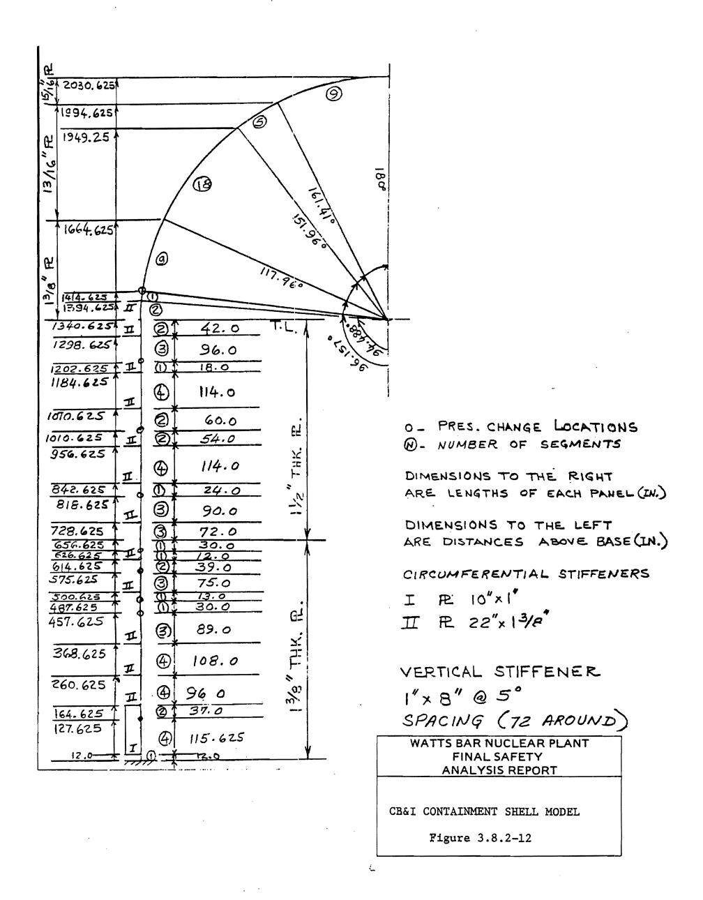
Figure 3.8.2-12 CB & I Containment Shell Model
