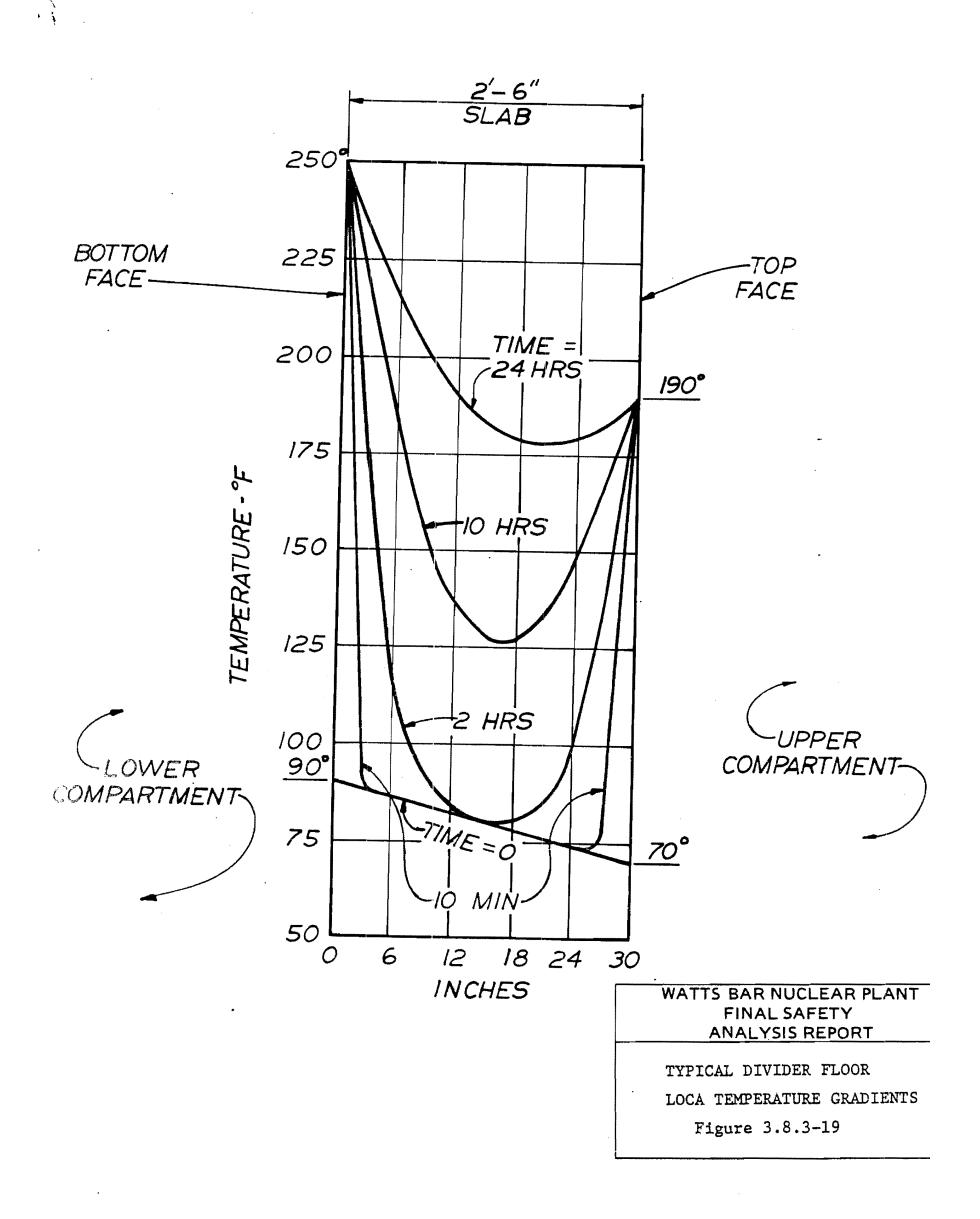
Figure 3.8.3-19 Typical Divider Floor LOCA Temperature Gradients
