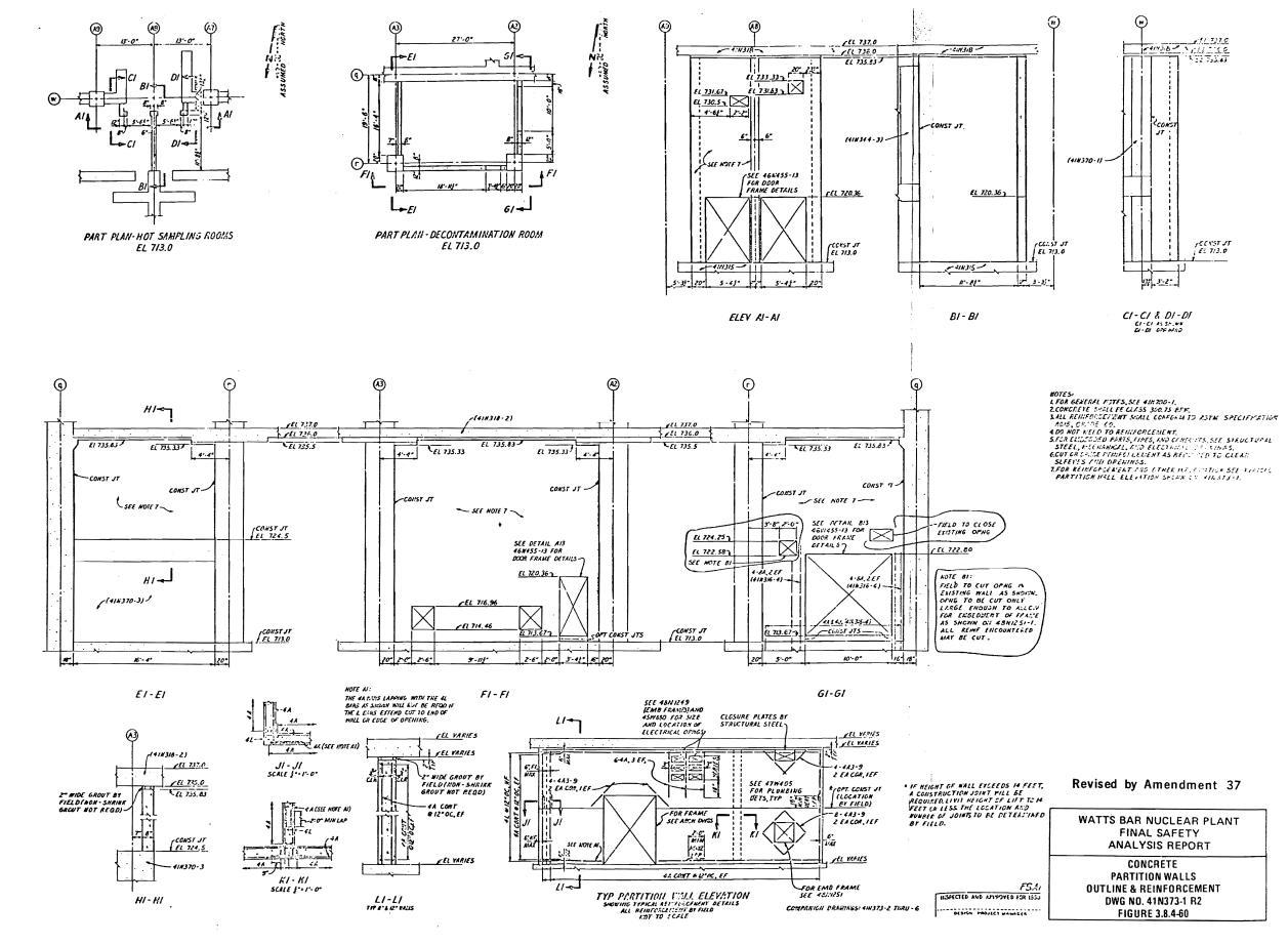
Figure 3.8.4-60 Concrete Partition Walls Outline and Reinforcement (Sheet 1)
