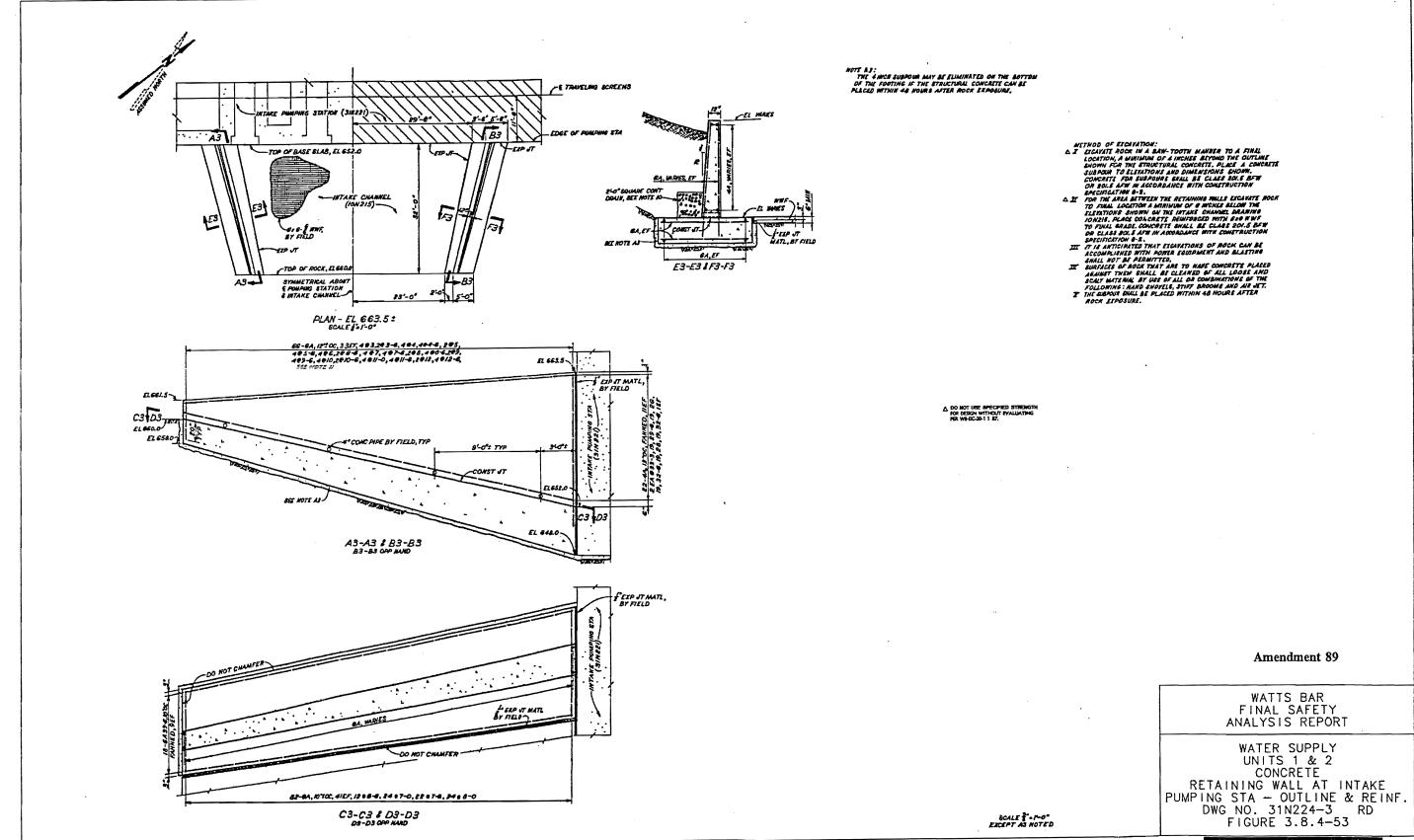
Figure 3.8.4-53 Water Supply Units 1 & 2 Concrete Retaining Wall at Intake Pumping Station - Outline and Reinforcement
