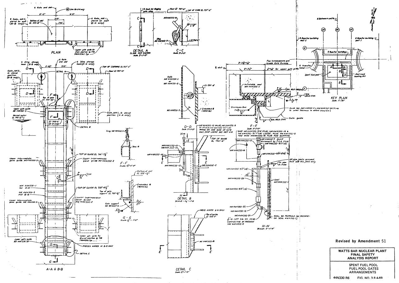
Figure 3.8.4-69 Spent Fuel Pool Fuel Pool Gates Arrangements
