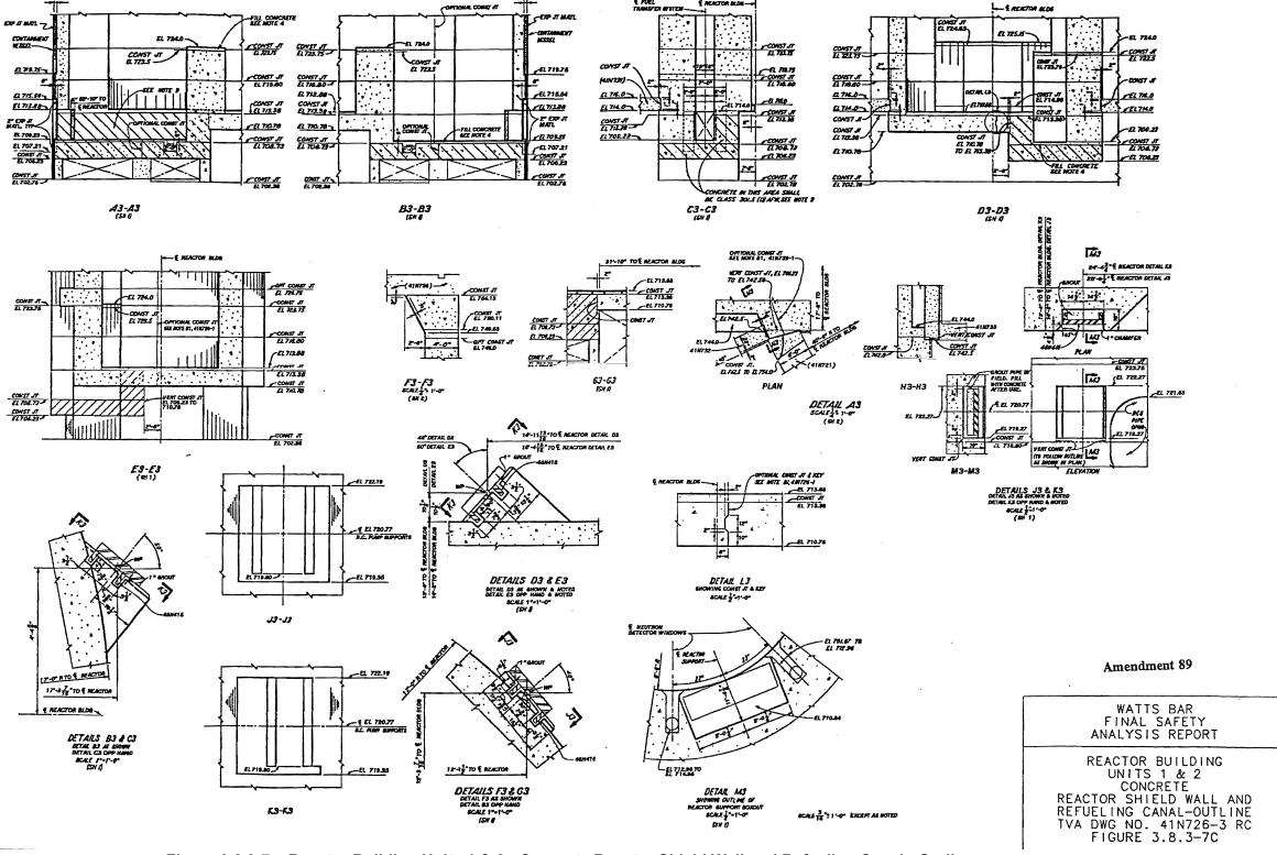
Figure 3.8.3-7c Reactor Building Units 1 & 2 - Concrete Reactor Shield Wall and Refueling Canal - Outline
