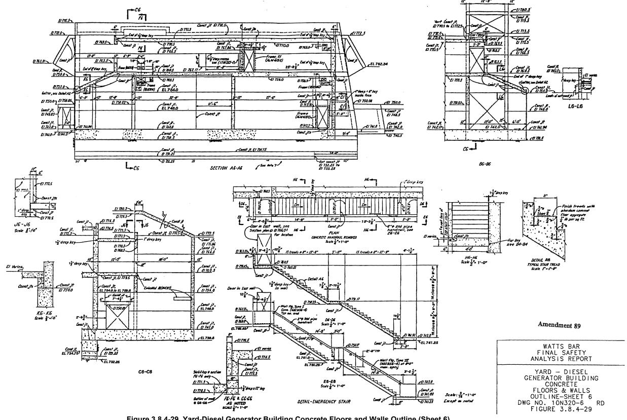
Figure 3.8.4-29 Yard-Diesel Generator Building Concrete Floors and Walls Outline (Sheet 6)
