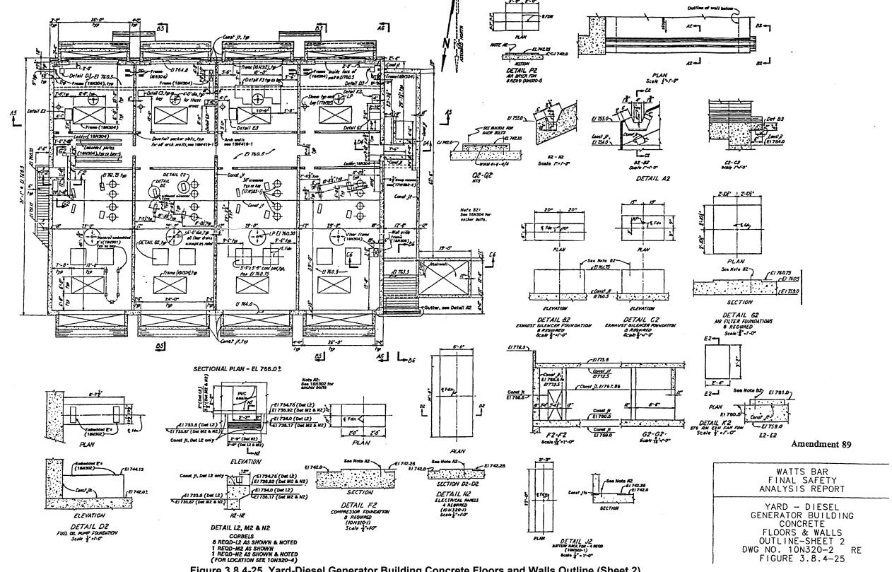
Figure 3.8.4-25 Yard-Diesel Generator Building Concrete Floors and Walls Outline (Sheet 2)
