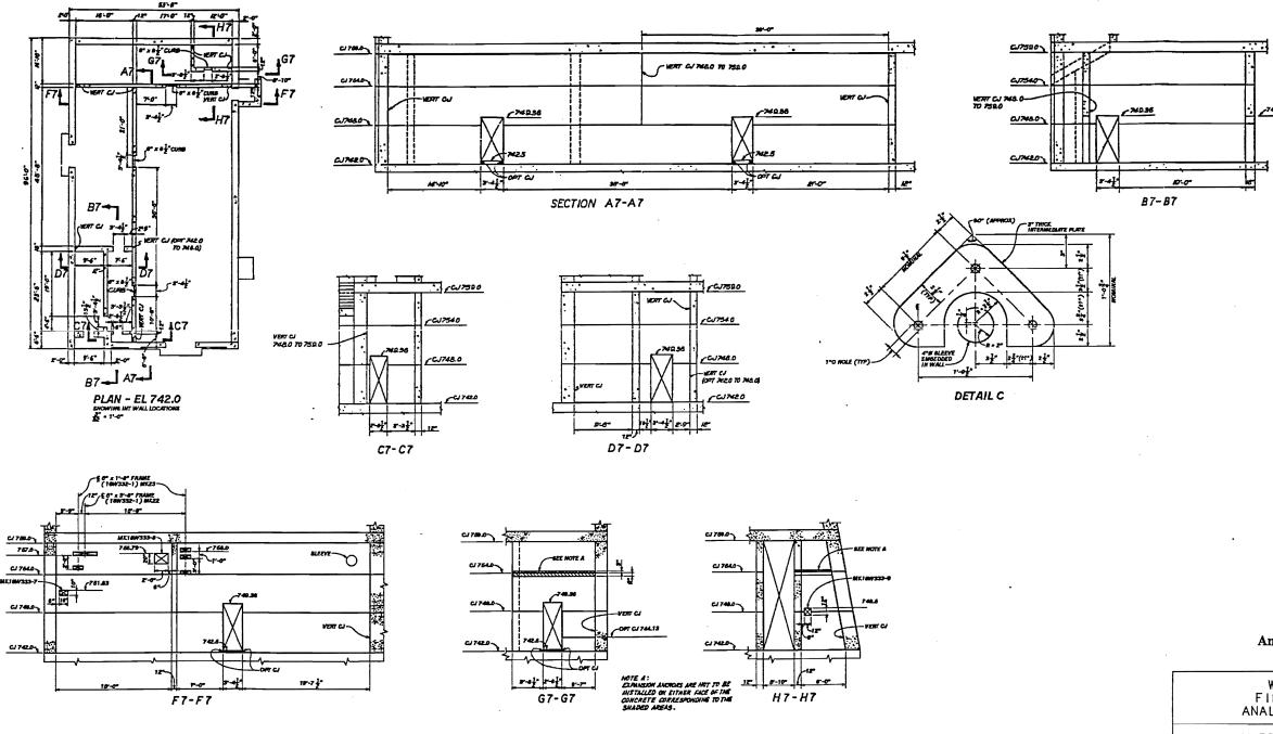
Figure 3.8.4-76 Yard Additional Diesel Generator Building Concrete Interior Walls EL. 742.0 Outline
