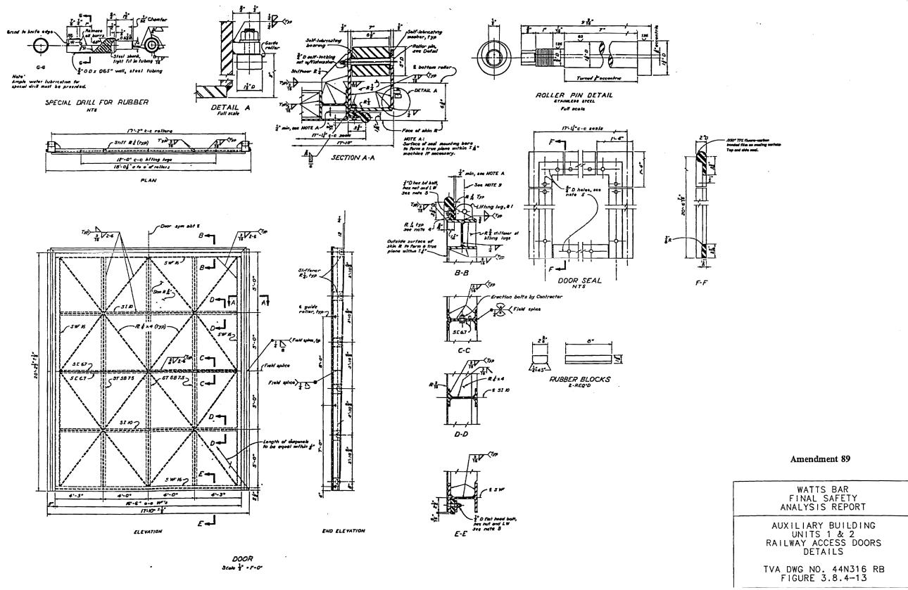
Figure 3.8.4-13 Auxiliary Buildings Units 1 & 2 Railway Access Doors Details
