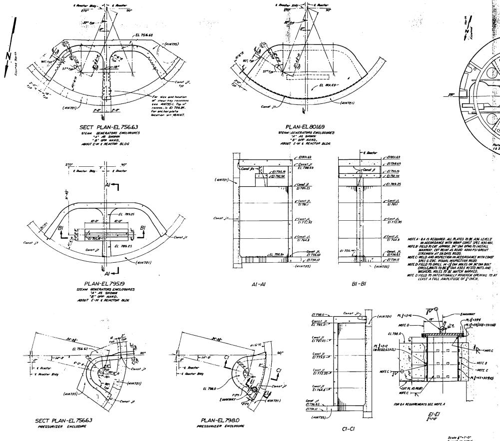
Figure 3.8.3-20 Reactor Building Units 1 & 2 - Concrete Steam Generator and Pressurizer Enclosure - Outline
