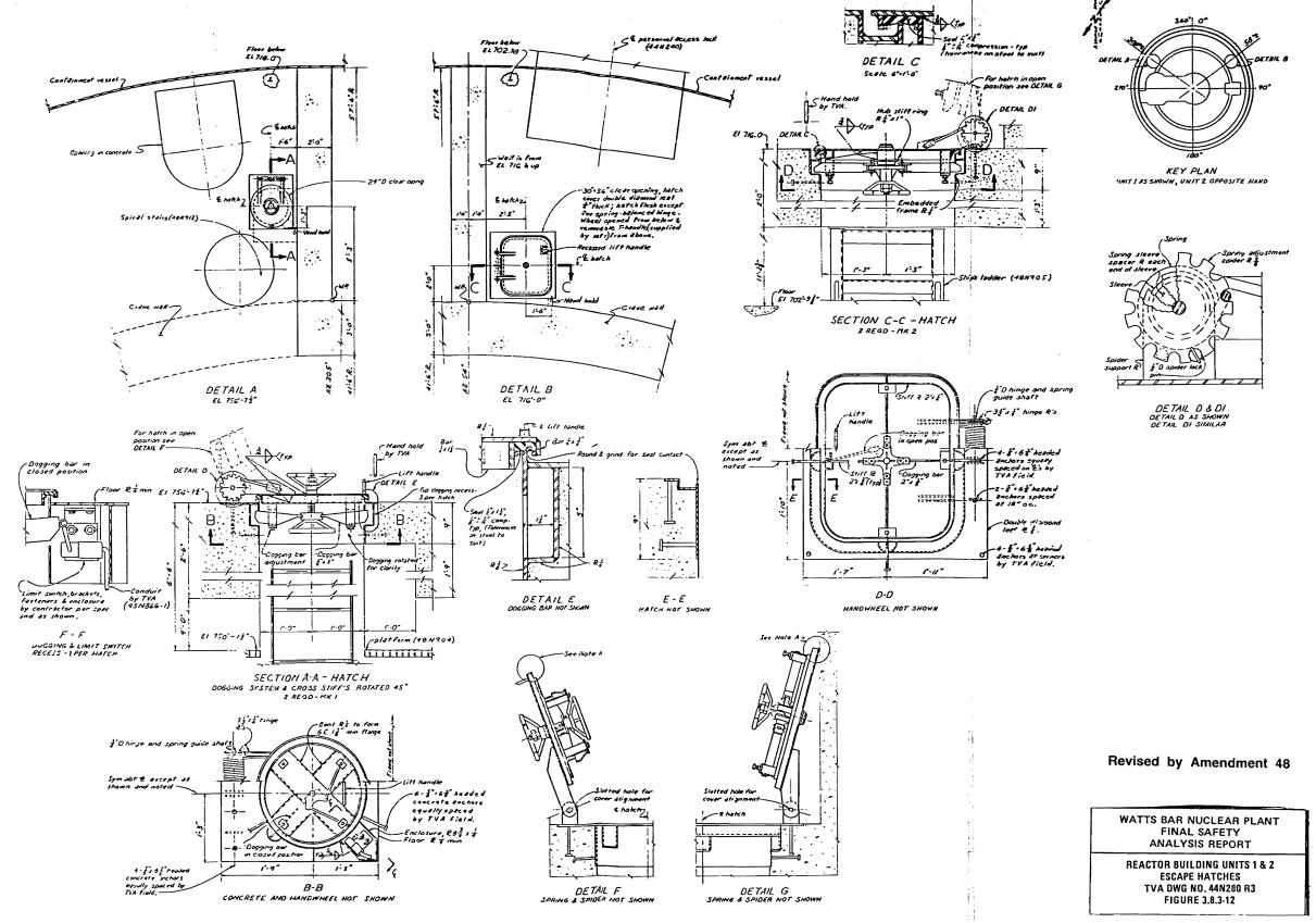
Figure 3.8.3-12 Reactor Building Units 1 & 2 - Escape Hatches
