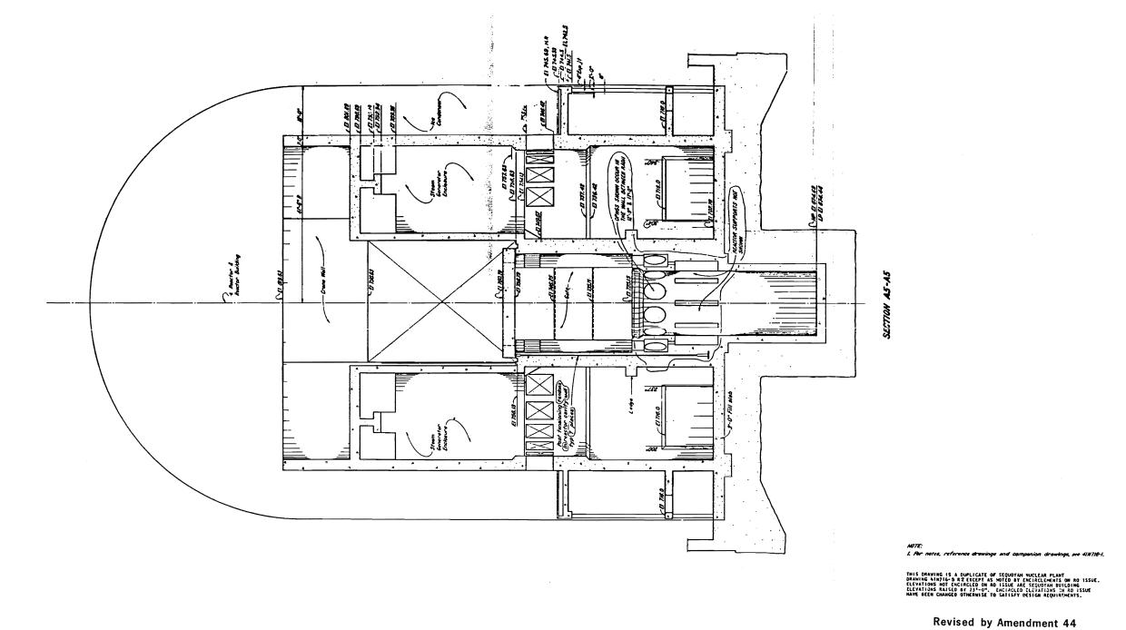
Figure 3.8.3-5 Reactor Building Units 1 & 2; Concrete Interior Structure Outline
