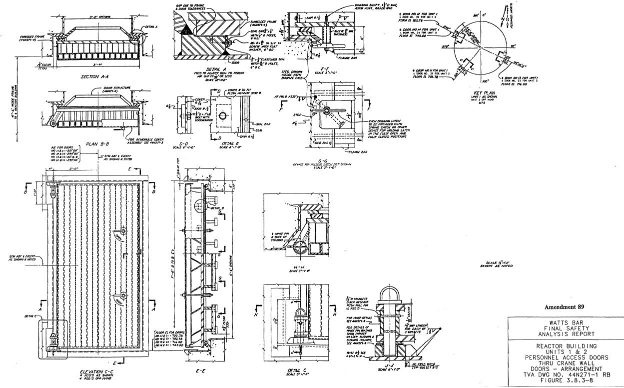
Figure 3.8.3-8 Reactor Building Units 1 & 2 - Personnel Access Doors Thru Crane Wall Doors -Arrangement
