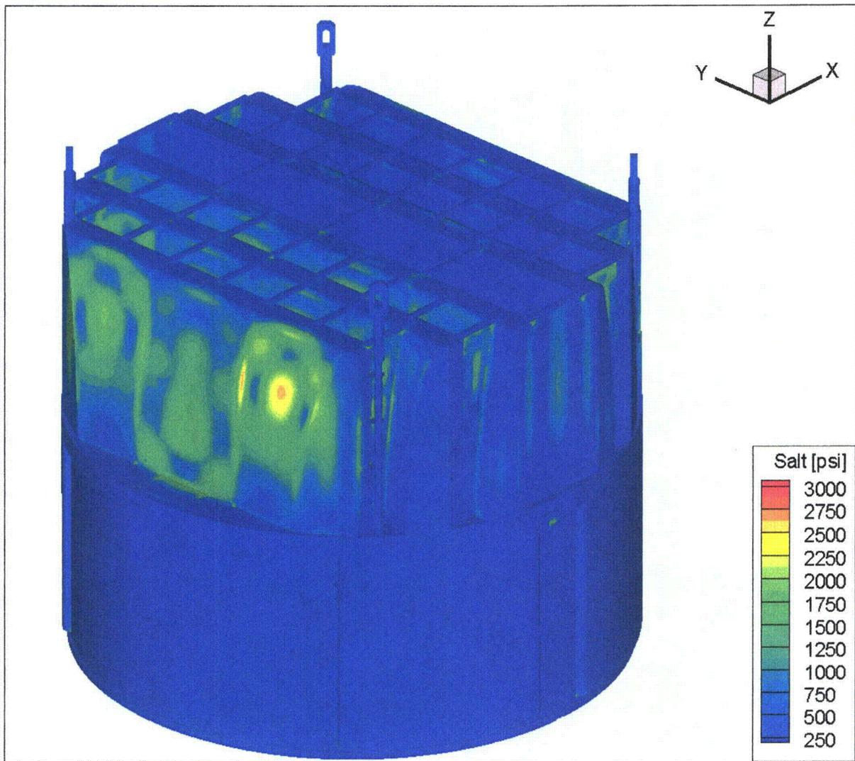
Figure 13d. Contour plot of alternating stress intensity,  $S_{alt}$ , for CLTP operation with frequency shifts. The recorded stress at a node is the maximum value taken over all frequency shifts. The maximum alternating stress intensity is 2914 psi. First view.
