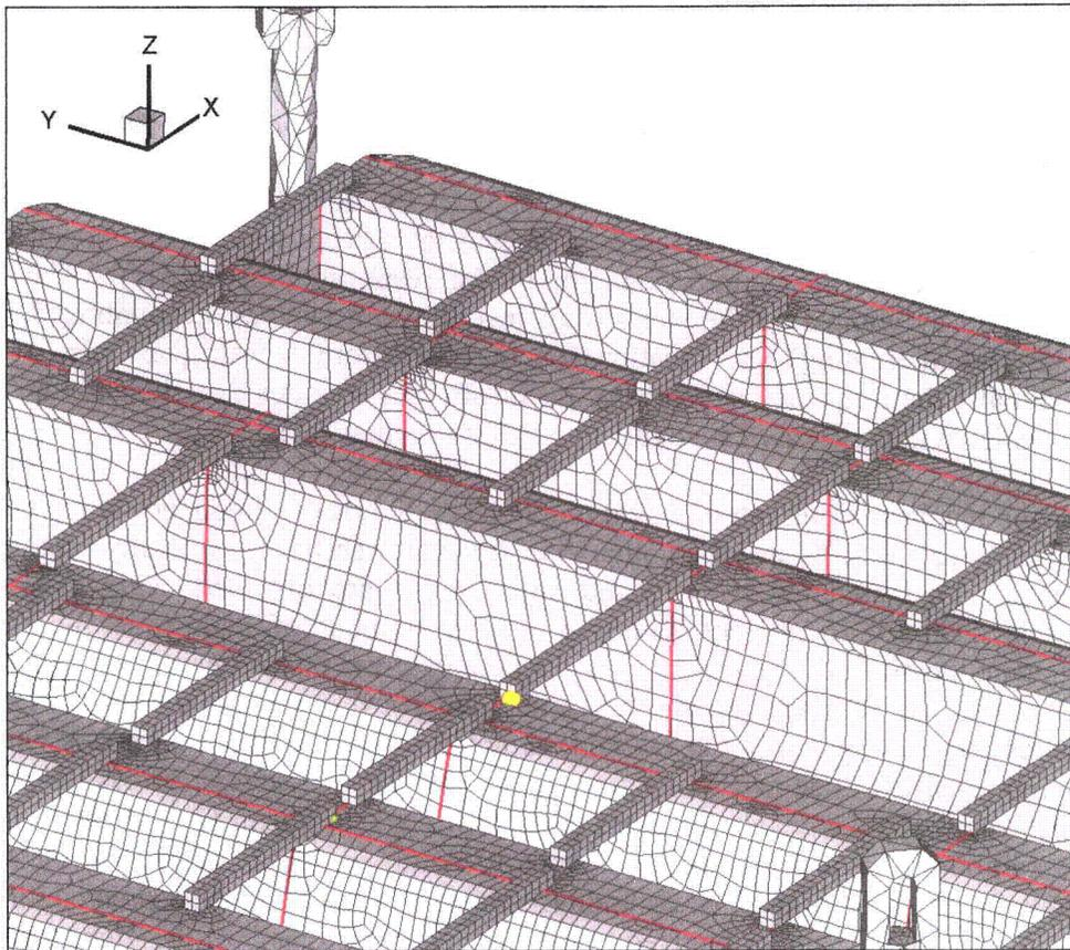
Figure 11f. Location of node on tie bar/top vane bank plate weld analyzed with sub-model analysis procedure in [29]. Sub-model corresponds to location 9 in Table 7.
