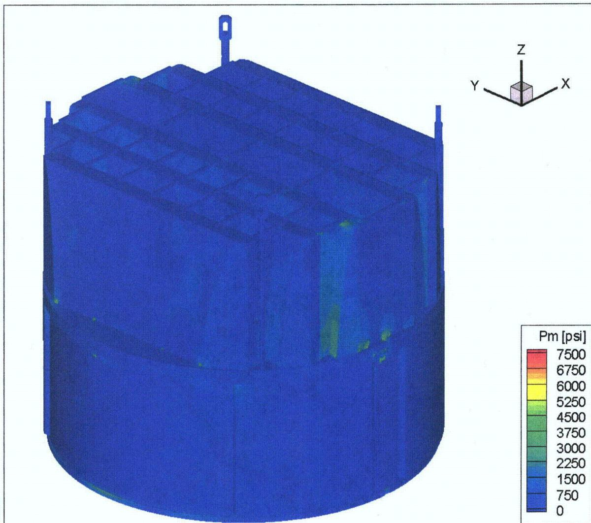
Figure 13a. Contour plot of maximum membrane stress intensity,  $P_m$ , for CLTP operation with frequency shifts. The recorded stress at a node is the maximum value taken over all frequency shifts. The maximum stress intensity is 7490 psi.
