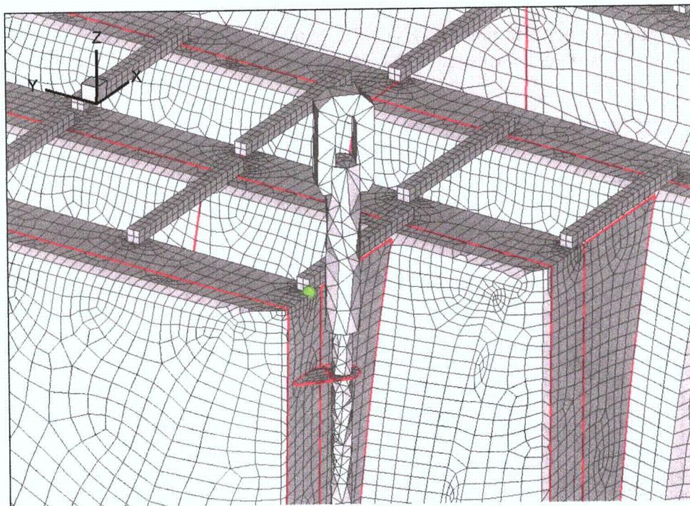
Figure 11e. Location of node on side plate/top plate weld analyzed with sub-model analysis procedure in [29]. Sub-model corresponds to location 8 in Table 7.
