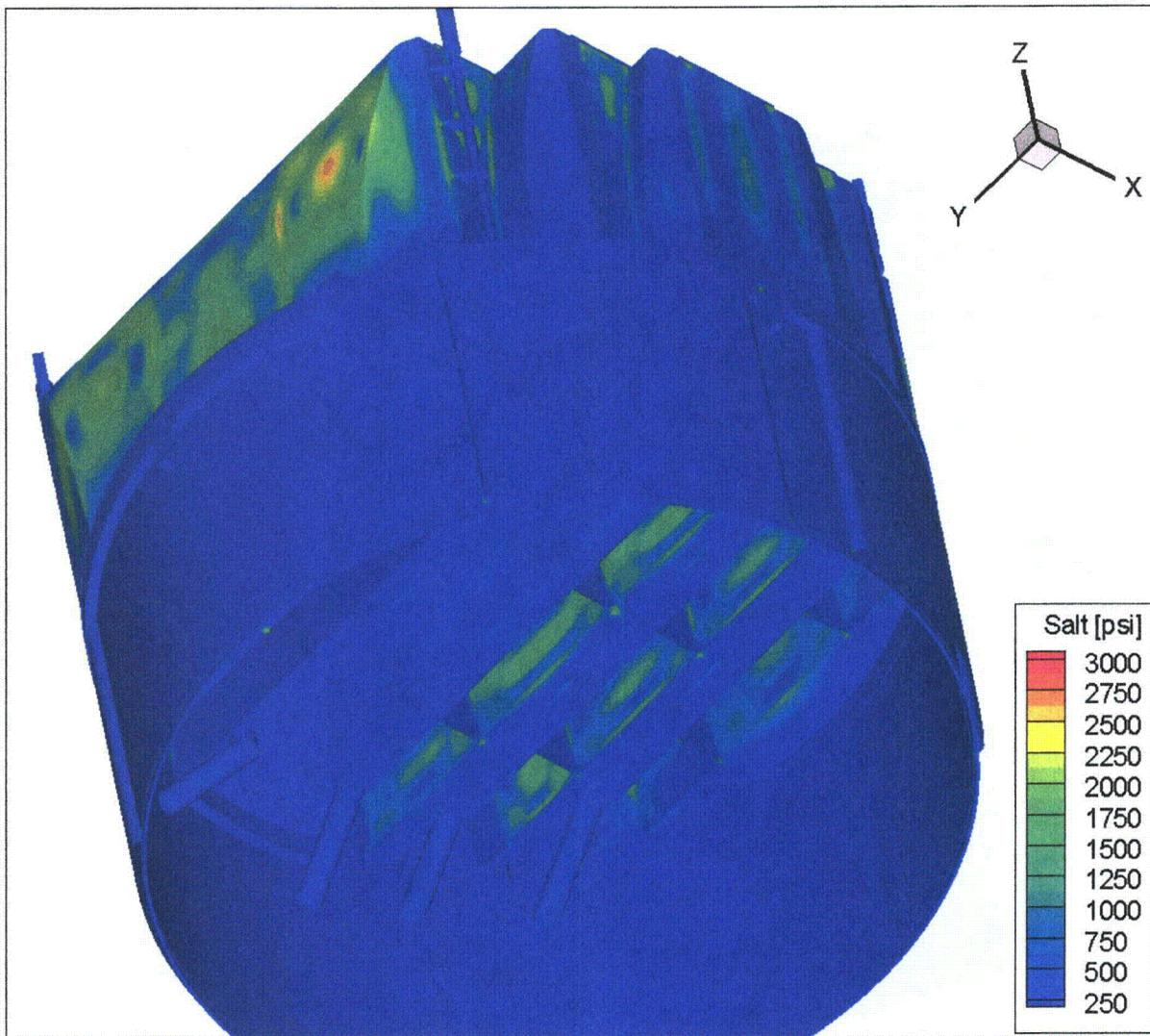
Figure 13e. Contour plot of alternating stress intensity,  $S_{alt}$ , for CLTP operation with frequency shifts. The recorded stress at a node is the maximum value taken over all frequency shifts. Second view from below.
