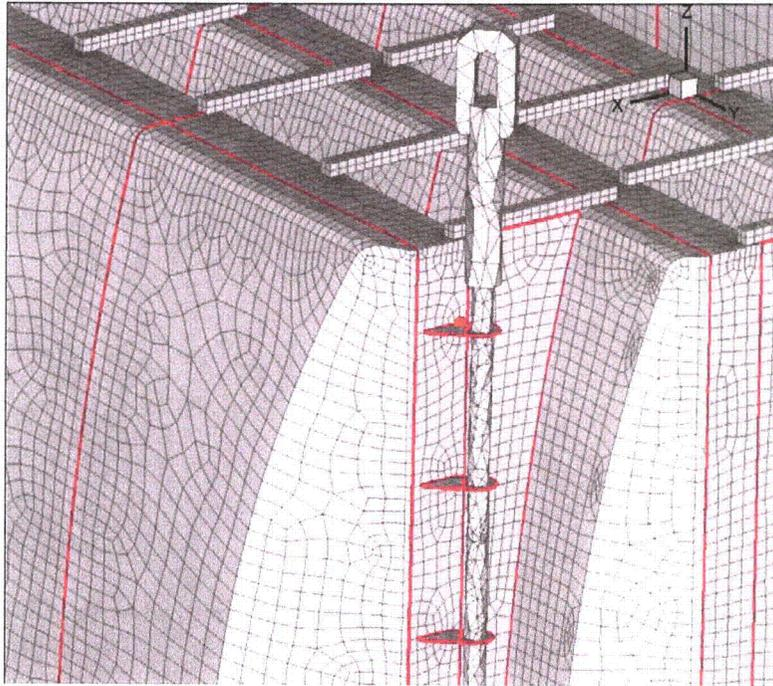
Figure 11b. Location of node on inner hood/hood support/middle base plate weld analyzed with sub-model in [29]. Sub-model corresponds to location 5 in Table 7.
