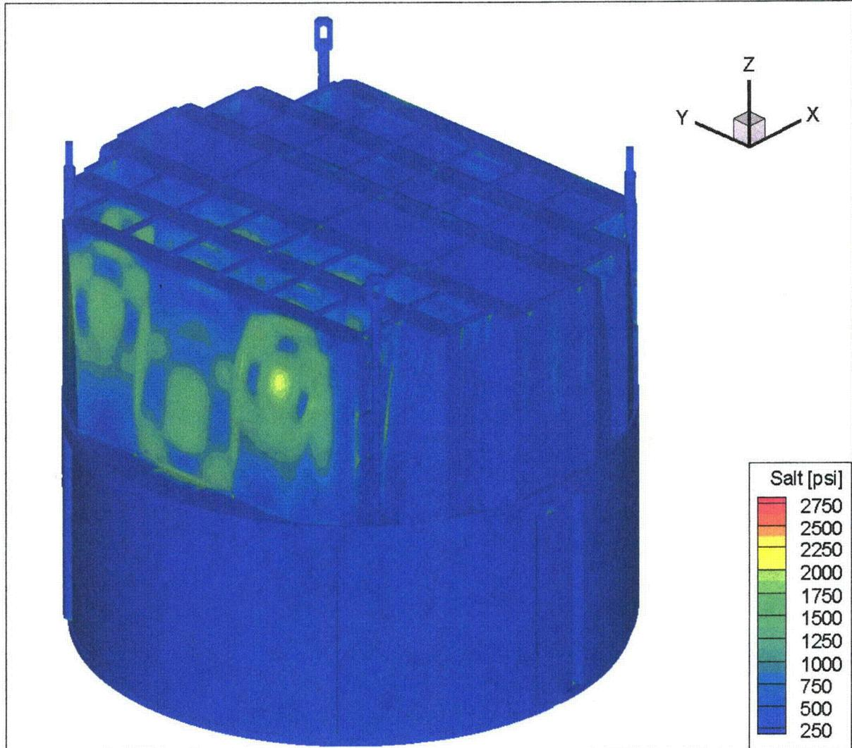
Figure 12d. Contour plot of alternating stress intensity,  $S_{alt}$ , for CLTP load. The maximum alternating stress intensity is 2728 psi. First view.
