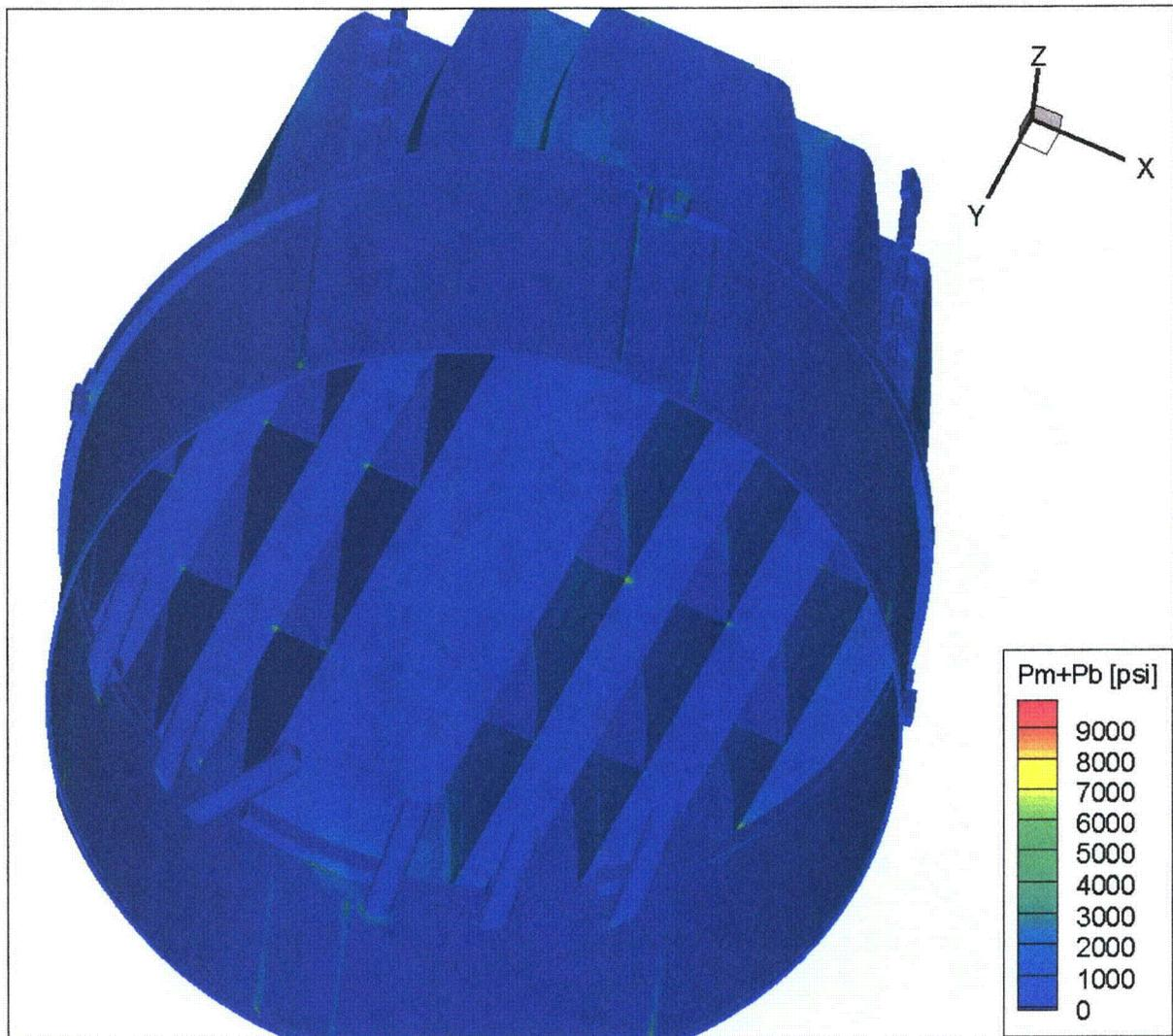
Figure 13c. Contour plot of maximum membrane+bending stress intensity,  $P_m+P_b$ , for CLTP operation with frequency shifts. This second view from beneath reveals stresses on the hood support/base plate junctions, outer cover plate and drain channel/skirt welds.
