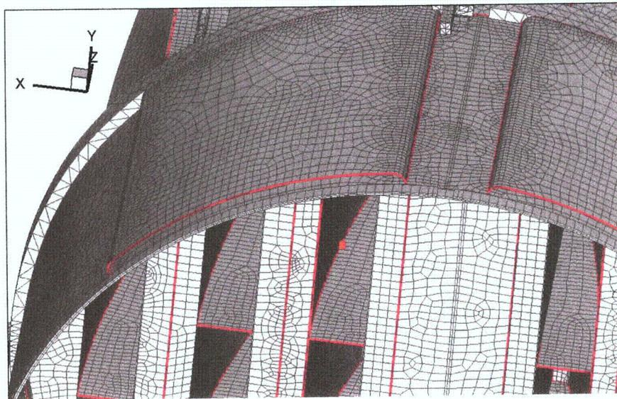
Figure 11d. Location of node on hood/hood support weld analyzed with sub-model analysis procedure in [26]. Sub-model corresponds to location 7 in Table 7.
