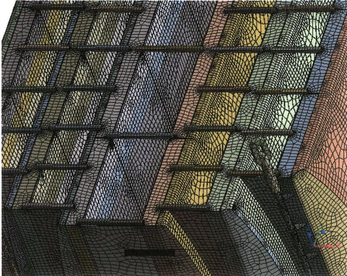
Figure 5f. Close up view of tie bars.
