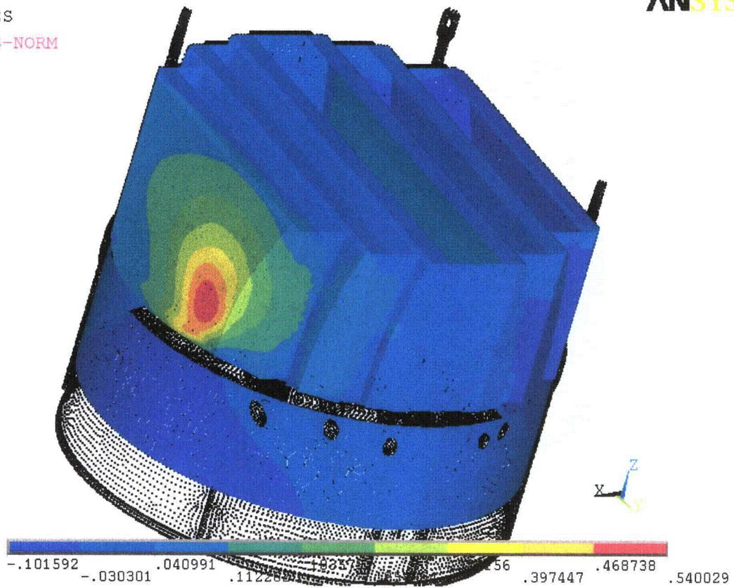
Figure 8a. Real part of unit pressure loading MSL A (in psid) on the steam dryer at 50.1 Hz. No loading is applied to the submerged surface and lifting rods.
