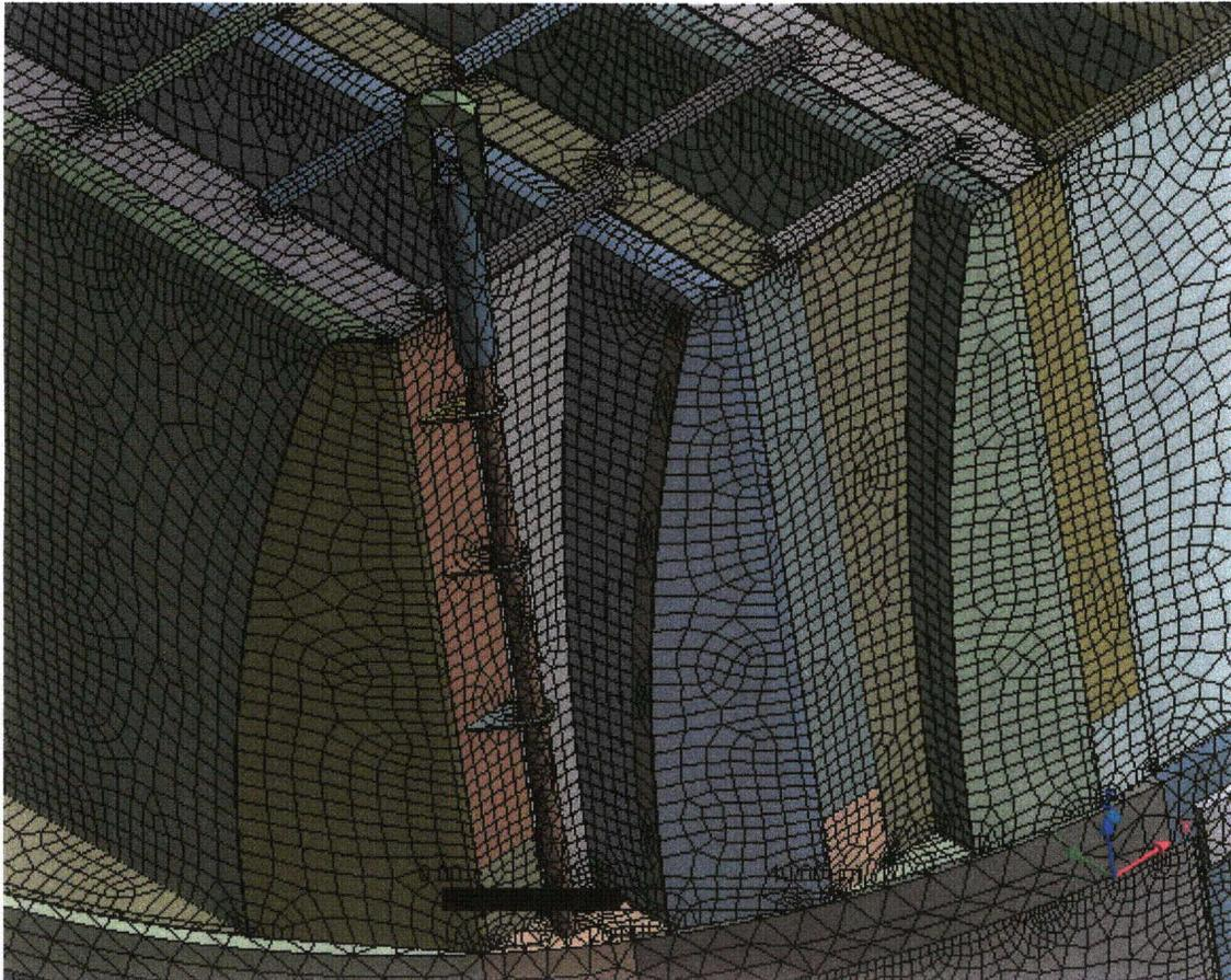
Figure 5b. Close up of mesh showing on-site modifications.
