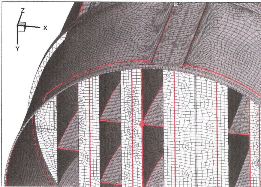
Figure 11c. Location of node on hood/hood support/base plate weld analyzed with sub-model in [25]. Sub-model corresponds to location 6 in Table 7.
