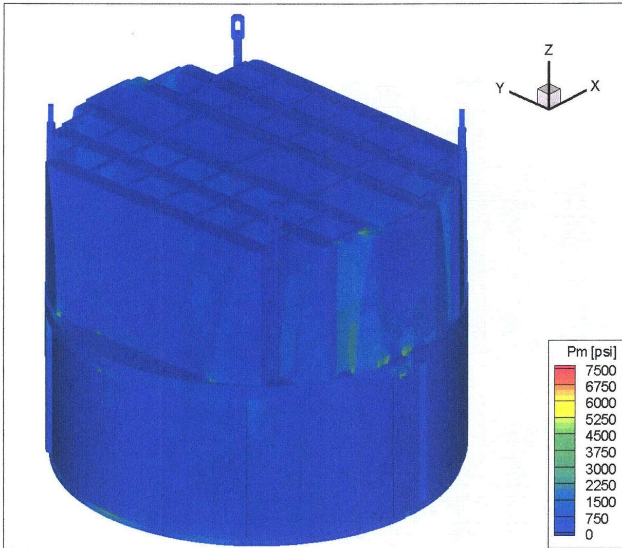
Figure 12a. Contour plot of maximum membrane stress intensity,  $P_m$ , for CLTP load. The maximum stress intensity is 7475 psi.
