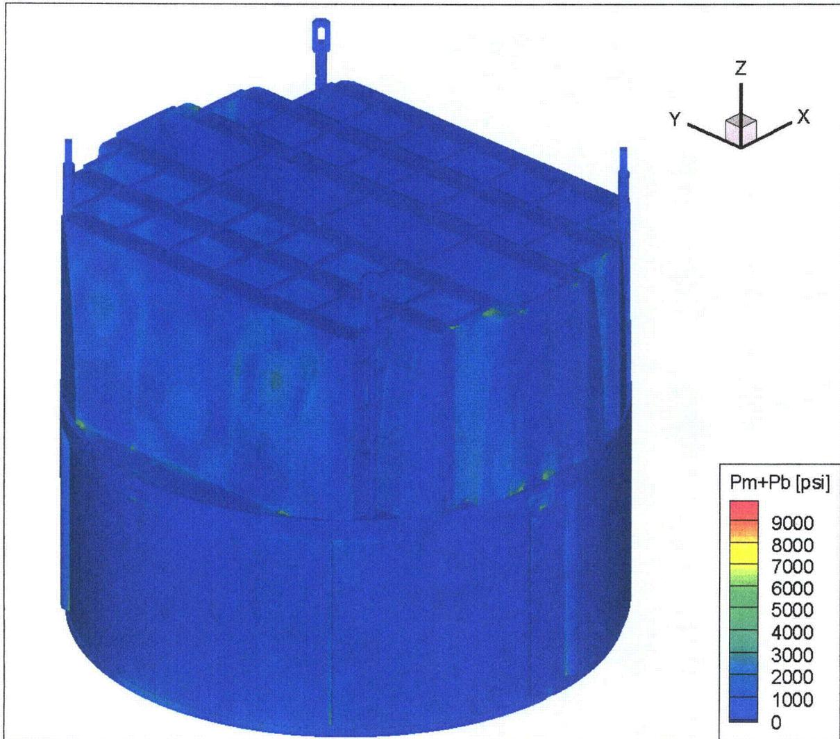
Figure 13b. Contour plot of maximum membrane+bending stress intensity,  $P_m+P_b$ , for CLTP operation with frequency shifts. The recorded stress at a node is the maximum value taken over all frequency shifts. The maximum stress intensity is 9809 psi. First view.
