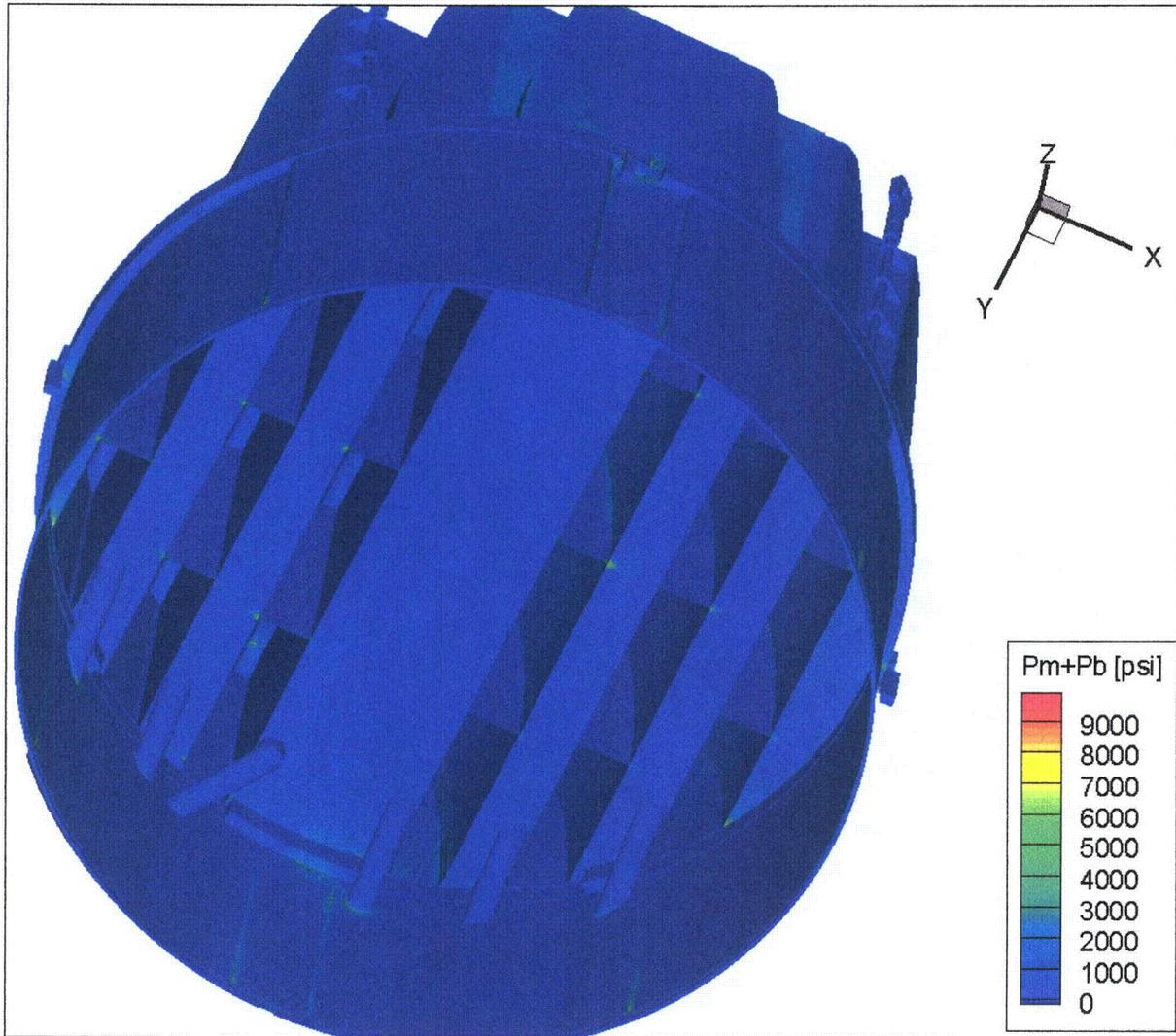
Figure 12c. Contour plot of maximum membrane+bending stress intensity,  $P_m+P_b$ , for CLTP load. This second view from below shows the high stress intensities at the hood/stiffener/base plate junctions and drain channel/skirt welds.
