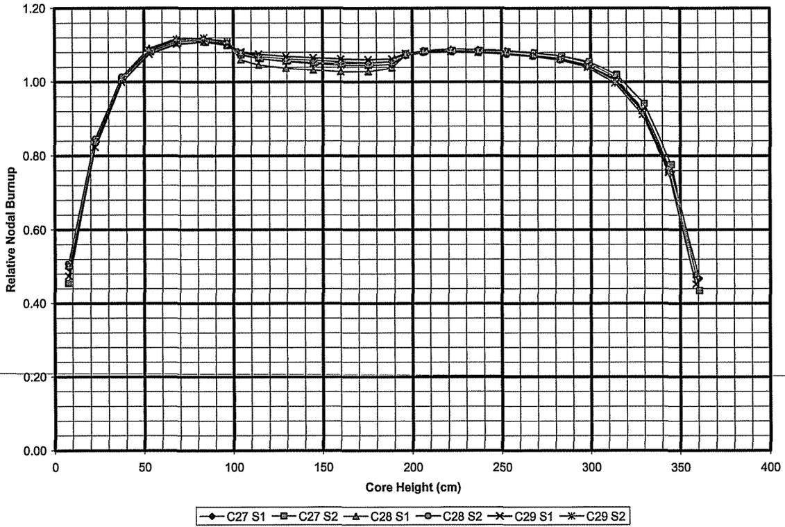
**Figure 1 - Axial Burnup Profiles for Fuel Assemblies Containing PPSAs**
