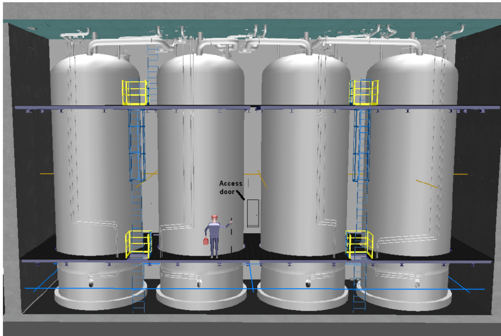
Figure 12.03-12.04-9 (Part 2) —Coolant Storage Compartment Facing North - Exterior Wall Removed
