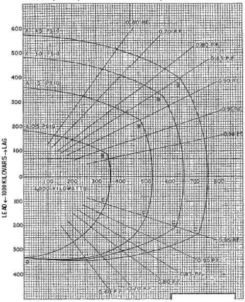
CURVE AS LIMITED BY FIELD HEATING CURVE BC LIMITED BY ARMATURE HEATING CURVE CO LIMITED BY ARMATURE CORE END HEATING
