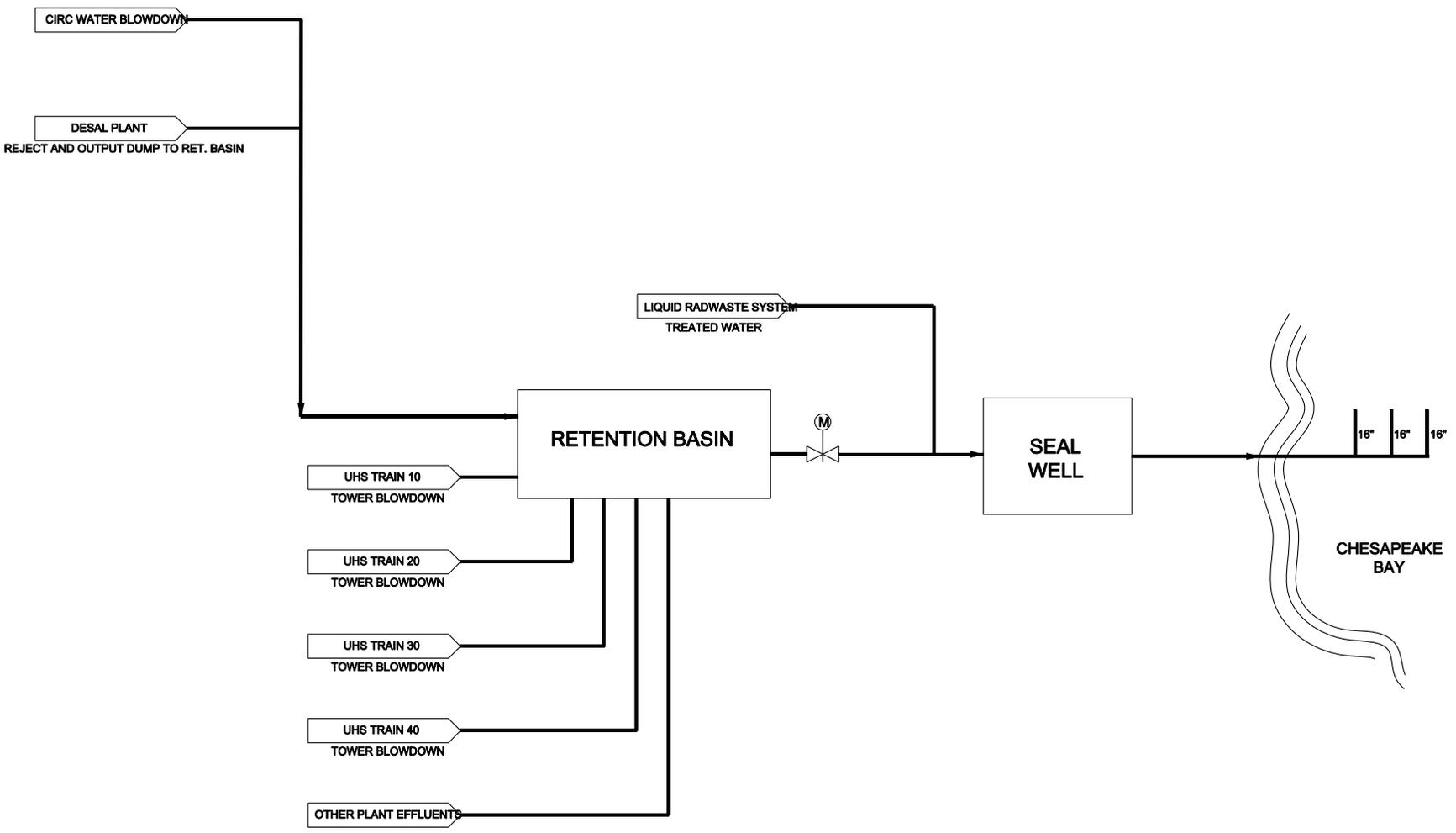
Figure 10.4-7—{Circulating Water System Plant Discharge}
