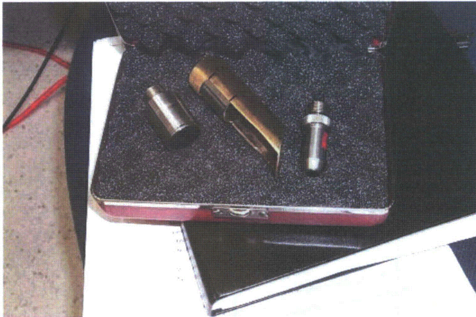
Figure 3.11 Two Immersion Ultrasonic Transducers with Mirror Assembly in Center. The mirror provided a 0-degree incident angle for the inspection.
