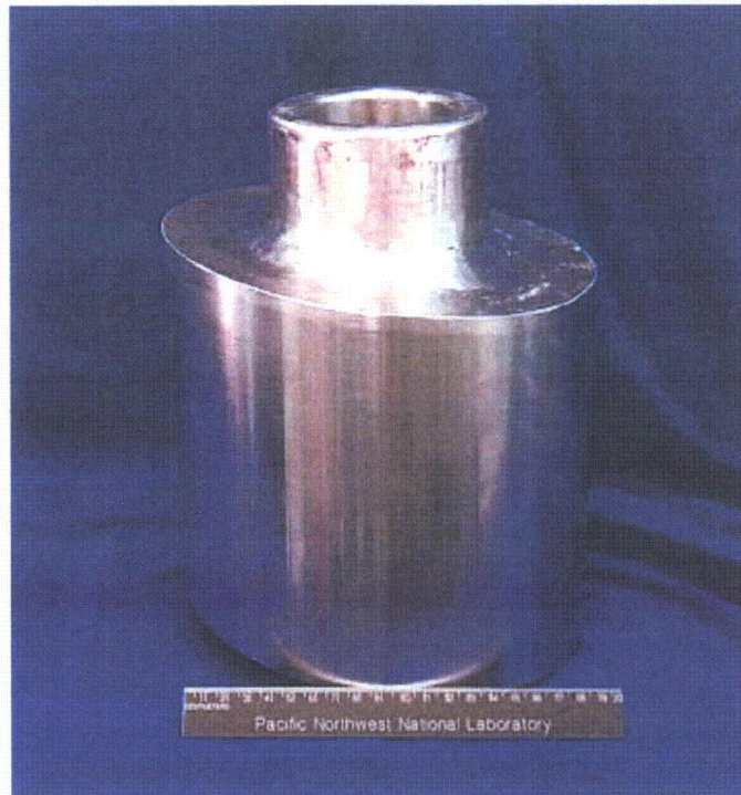
Figure 4.2 Midland Control Rod Drive Mechanism Used for Testing Immersion UT Equipment and Techniques
