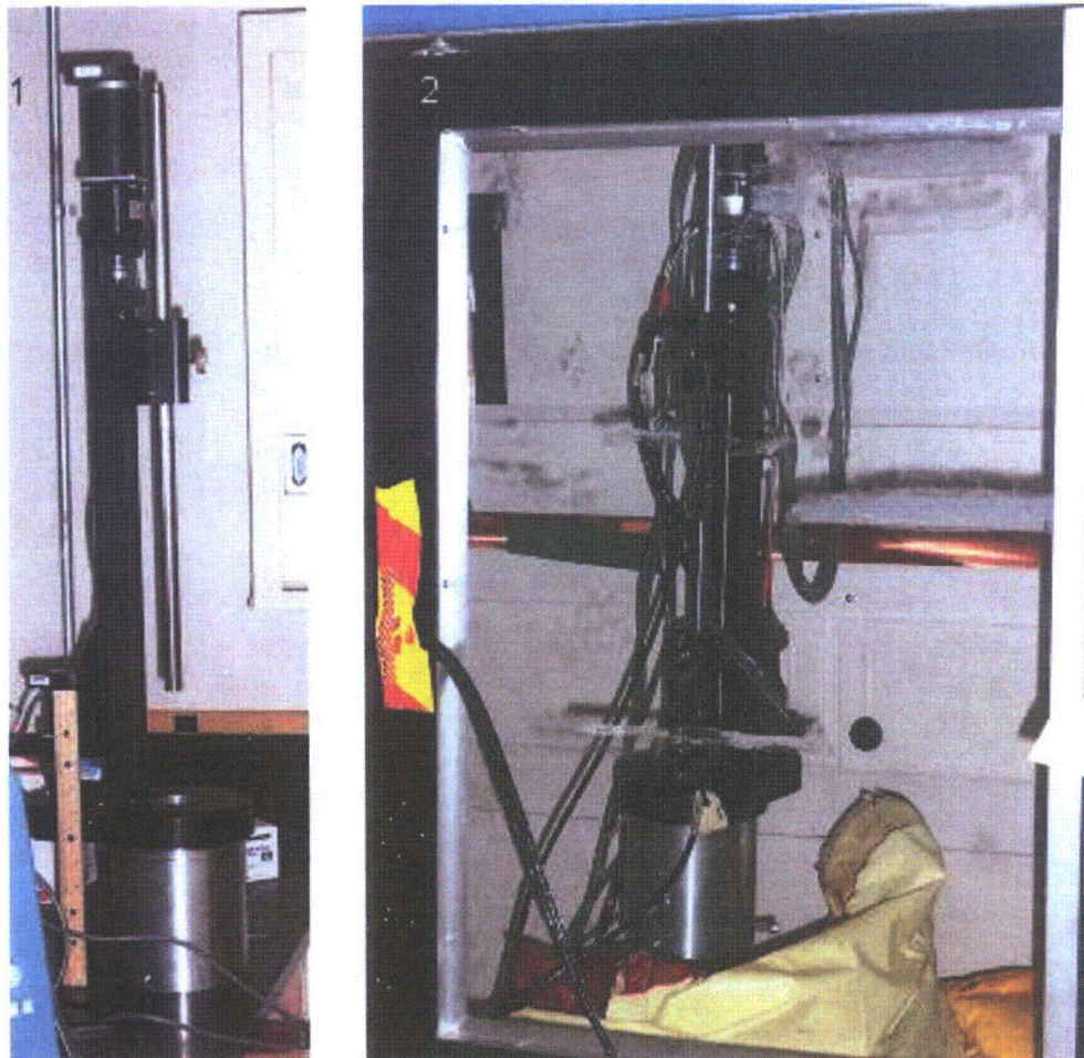
Figure 3.1 CRDM Scanner on Laboratory Bench with 30-cm Scale (left) and in Use on CRDM Nozzle 31 in PNNL Walk-In Hood (right)
