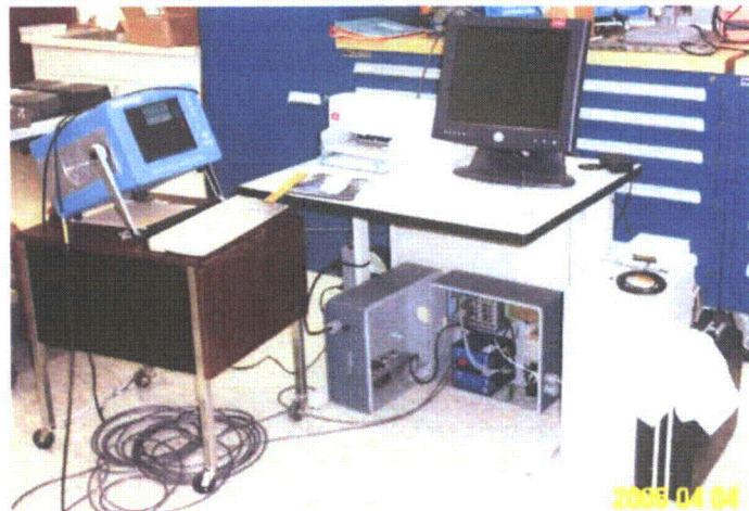
Figure 3.4 Data Collection Apparatus: Zetec Eddy Current Instrument (left), Computer (lower right), and Control Electronics (bottom center)
