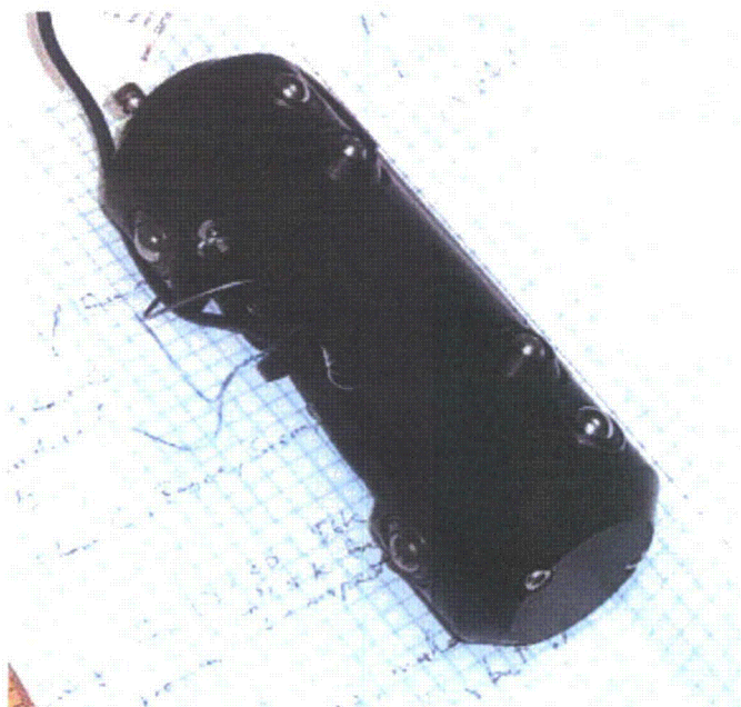
Figure 3.5 Redesigned Probe Assembly Showing Roller Bearings and Both Sensors
