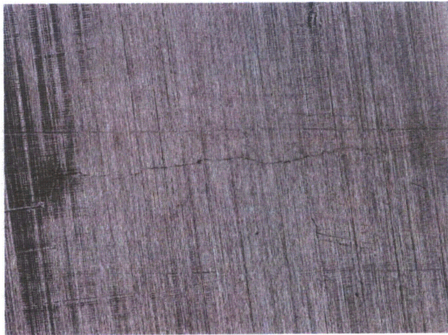
Figure 4.14 A Crack 28 \mu\text{m} (0.001 in.) Wide Cutting Perpendicularly Across Machining Marks
