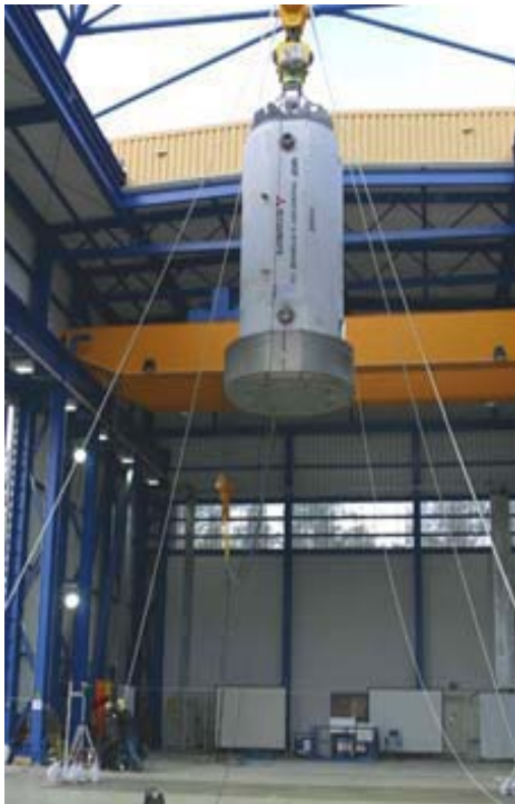
9-Meter Vertical Drop Cask
