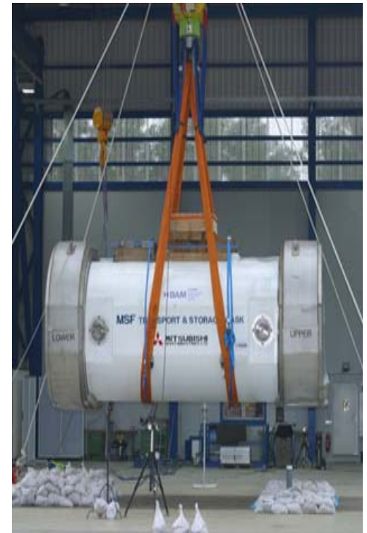
1-Meter Horizontal Drop - Cask
