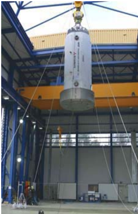
9-Meter Vertical Drop Cask
