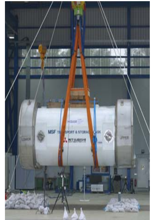
1-Meter Horizontal Drop - Cask
