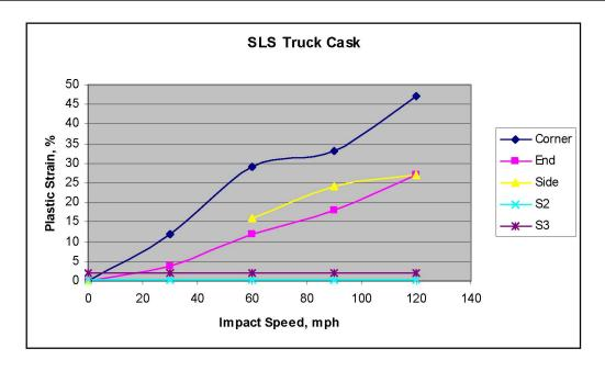
NOTE: <sup>1</sup> Data points for strain versus speeds greater than 30 mph taken directly from NUREG/CR-6672 (Ref. D4.1.65, Table 5.3): plots extended to origin (0,0) to determine crossover for S2 and S3 threshold strains. <sup>2</sup> S2 and S3 threshold strains based on information in *A Railroad Industry Critique of the Model Study* (Ref. D4.1.30).
