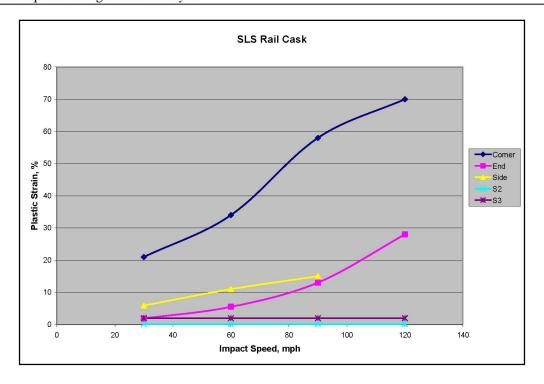
NOTE: <sup>1</sup> Data points for strain versus speeds greater than 30 mph taken directly from NUREG/CR-6672 (Ref. D4.1.65, Table 5.3): plots extended to origin (0,0) to determine crossover for S2 and S3 threshold strains. <sup>2</sup> S2 and S3 threshold strains based on information in *A Railroad Industry Critique of the Model Study* (Ref. D4.1.30).
