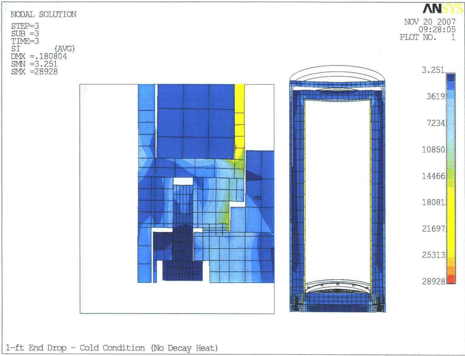
Figure 33 Stress Intensity Plot – 1-ft End Drop – Load Combination No.3
