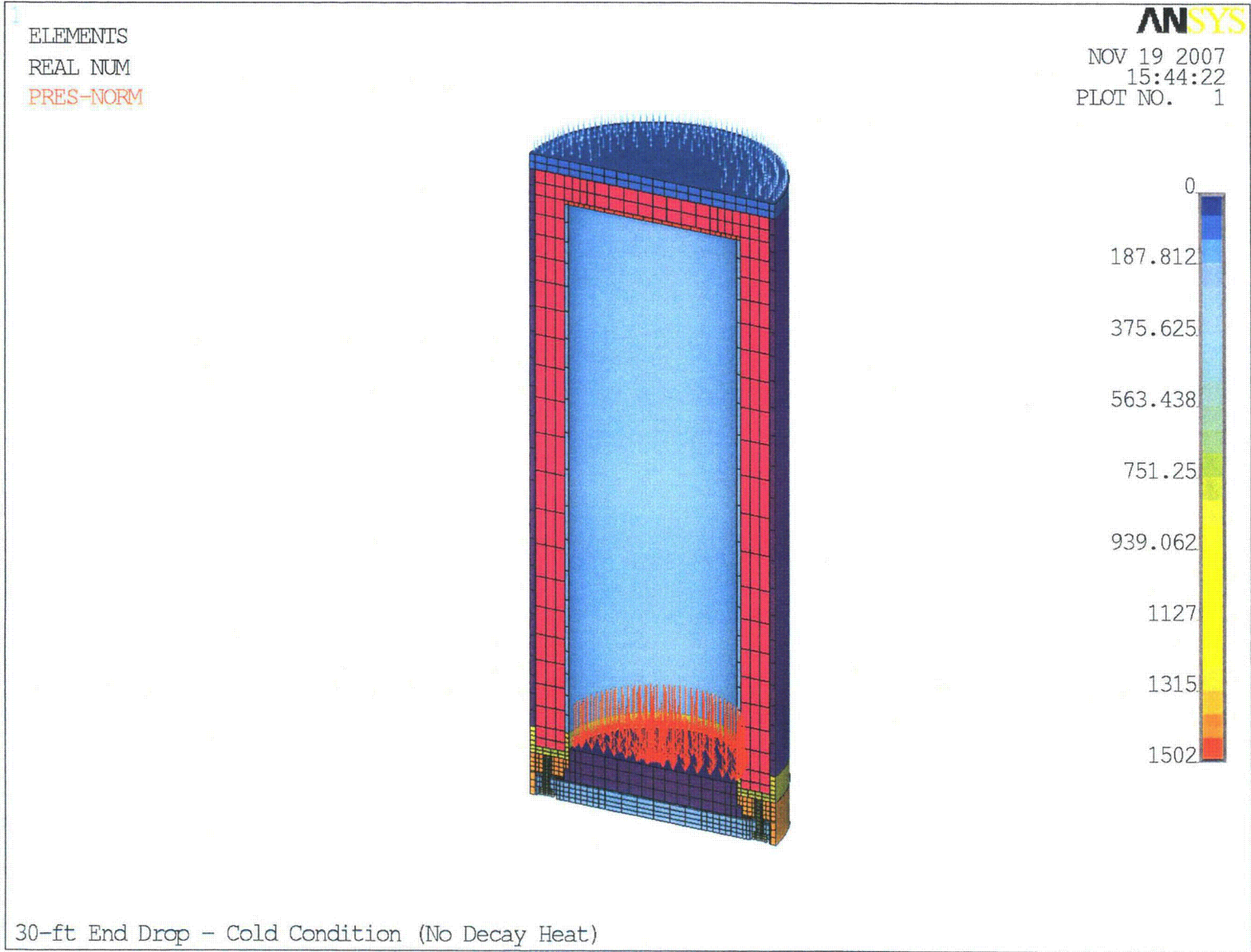
Figure 9 Temperature Profile and Pressure Distribution Used for 30-ft End Drop – Load Combination No.3
