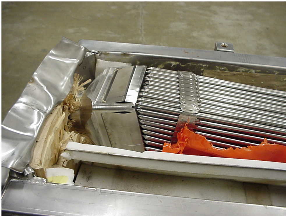
Figure 2-41 Fuel Damage CTU 2
