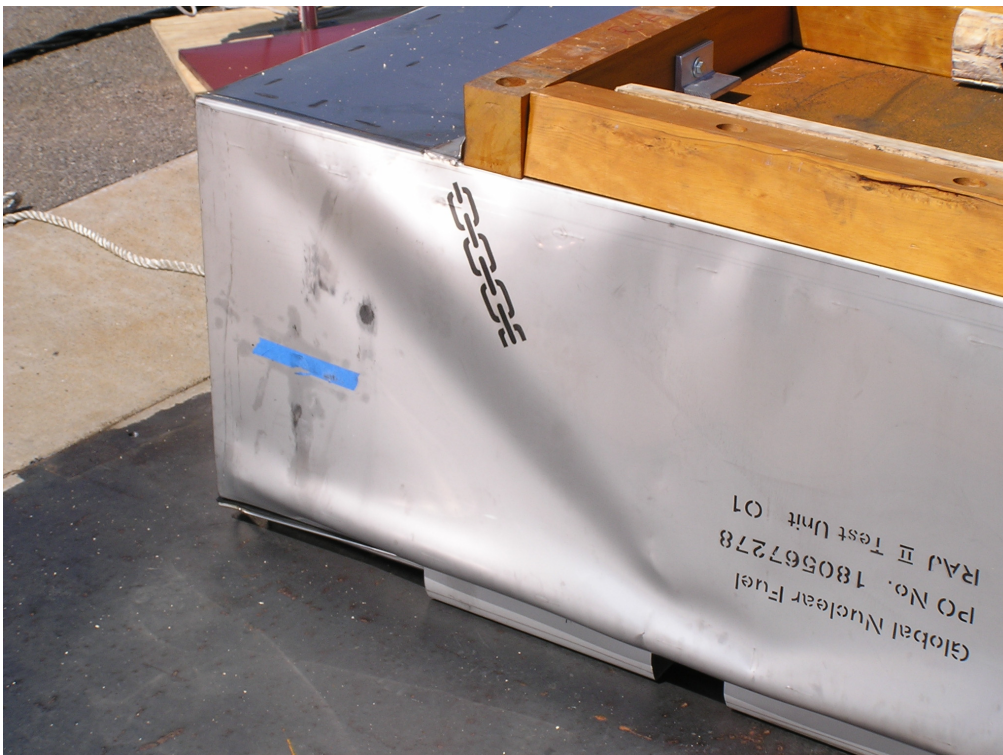
Figure 2-30 Secondary Impact End Damage
