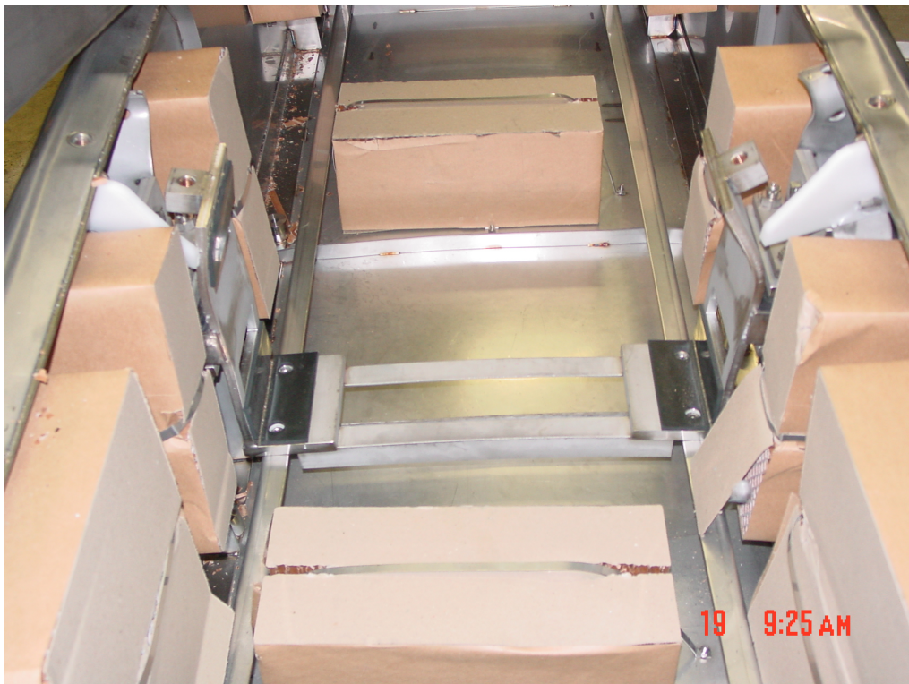
Figure 2-37 Internal Damage to Outer Container CTU 1
