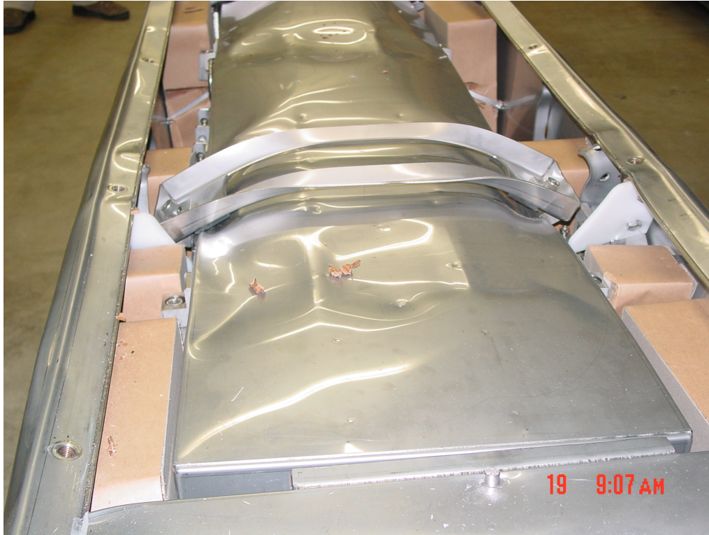
Figure 2-36 Damage Inside Outer Container to CTU 1
