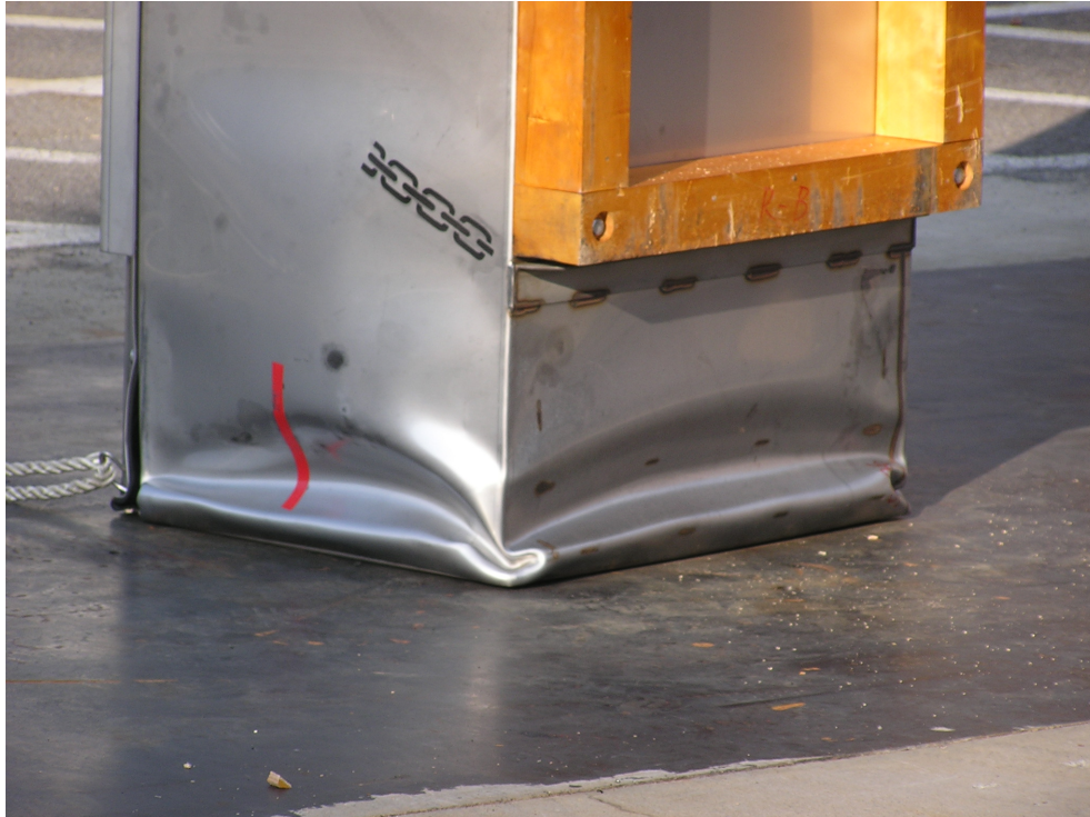
Figure 2-34 Damage from End Impact (Bottom and Side)
