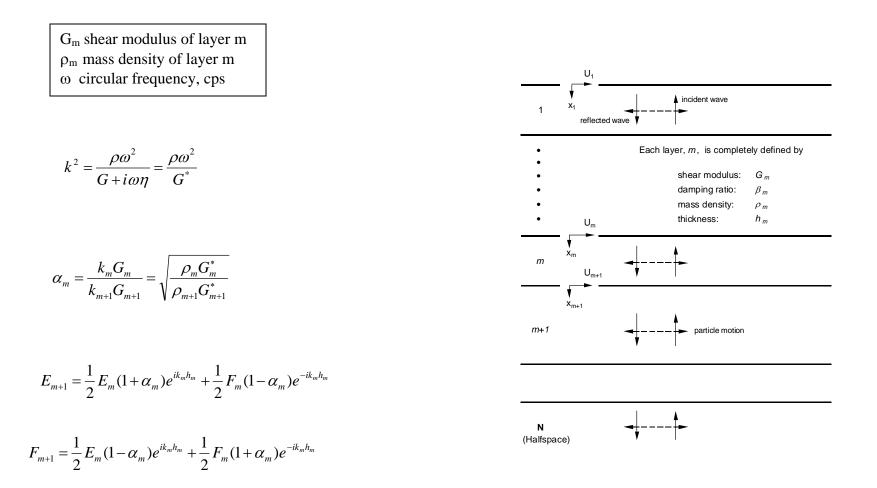
Figure 2-1 One-Dimensional Wave Propagation in Layered System
