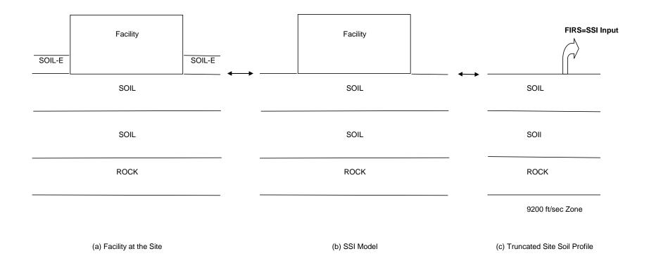
Figure 3-5 Development of FIRS and SSI Input Motion for Analysis of Structures with Shallow Embedment Modeled as Surface Structures
