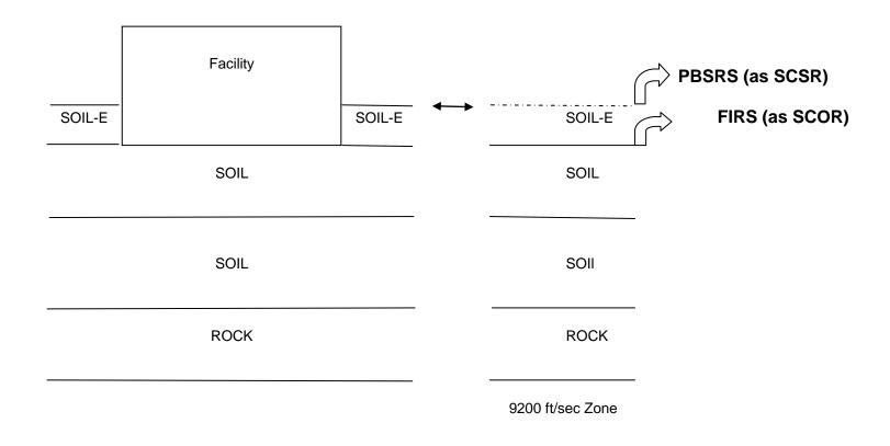
(a) Facility at the Site-SSI Model (b) Site Soil Profile Figure 3-6 Development of FIRS and SSI Input Motion for Analysis of Structures with Embedment
