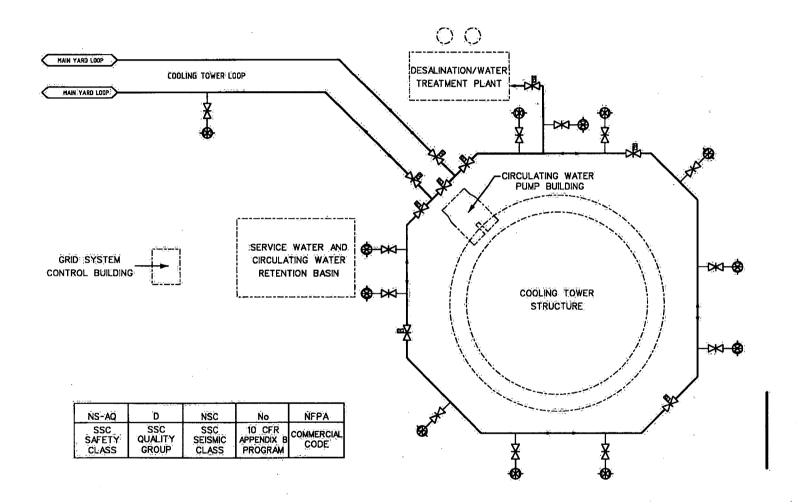
Figure 9.5-2-{CCNPP Unit 3 Fire Water Distribution System - Cooling Tower Loop}
