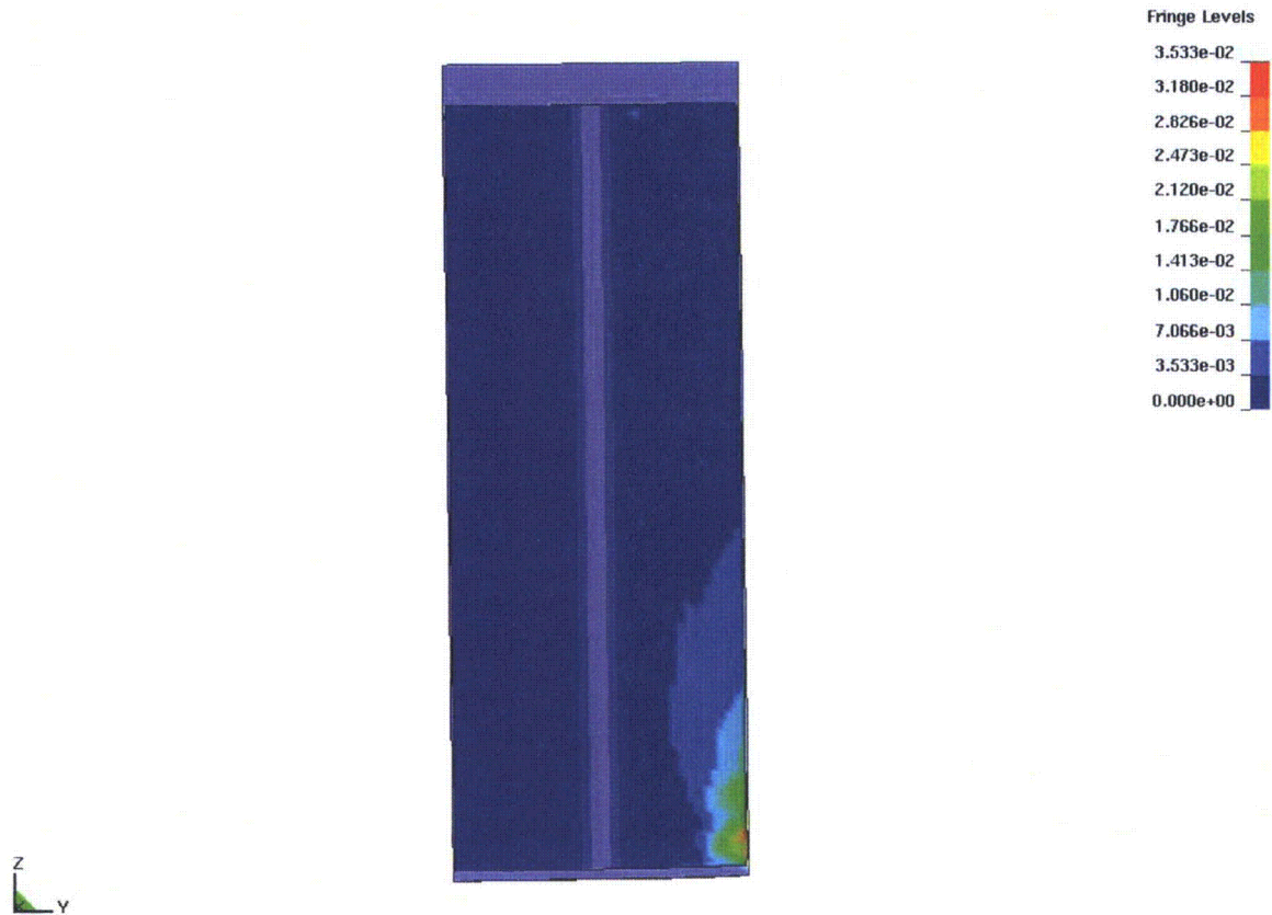
Figure 6.3.2.1-1. Max EPS for SNF Canister inside a Transportation Cask Subjected to 12-ft Drop with 4-degree Off-Vertical Orientation
