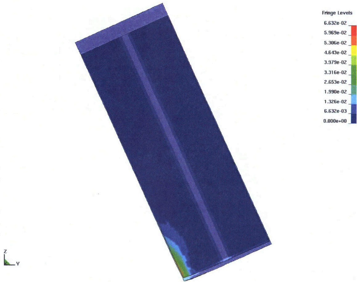
Figure 6.3.2.5-5. Max EPS for SNF Canister inside a Transportation Cask Subjected to a 30-ft End Drop with the Center of Gravity over the Corner of Cask
