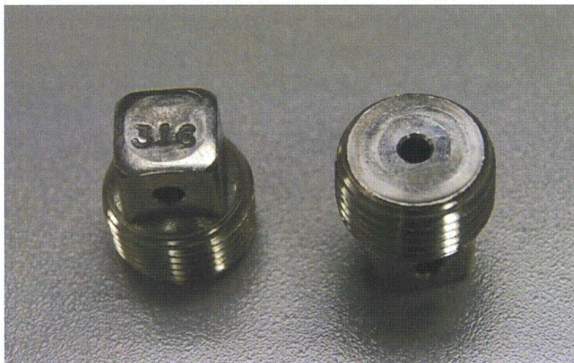
Figure 15 – "T" drain plugs supplied with environmentally qualified MOV motors from Limitorque. These plugs must be installed to maintain environmental qualification of the motor. They shall be oriented at the lowest point of the motor, one on each bearing bracket.
