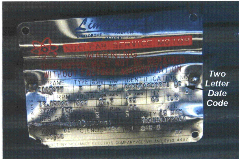
Figure 1 – Month and year of manufacture can be determined by the last two alpha characters in the Identification Number field. This motor has a data code of HC, which corresponds to a manufacturing date of August 2000 as shown on Appendix 1, Reliance Electric Motor Corporate Date Code.
