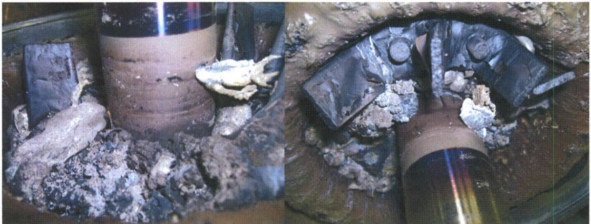
Figure 30 - Failed magnesium rotor. Note angularity of rotor fins relative to shaft and globs of molten magnesium. Note this is shown with the bearing bracket removed in a shop environment.
