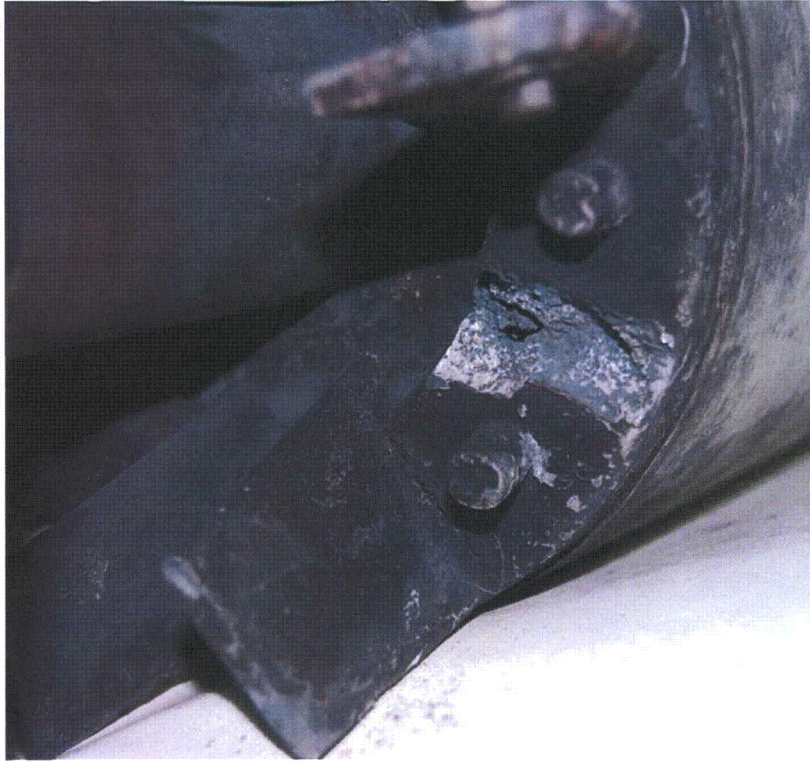
Figure 36 – Magnesium rotor with black corrosion product build-up between the rotor end lamination and the magnesium end ring. NOTE: one cooling fin has broken off the end ring.
