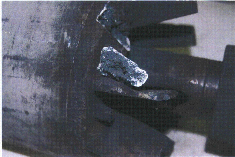
Figure 27 – Rotor with cooling fan/magnesium end ring detached.
