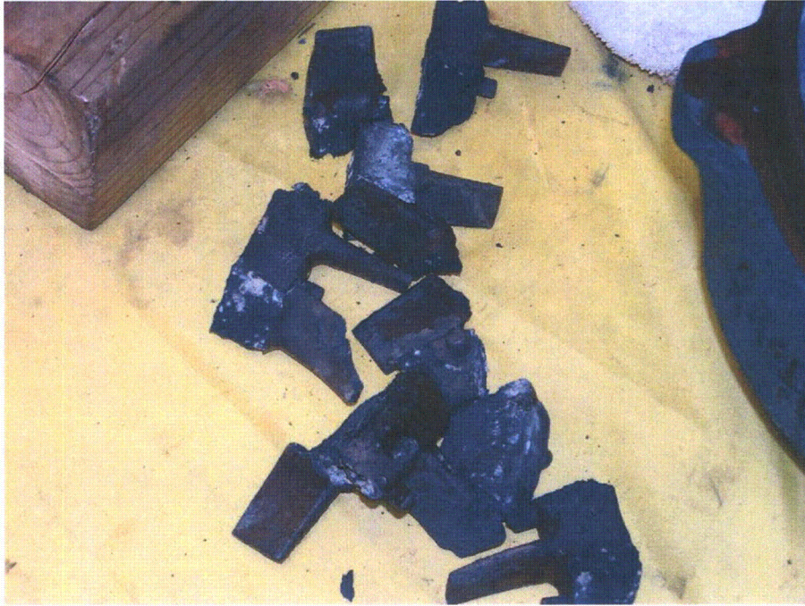
Figure 29 – Catastrophic failure of magnesium end ring.
