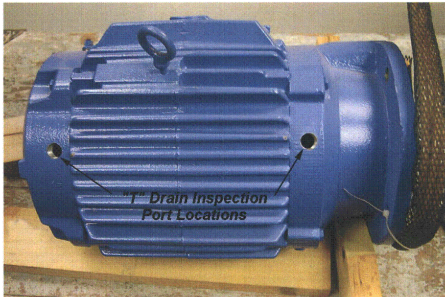
Figure 17 - "T" drain inspection port locations. There are other locations clocked on the bearing brackets that have NPT pipe plugs inserted. Use the "T" drain and other pipe plug locations for borescope inspection.
