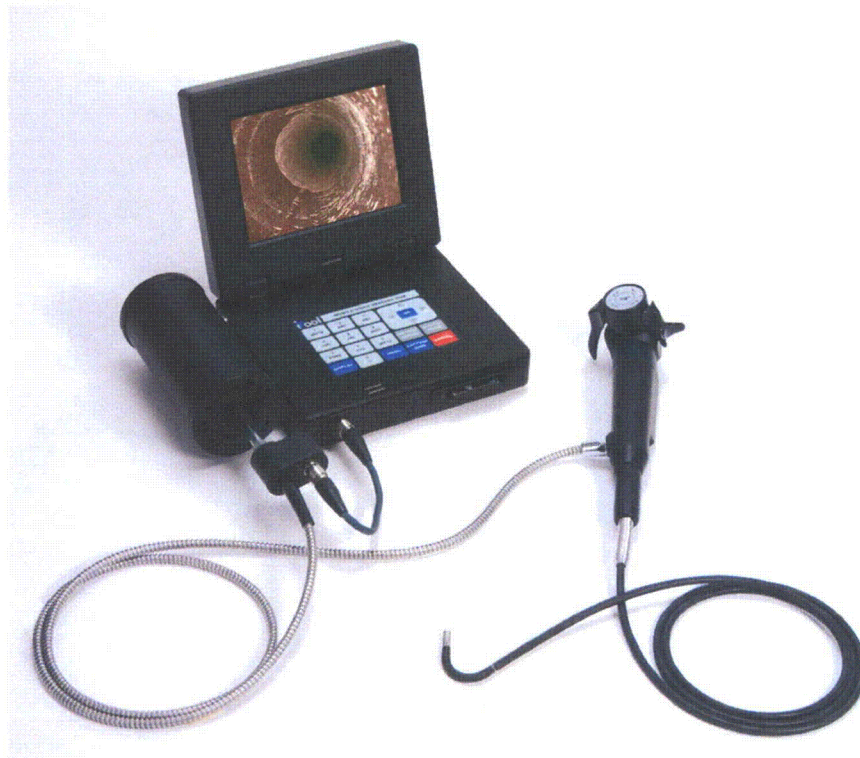
Figure 12 – iTool videoscope. It consists of the computer, the light source (cylinder on left hand side) and four way articulating probe.
