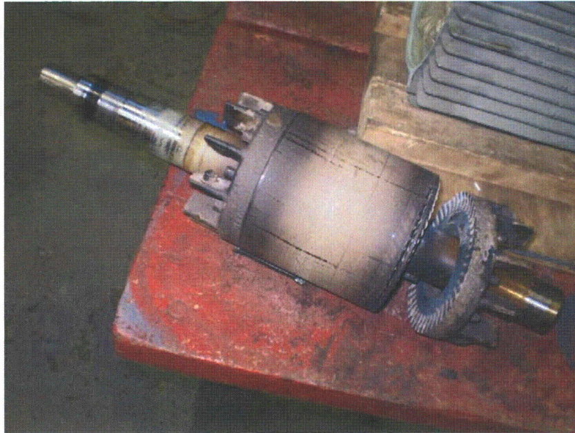
Figure 5 – 150 lb-ft magnesium rotor after removal from stator frame. Note the heavy heat damage on the magnesium rotor end rings as compared to that apparent on the center body of the rotor.
