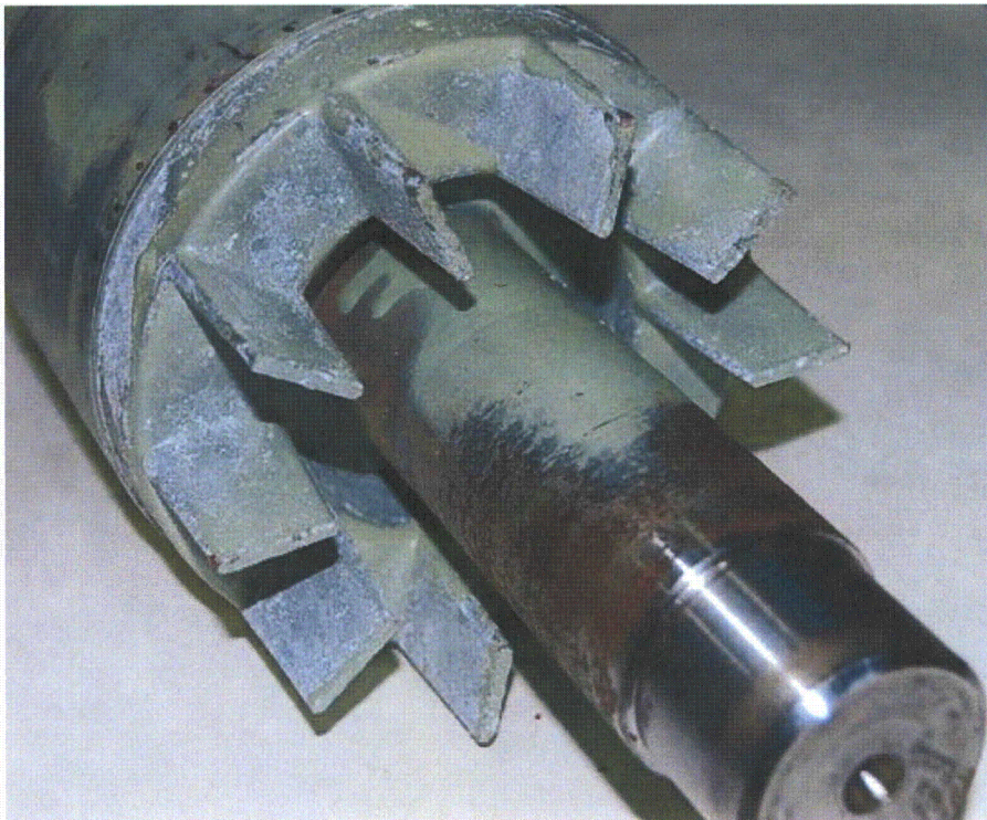
Figure 3 – General corrosion on magnesium end ring.
