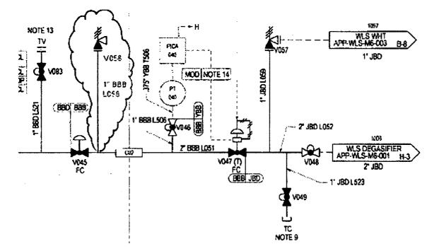
Modify DCD Figure 9.3.6-1, Chemical and Volume Control System as shown:
