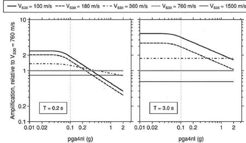
**Figure 5.** Combined amplification for  $T=0.2$  s and  $T=3.0$  s as function of  $pga4nl$ , for suite of  $V_{S30}$ . Note at short periods (left graph), purely linear amplification does not occur on soft soils until  $pga4nl < 0.03$  g.
