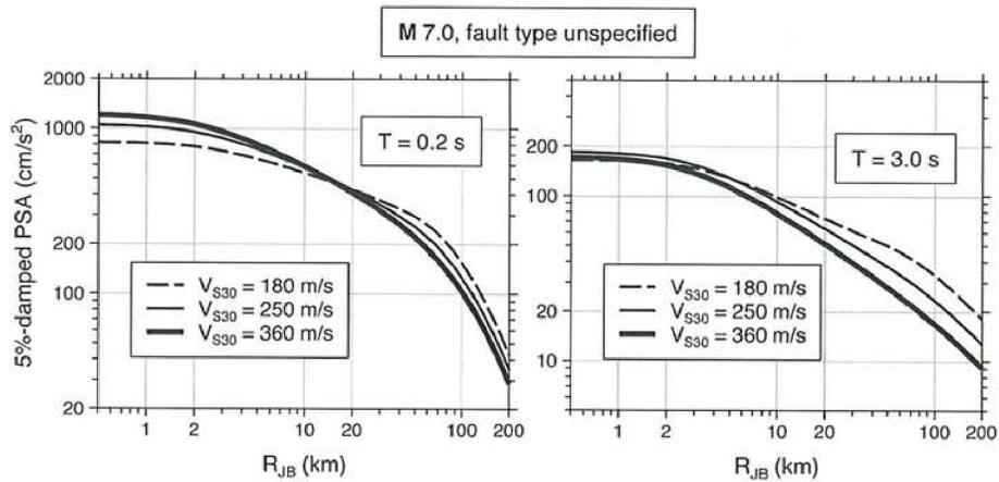
**Figure 12.** PSA from our equations, as a function of distance for magnitude 7, fault type unspecified, and three values of  $V_{S30}$ . Note that the same vertical scale was used for both graphs in order to compare the magnitude scaling for the two periods.
