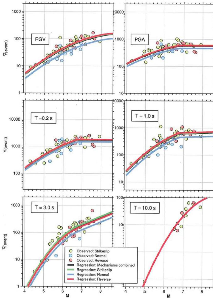
**Figure 9.**  $\bar{Y}(event)$  (the antilog of the average of the log of the motions for each event adjusted to the reference distance of 1 km and the reference velocity of 760 m/s; in the terminology of Equations 14 and 15,  $\bar{Y}(event) = \exp(c_0(event))$ ) and Stage 2 regression fits. Note that the same vertical scale was used for all graphs in order to compare the magnitude scaling from period to period.
