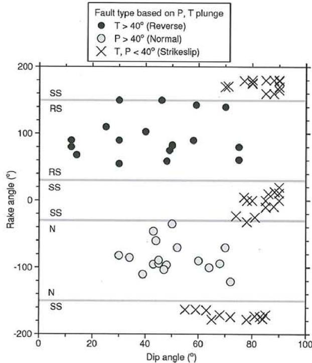
**Figure 1.** Distribution of the data we used in rake-angle and dip-angle space. The horizontal gray lines indicate boundaries between fault types used by BJF97, and the symbols and colors indicate our classification based on the plunges of the  $P$ - and  $T$ -axes (our classification scheme is indicated in the legend; see Appendix D in BA07).
