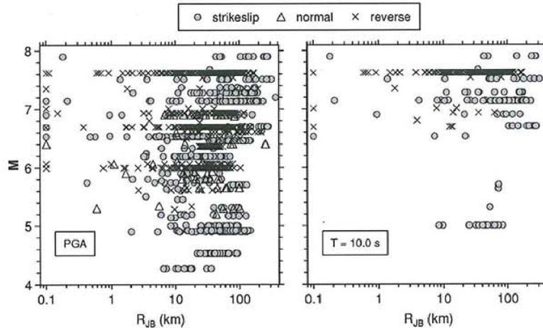
**Figure 2.** Distribution of data used to derive our regression equations for PGA and for PSA at a period 10.0 s, differentiated by fault type (points with  $R_{JB}$  less than 0.1 km plotted at 0.1 km). The overall distributions for periods less than about 4 s are similar to those for PGA, although there are fewer recordings (the number of available recordings decreases noticeably for periods longer than 2 s).
