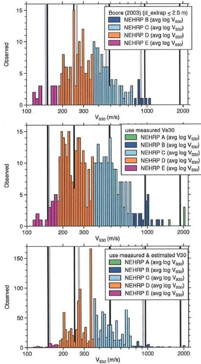
**Figure A1.** Histograms used to determine value of  $V_{S30}$  to use in evaluating NGA GMPEs for a particular NEHRP class (gray vertical lines are the geometrical means of the  $V_{S30}$  in each NEHRP site class, and black vertical lines are recommended values for each NEHRP class, as given in the second-to-last column in Table A1).
