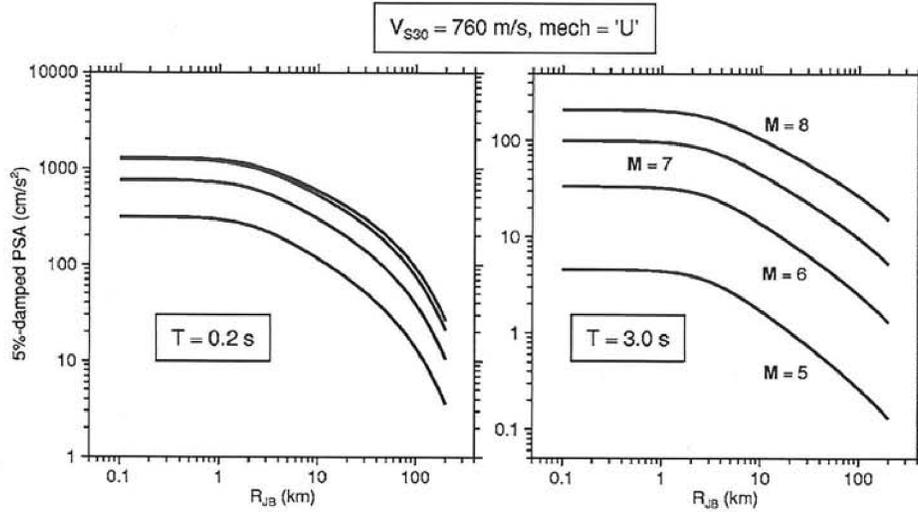
**Figure 11.** PSA from our equations, as a function of distance. The spectra are shown for magnitudes 5, 6, 7, and 8, for fault type unspecified and  $V_{S30} = 760 \text{ m/s}$ . Note that the same vertical scale was used for both graphs in order to compare the magnitude scaling for the two periods.
