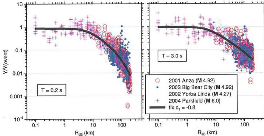
**Figure 6.** Normalized ground motions for four events, using extended data set (more data than in NGA Flatfile). Black curve is regression fit obtained with constraints  $c_1 = -0.8$  and  $c_2 = 0.0$ .
