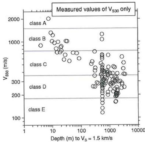
**Figure 14.**  $V_{S30}$  plotted against one measures of basin depth: the depth to a shear-wave velocity of 1.5 km/s. All values in the NGA Flatfile with basin depths and measured (rather than estimated) values of  $V_{S30}$  are shown.
