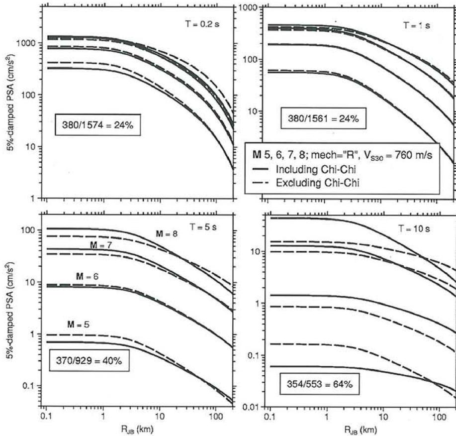
**Figure 16.** Comparisons of PSA for four periods from equations developed with and without 1999 Chi-Chi mainshock. Ratios are number of Chi-Chi recordings used to develop final equations divided by total number of recordings.
