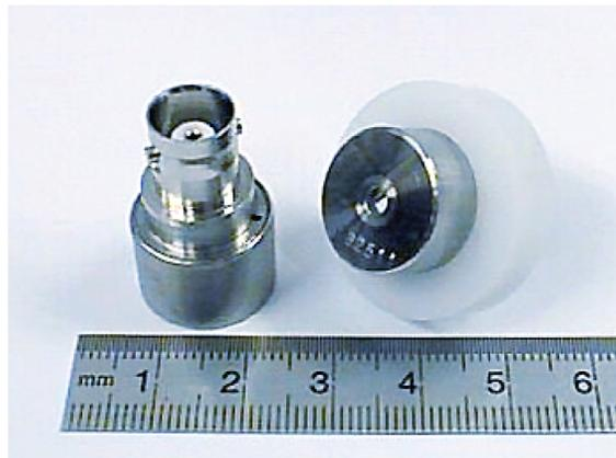
Figure 04.04-4-24: Typical AMS Table Activation Detector
