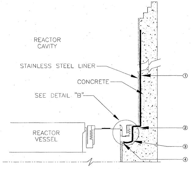
DRYWELL AND REACTOR CAVITY SECTION DETAIL "A"
