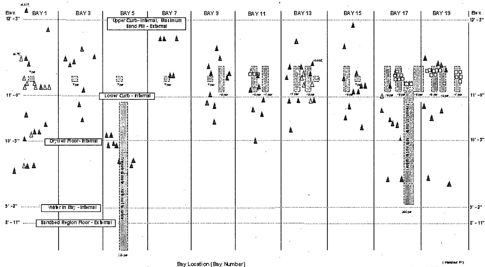
For illustration of measurement locations in each bay. Vertical dimensions to scale showing approximate measurement locations. Horizontal dimensions not to scale to the individual bays.
