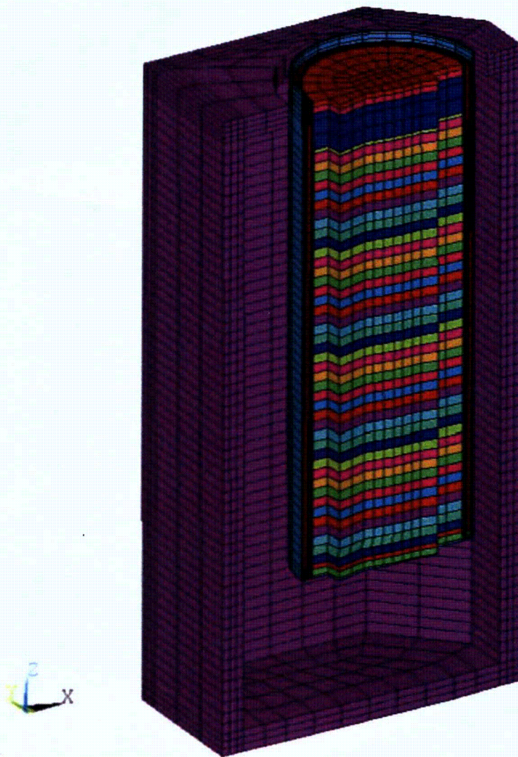
Figure 10. ANSYS Representation of Naval Short Waste Package in Waste Package Transfer Trolley Shielded Enclosure in Room 1006 (Close-up, Cut-away View, Room Not Shown)
