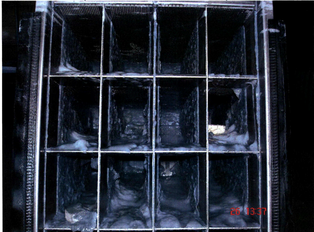
Figure 3-21: Test 3 Open Area with 100% Non-Chemical and Chemical Debris (Photo Taken After Draindown)
