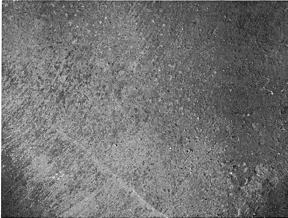
Figure 3-7 Ground Surface Condition Evaluated on BWR/3 Beam Removed from Quad Cities Unit 1 Beam. Typical of all Removed Beams
