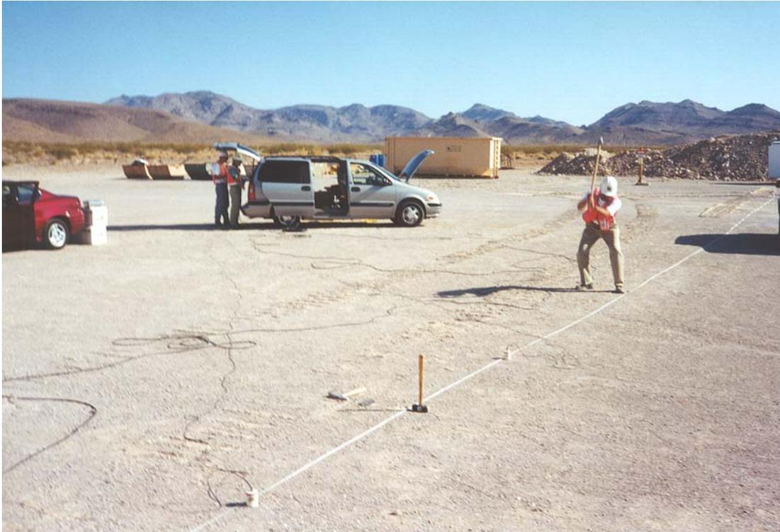
Figure 45. Using the Sledgehammer Source at SASW-23
