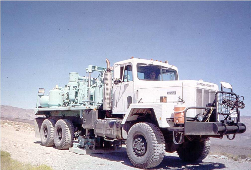
Figure 158. Photograph of Vibroseis Truck in Operation on the Crest of Yucca Mountain
