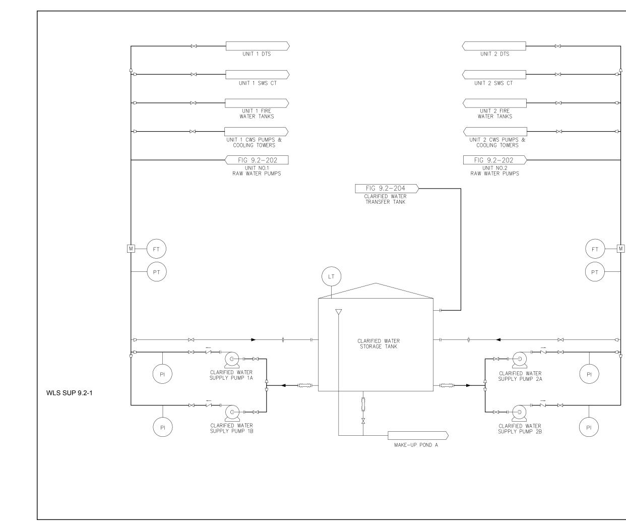
Raw Water System, Clarified Water Subsystem FIGURE 9.2-205
