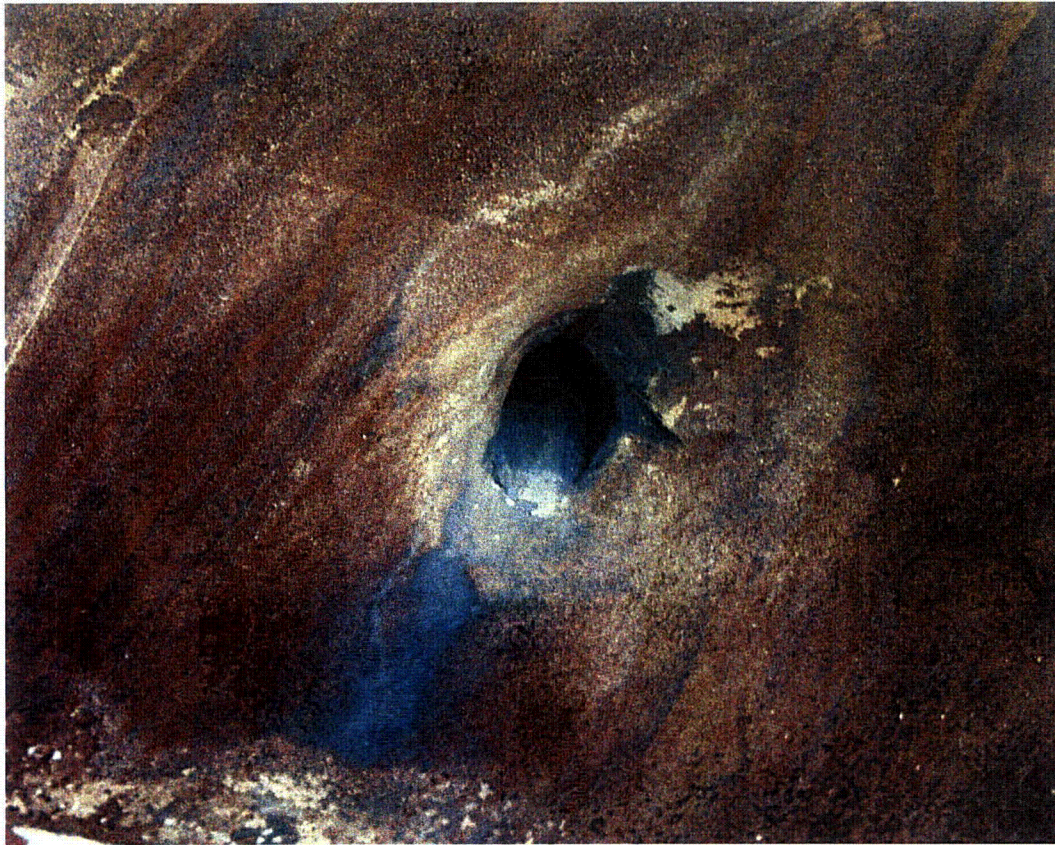
Figure 1.3. Puncture in Tank Car
