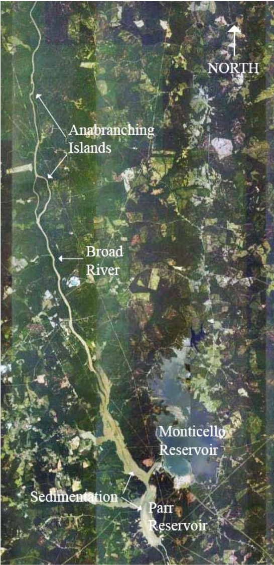
Figure 2.3-17. Backwater Effects from Parr Reservoir Extend Thirteen Miles Upstream
