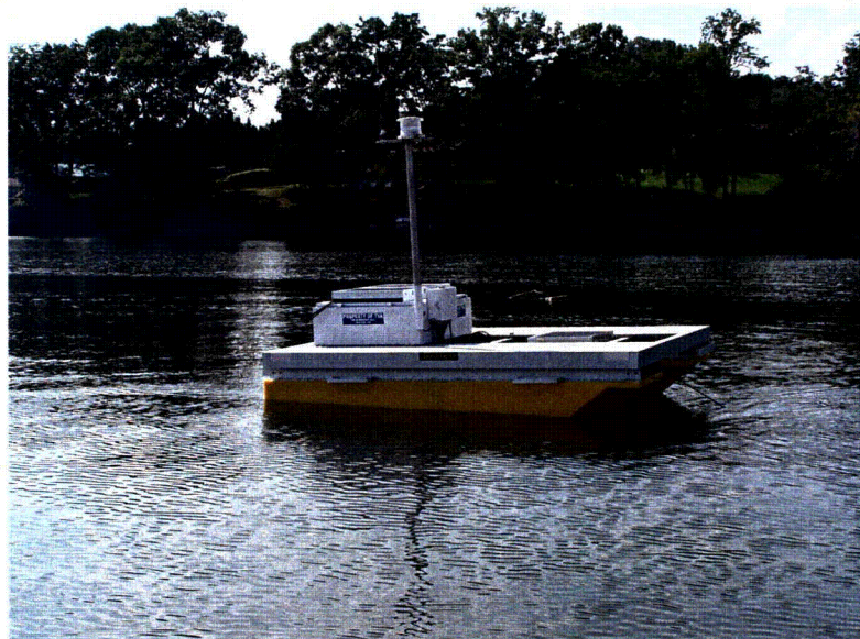
Figure 34. Station 14 Floating Water Temperature Station
