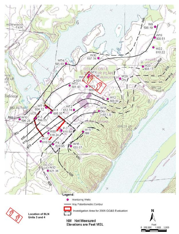
Note: The March 2005 reading from Well W29 is considered an anomalous reading, and the water level and interpretation of the groundwater elevations in the vicinity of Well W29 depicted in this figure are not considered in current groundwater evaluations.
