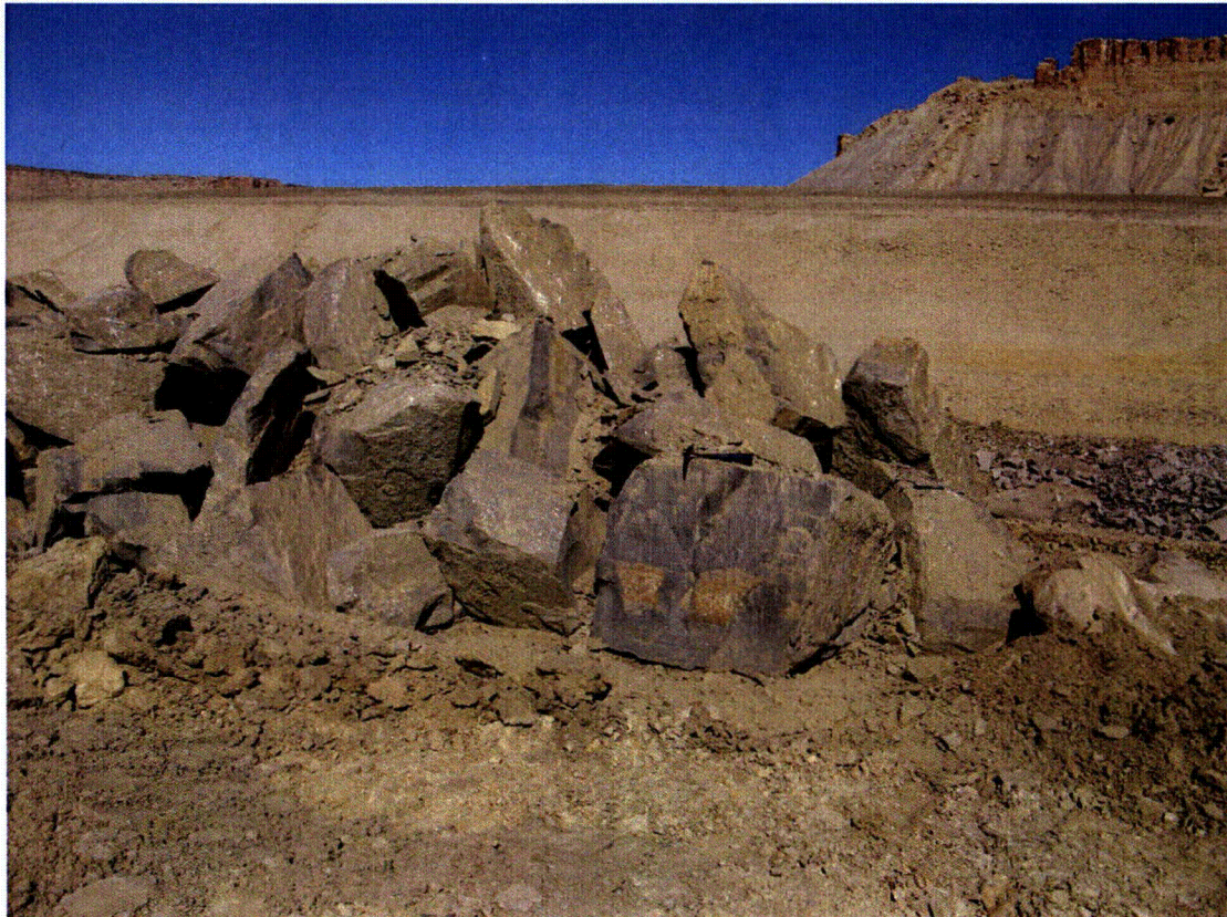
Figure 11. Stockpiled Dolomitic Limestone as Much as 3 Ft Thick Encountered During Initial Excavation Into Bedrock South of Location 1 of September 23
