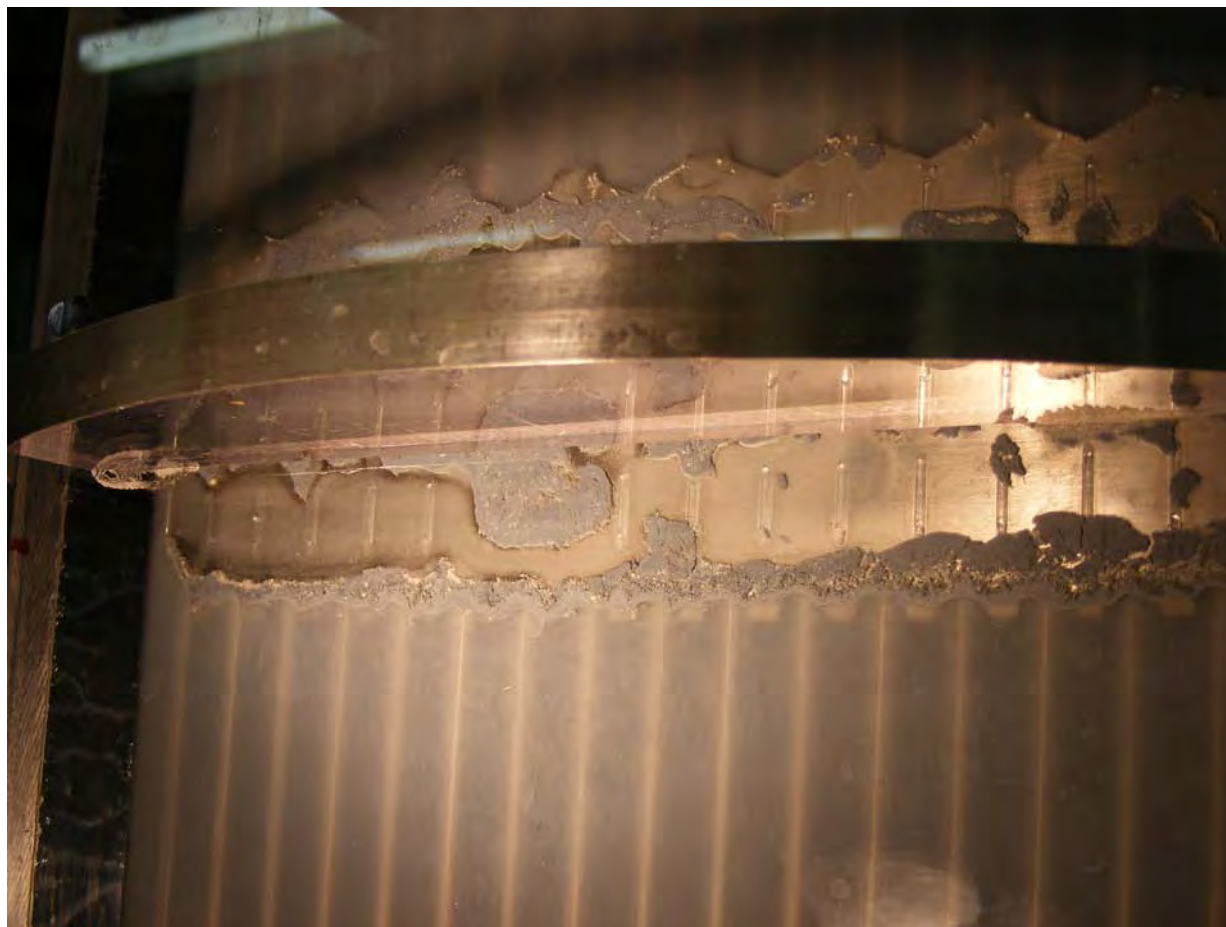
Sample of Debris Collection at Grid
