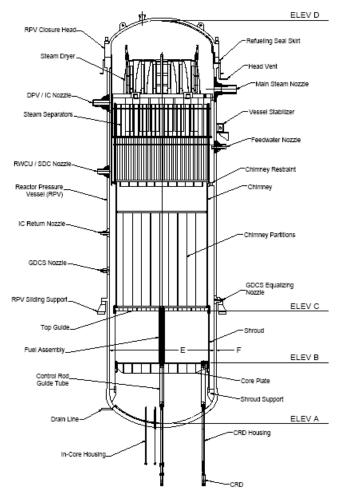
Figure 2.1.1-1. Reactor Pressure Vessel System Key Features Layout
