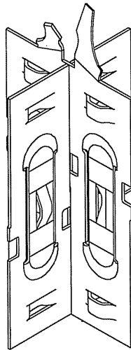
Figure 4.2.1-1 Mitsubishi Grid Spacer (Z3 Type) Schematic View
