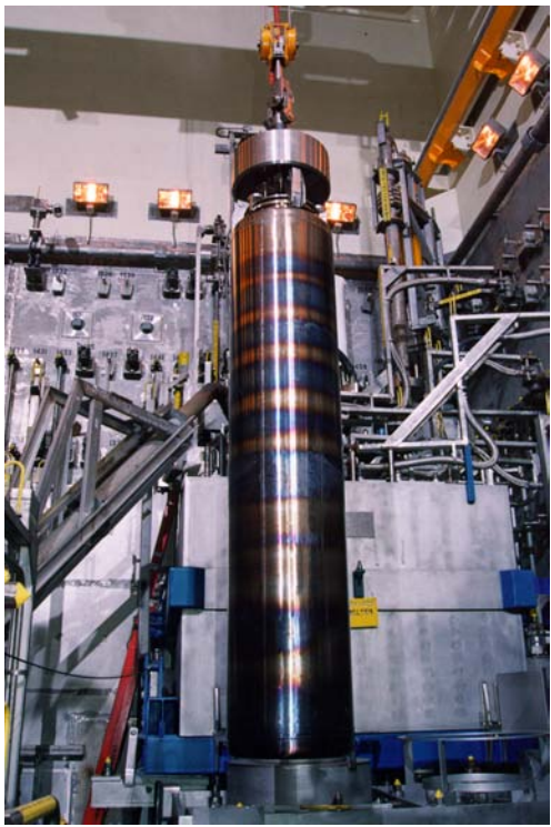
Top: Fuel rods are bundled together into fuel assemblies as shown here. These fuel assemblies are for a boiling water reactor. Bottom: Canister of high-level waste from the West Valley Demonstration Project. The canister is 2 feet (0.6 meter) in diameter, 10 feet (3 meters) long, and weighs about 2 metric tons. SOURCES: Top photo courtesy of the Nuclear Energy Institute. Bottom photo courtesy West Valley Nuclear Services Company.
