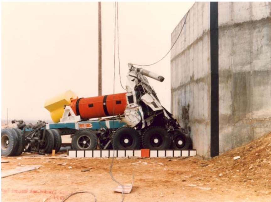
FIGURE 2.5 High-speed (135 kilometers per hour [84 miles per hour]) crash of a spent fuel package mounted on a truck trailer into a massive barrier carried out at Sandia National Laboratories in 1977. The truck cab was destroyed in the crash, but the package remained attached to the trailer. SOURCE: Sandia National Laboratories.
