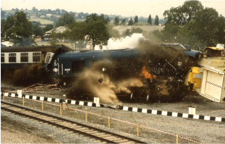
FIGURE 2.10 Full-scale crash test of a Magnox spent fuel package carried out in Leicester, England by the CEBG in July 1984. This photograph was taken just after the locomotive, which was traveling at 100 miles per hour (45 meters per second), collided with the package and flatcar. The collision has lifted the package and flatcar off the ground. SOURCE: Magnox Electric Ltd.
