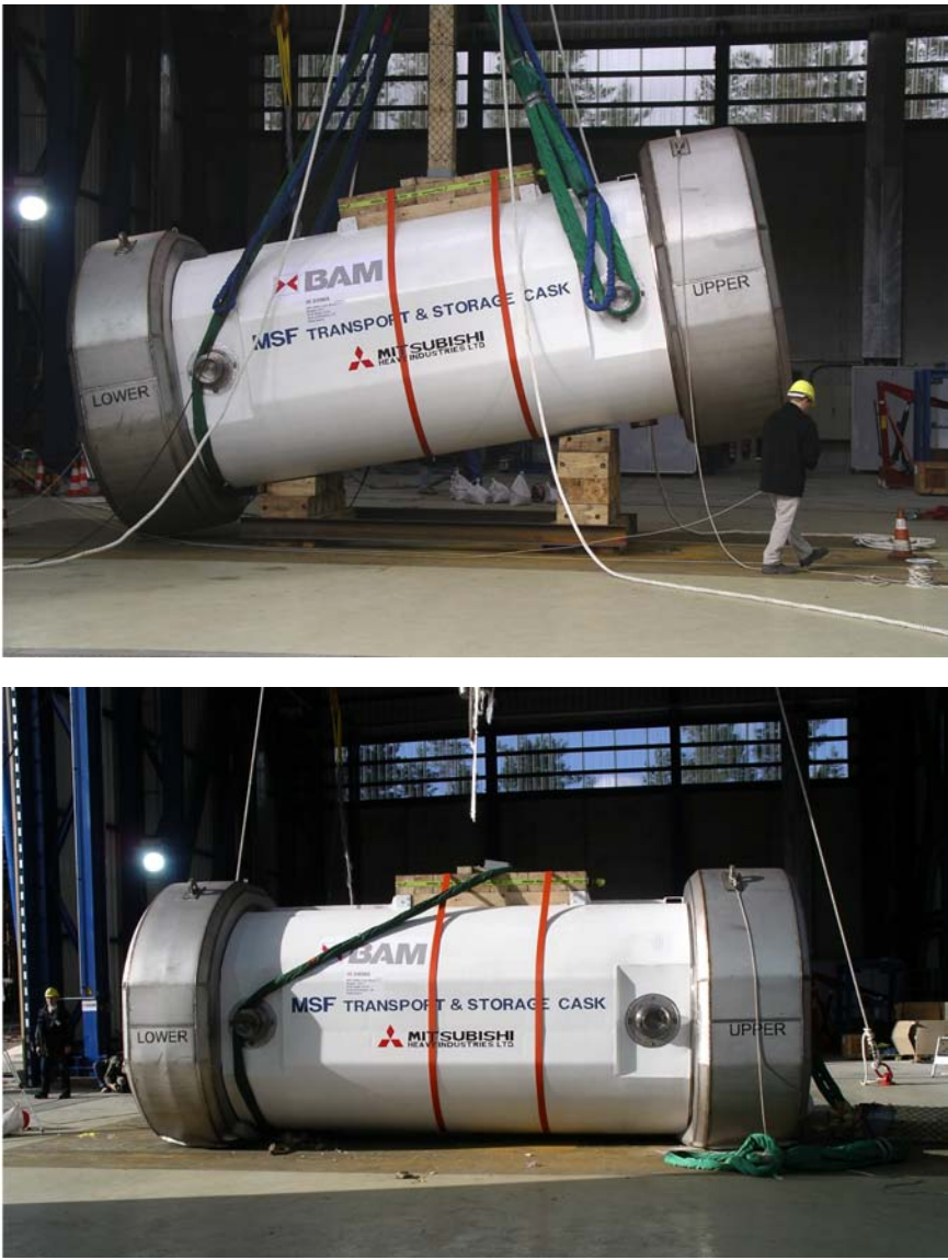
FIGURE 2.2 The German Federal Institute for Materials Research and Testing (BAM) carried out two 9-meter regulatory drop tests in September 2004 at its recently completed testing facility near Berlin. One of the tests was conducted on the 180 metric ton (198 short ton) Mitsubishi rail package shown in these photos. The top photo shows the package orientation for this test. The package was hoisted and dropped onto the steel plate embedded in the floor. The bottom photo shows the package after the test. SOURCE: Photo by K.D. Crowley.
