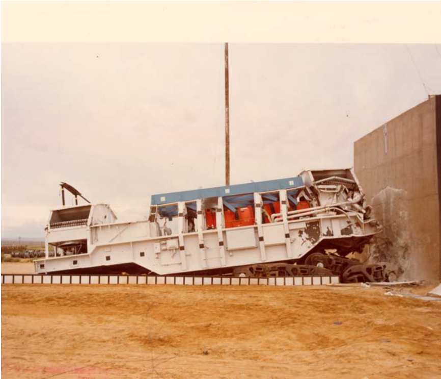
FIGURE 2.7 High-speed (131 kilometers per hour [82 miles per hour]) crash of a spent fuel package mounted in a railcar into a massive barrier carried out at Sandia National Laboratories in 1977. The railcar was destroyed in the crash, but the package sustained only superficial damage. SOURCE: Sandia National Laboratories.
