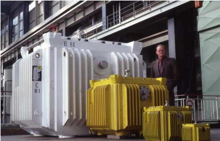
Full-scale (background) and \frac{1}{2} -, \frac{1}{4} -, and \frac{1}{8} -scale models (foreground) of the Magnox flask. SOURCE: Magnox Electric Ltd.
