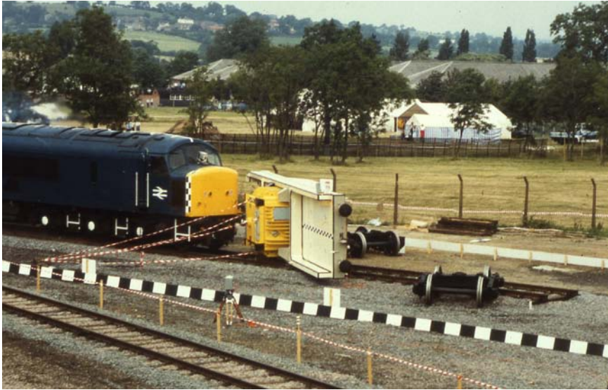
FIGURE 2.9 Configuration for the July 1984 full-scale crash test of a Magnox spent fuel package carried out in Leicester, England by the CEGB. The Magnox package was mounted on a flatrol railcar, which was turned on its side and laid diagonally across the track as shown in this photograph. The wires leading away from the package are connected to instruments for monitoring conditions during the early phases of the crash. SOURCE: Magnox Electric Ltd.
