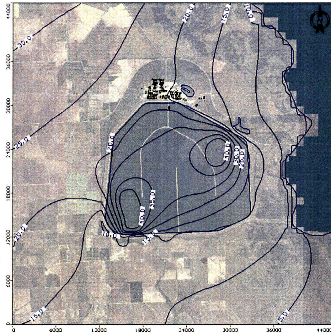
Figure 60: Simulated Groundwater Contours (Run 101) – Before Construction of STP 3 & 4 - Model Layer 2 (Stratum C)
