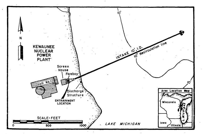
Figure 1. Schematic of Kewaunee Nuclear Power Plant showing plant location and entrainment sampling site, April 1975 through March 1976.
