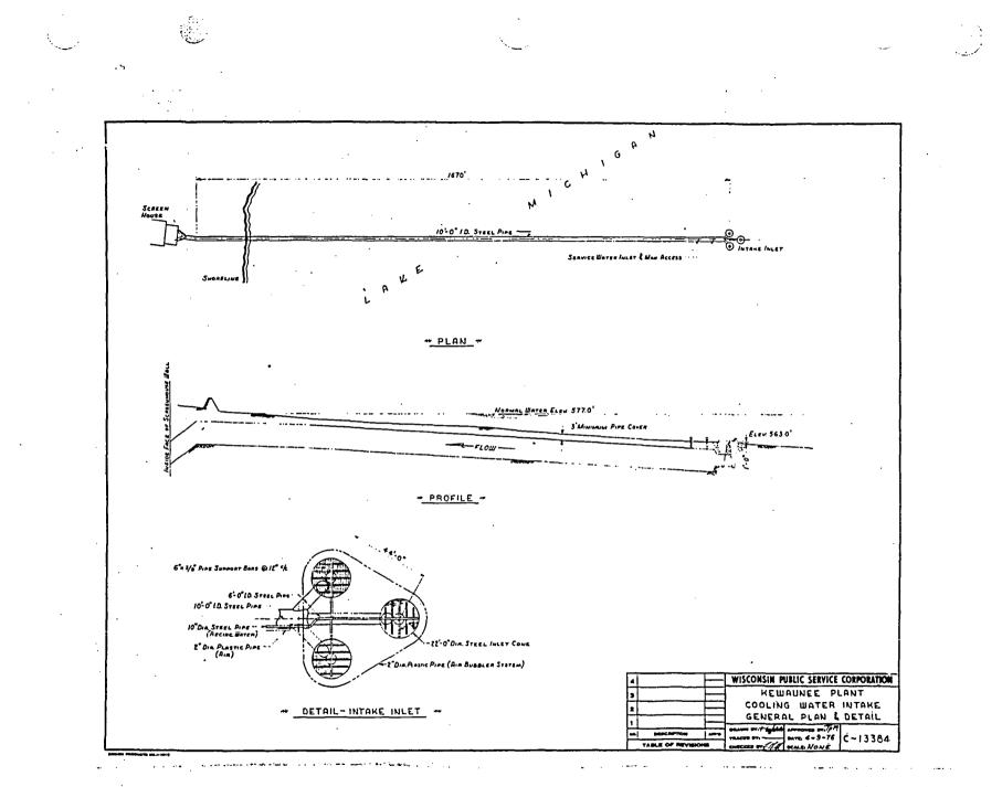
Figure 2. Description of intake inlet and pipe in relation to the bottom contour of Lake Michigan at Kewaunee Nuclear Power Plant.
