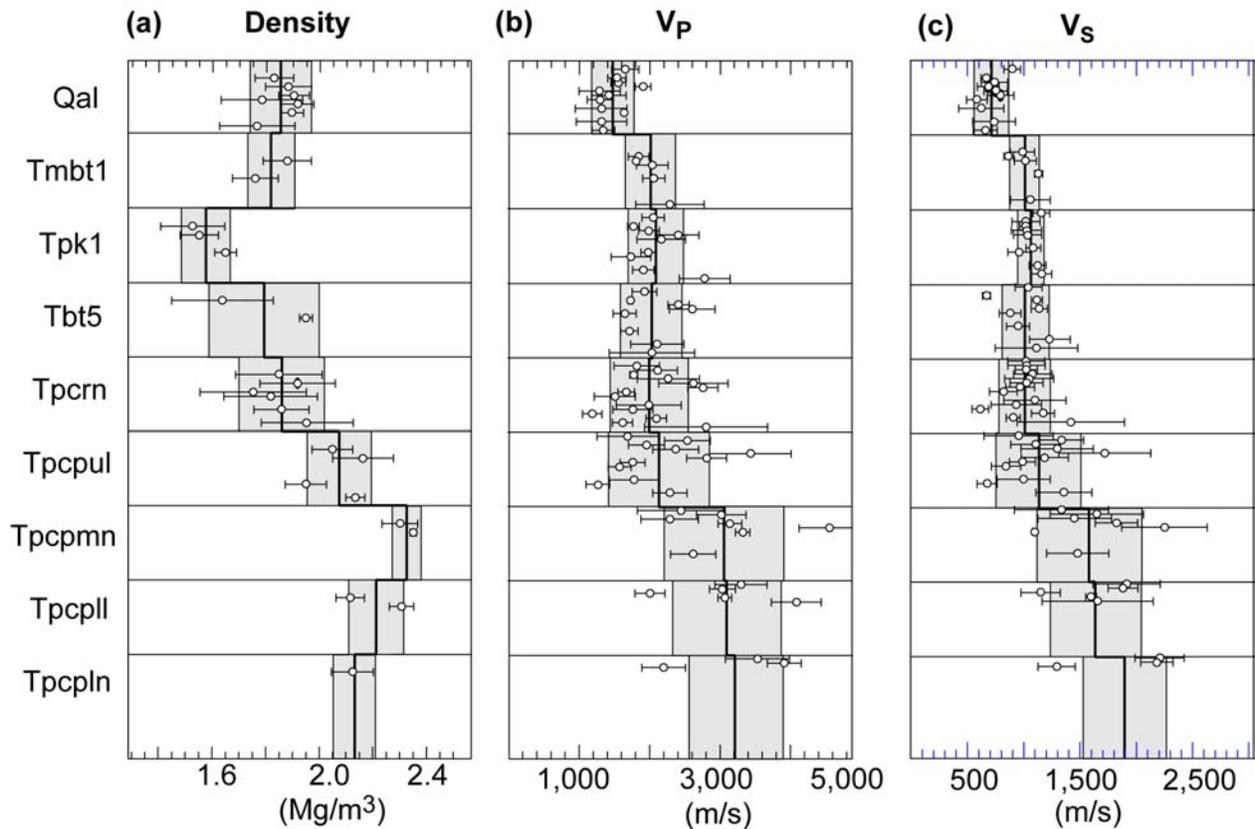
**Figure 3-5. Density Shown in (a), V<sub>p</sub> Shown in (b) and V<sub>s</sub> Shown in (c) Plotted as a Function of Stratigraphy. The Circles With 1-Sigma Error Bars are The Mean Values from Each Borehole Where Velocity or Density Data For That Unit were Obtained. The Thick Black Line With 1-Sigma Shaded Error Band is the Weighted Mean of the Borehole Data.**
