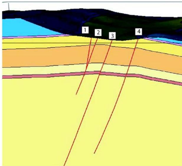
**Figure 2-5. EarthVision® Model Exhibiting the Small Offsets of Faults 1, 2, 3, and 4. View Is to the North With No Vertical Exaggeration. Model Is Sliced at Northing 4078481. See Figure 2-1 For Map View of Fault Locations.**
