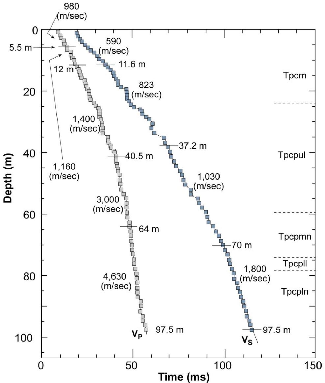
Figure 3-2. DOE Velocity Data from Down Hole Measurements at Borehole RF#15, The Velocity Intervals and Values Are Noted. The Data Were Scanned and Then Regraphed from Figure V-3 in Bechtel SAIC Company, LLC (2002).
