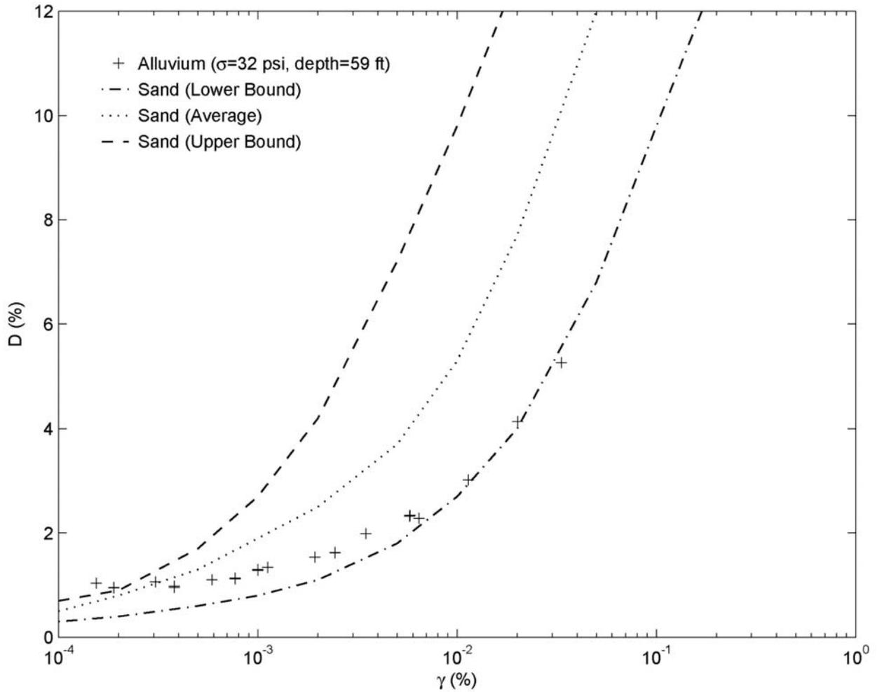
**Figure 3-8. Damping Ratio Results for the Alluvial Sample from the Proposed Waste Handling Building (Modified from Bechtel SAIC Company, LLC, 2002). Also Shown for Comparison are Average, Upper, and Lower Bound Sand Curves.**
