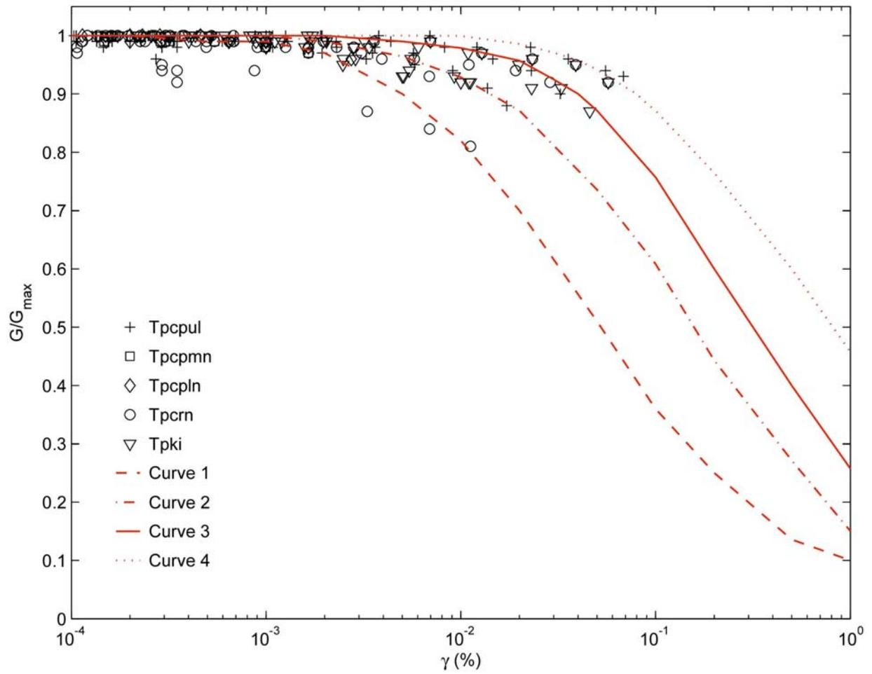
**Figure 4-11. Range of Tuff Normalized Shear Modulus Curves Used for Ground Response Calculations (Modified from Bechtel SAIC Company, LLC, 2002)**
