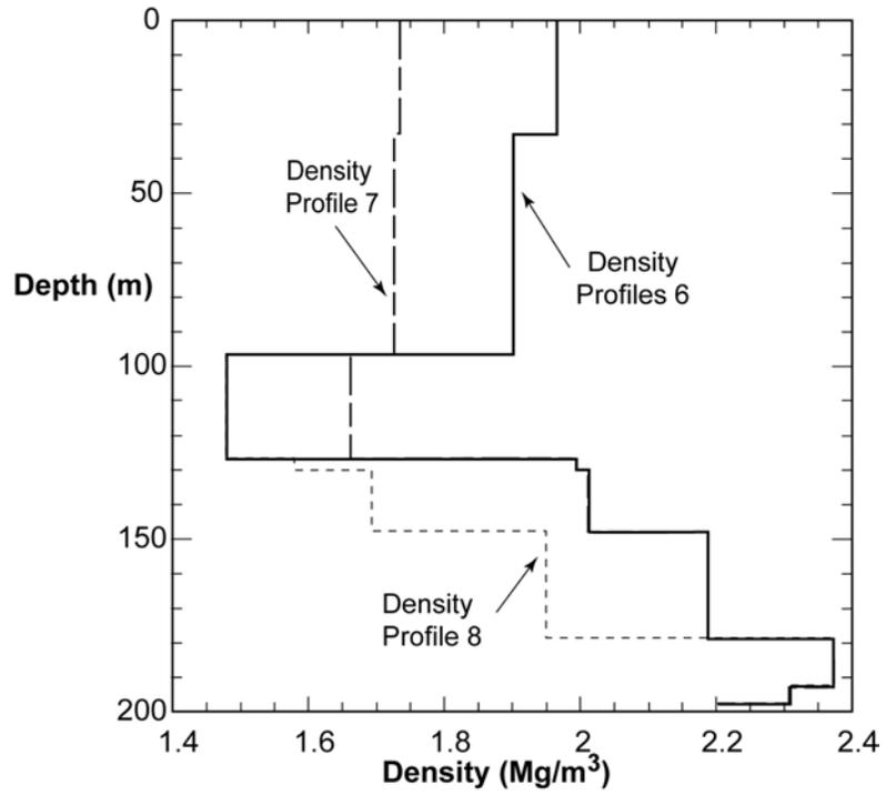
Figure 4-10. Density Profiles 6, 7, and 8 Used in the Ground Response Calculations
