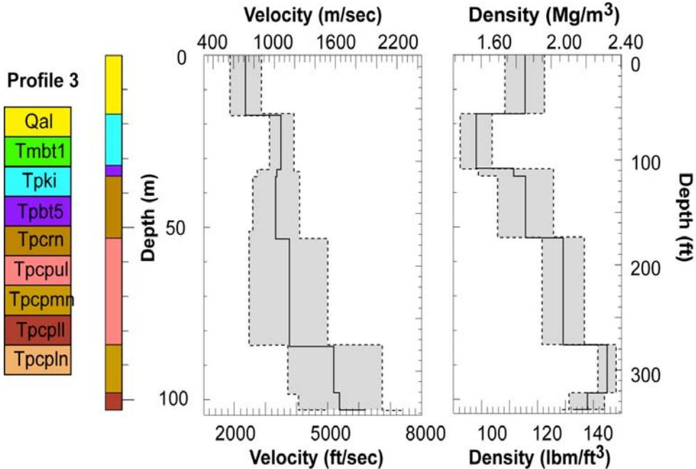
Figure 4-6. Thickness, Velocity, and Density Profile 3 Used in the Ground Response Calculations
