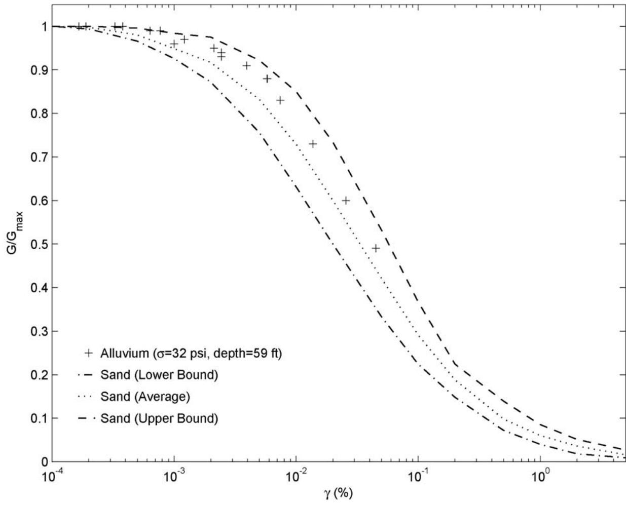
**Figure 3-7. Normalized Shear Modulus Results for the Alluvial Sample from the Proposed Waste Handling Building (Modified from Bechtel SAIC Company, LLC, 2002). Also Shown for Comparison Are Average, Upper, and Lower Bound Sand Curves.**
