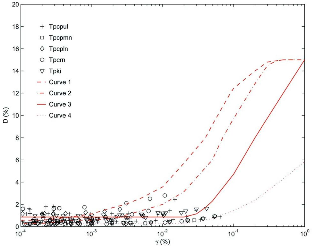
Figure 4-12. Range of Tuff Damping Curves Used for Ground Response Calculations
