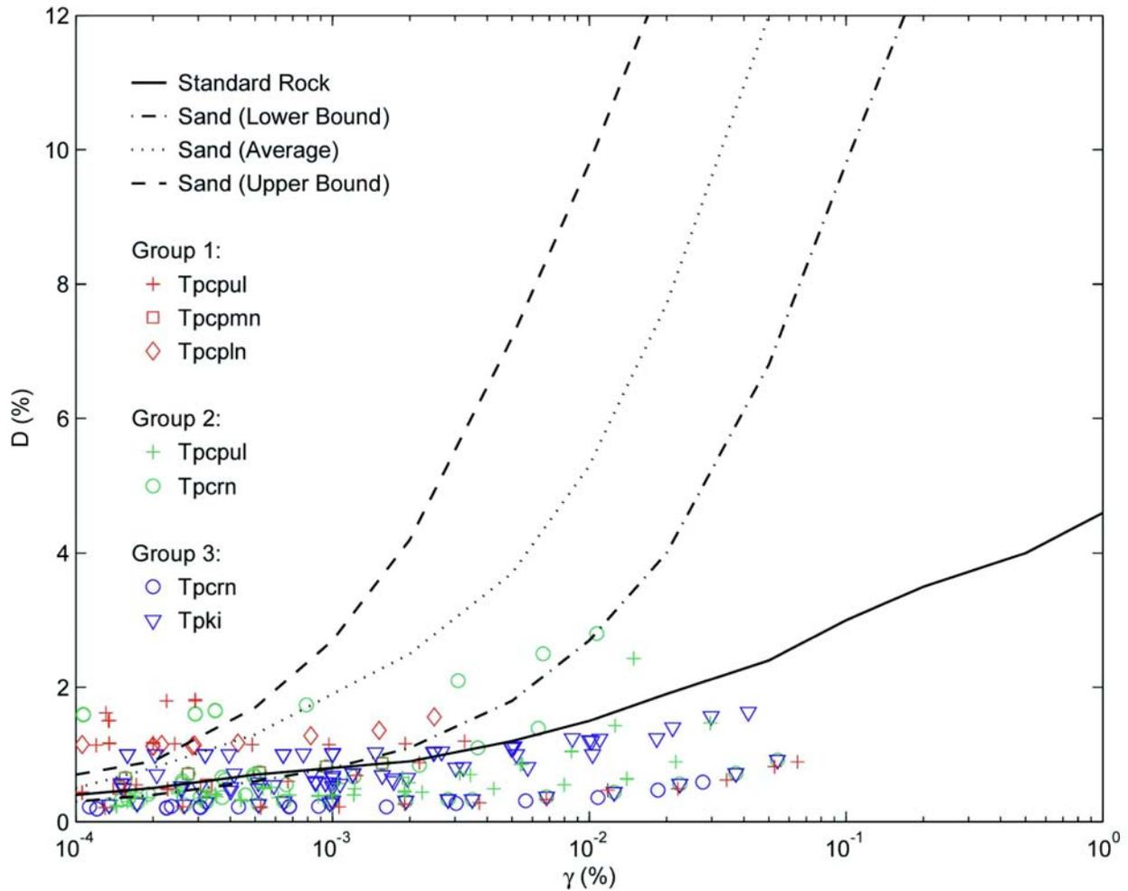
**Figure 3-10. Damping Ratio Data for the Tuff Samples from the Proposed Waste Handling Building (Modified from Bechtel SAIC Company, LLC 2002). Also Shown are Average, Upper, and Lower Bound Sand Curves and a Standard Rock Curve.**
