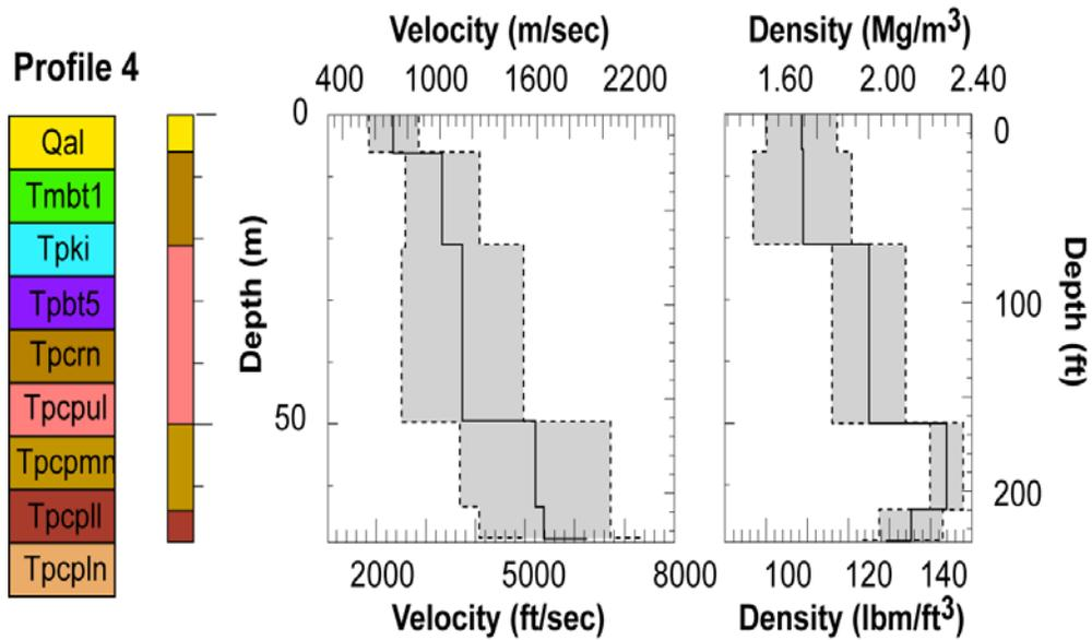
Figure 4-7. Thickness, Velocity, and Density Profile 4 Used in the Ground Response Calculations
