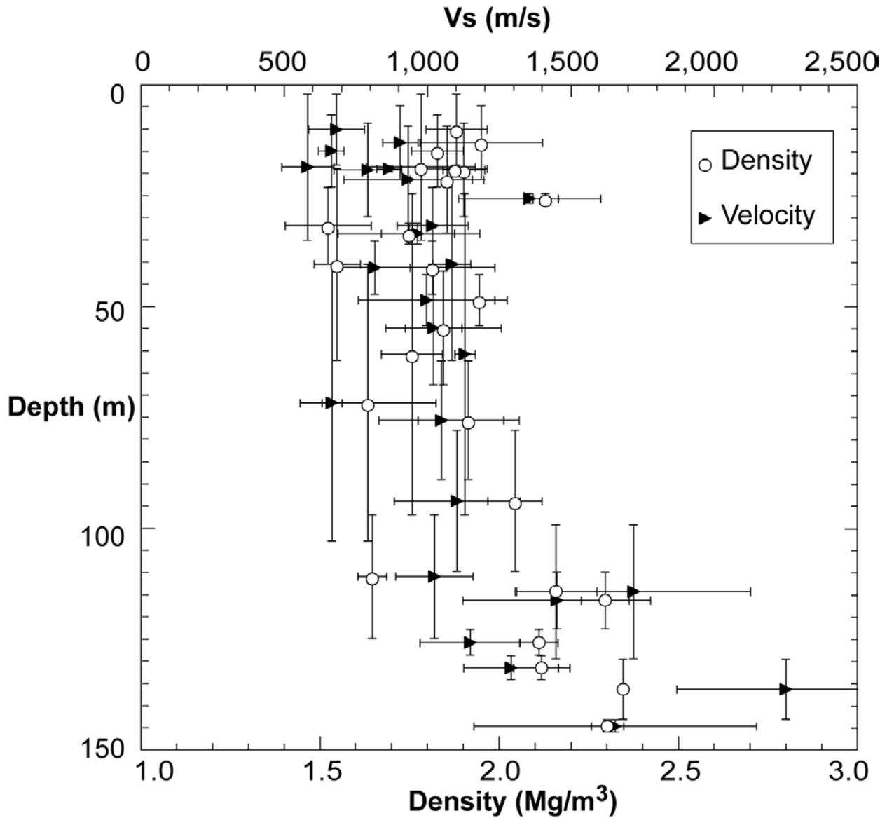
Figure 3-6. Density and Shear-Wave Velocity Plotted as a Function of Depth. The Error Bars for  $V_s$  and Density are the 1-Sigma Errors About the Reported Mean Values. The Error Bars for Depth Plot the Depth Range Over Which The Density or  $V_s$  Were Measured.
