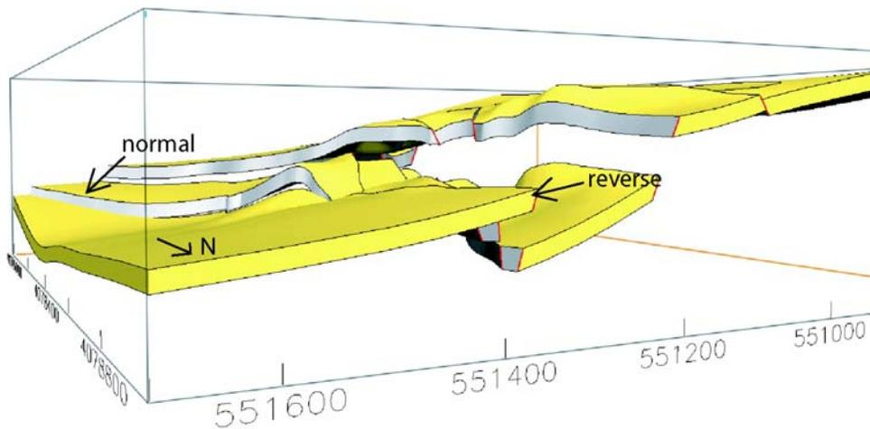
**Figure 2-4. Oblique View of the Tpcrn Layer in the EarthVision® Model Showing the Change in Displacement Along Fault 12. View is to the South-Southwest With No Vertical Exaggeration. Coordinates are UTM, Zone 11.**
