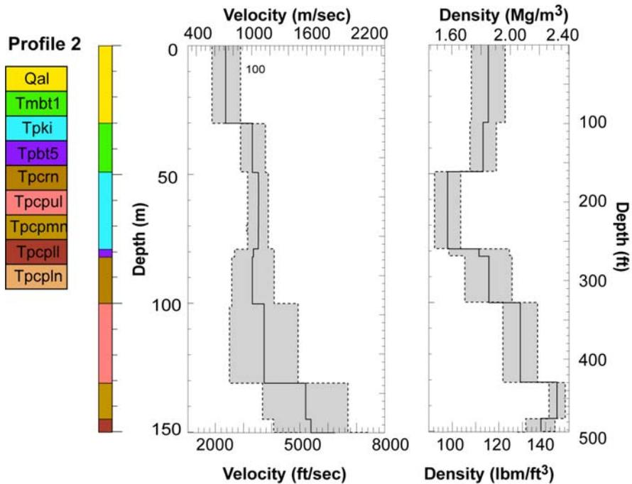
Figure 4.5. Thickness, Velocity, and Density Profile 2 Used in the Ground Response Calculations
