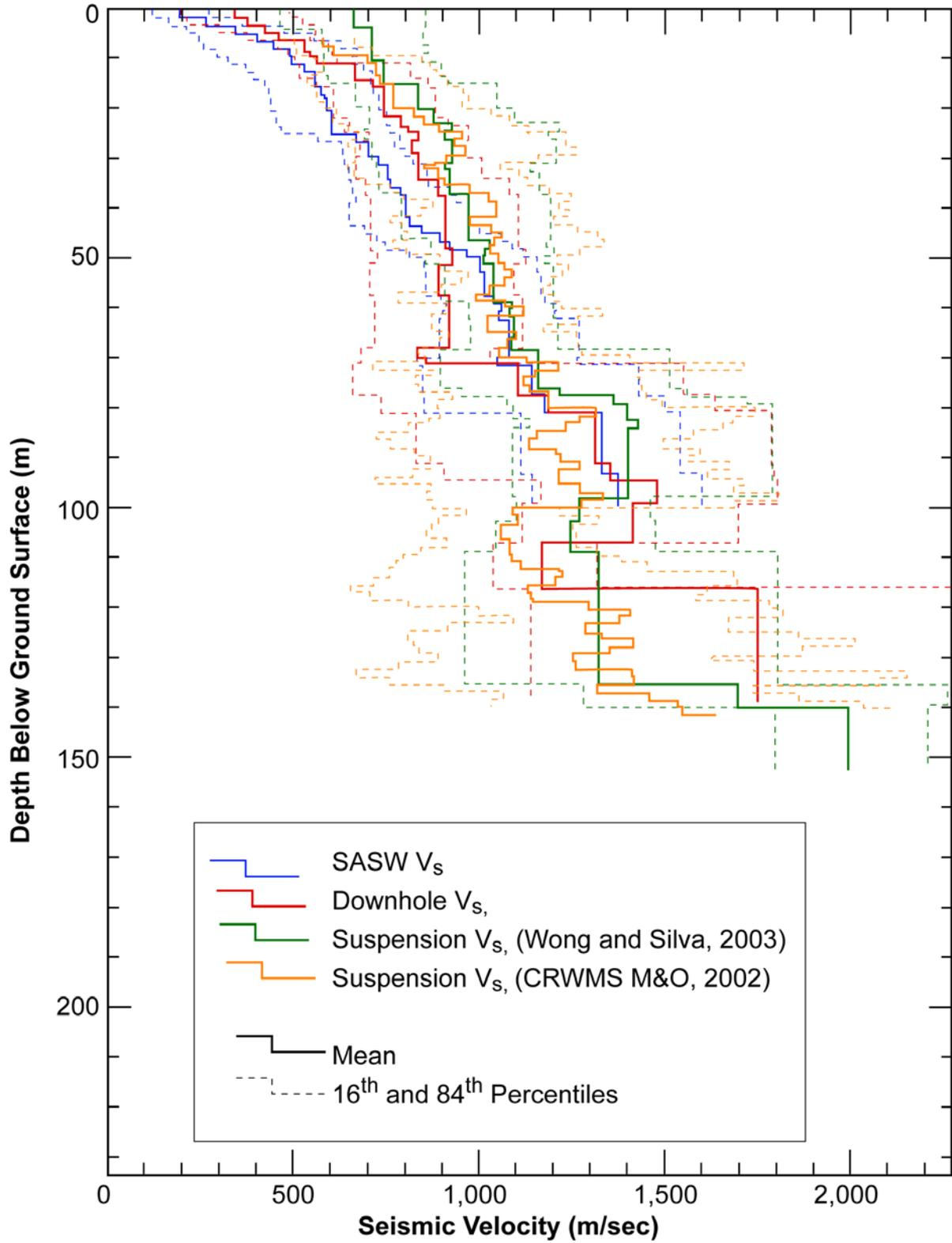
**Figure 3-4. Composite Shear-Wave Velocity Profiles Based on the DOE Data from Conventional Downhole, Suspension Surveys, and Spectral Analysis of Surface Waves Results**
