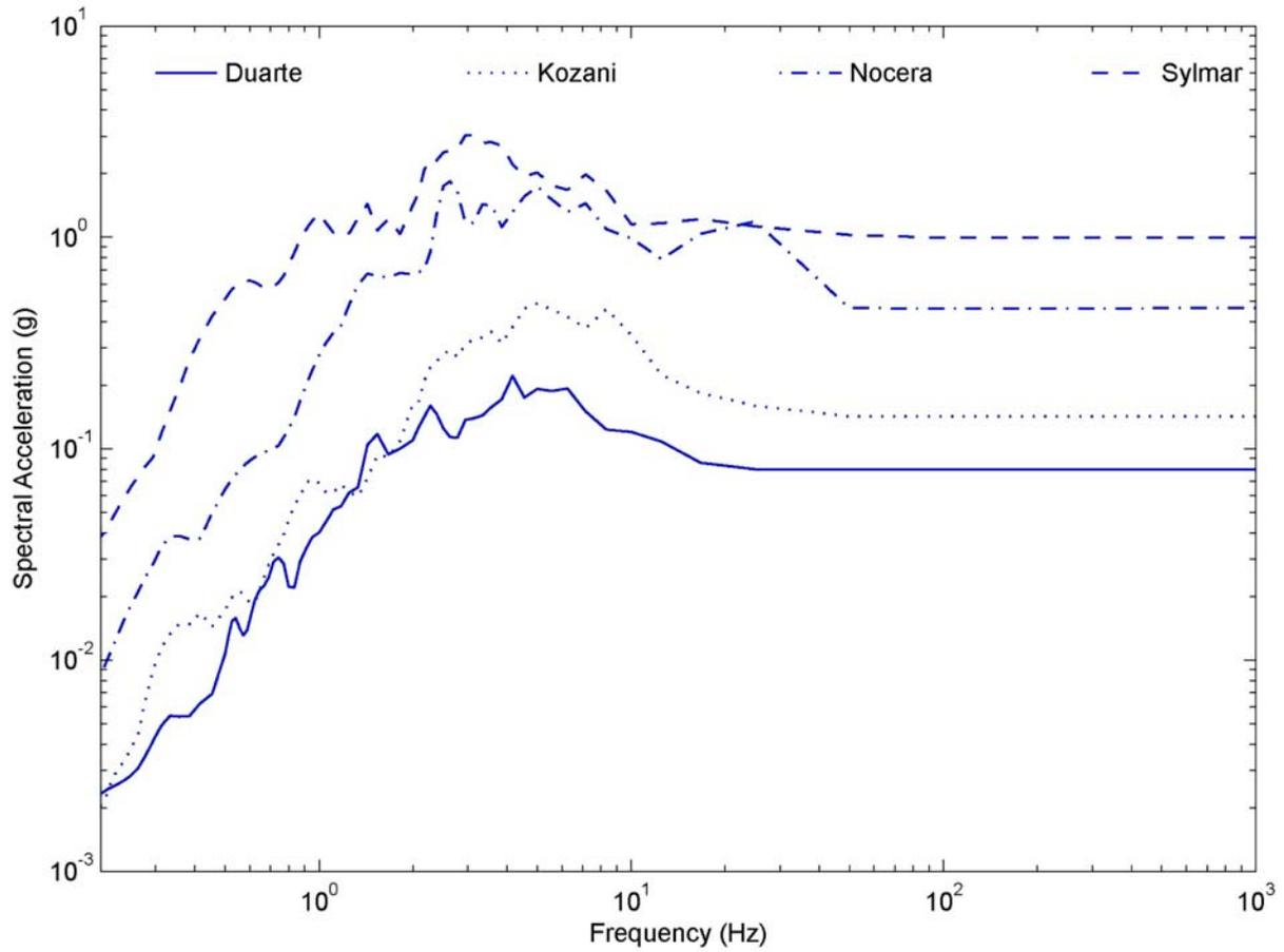
**Figure 4-3. Response Spectra (5 Percent Damped) of Input Time Histories Used in the Ground Response Calculations**
