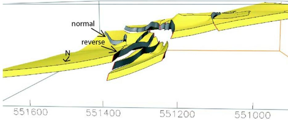
**Figure 2-3. East-West Slice of EarthVision® Model Layer Tpcrn Showing Change in Displacement Along Fault Surface. View Is to the South with No Vertical Exaggeration. Coordinates are UTM, Zone 11.**
