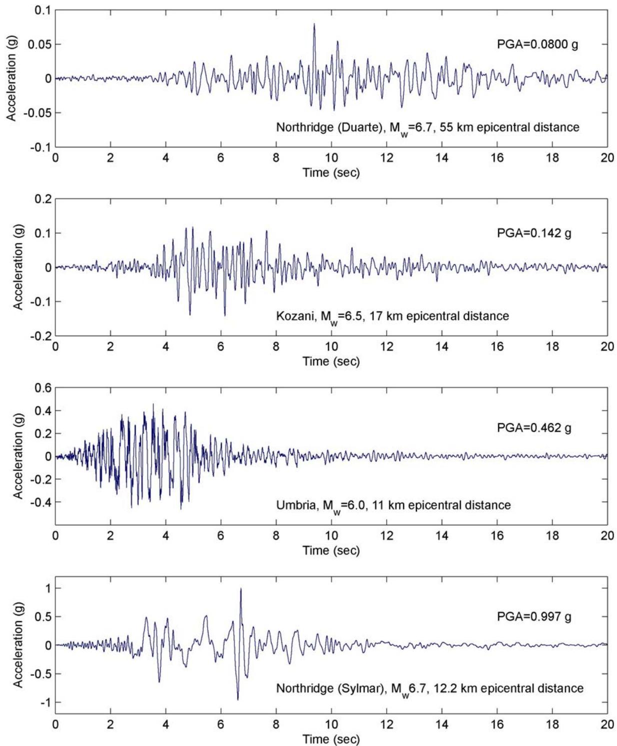
**Figure 4-2. Time History Inputs Used in the Ground Response Calculations**
