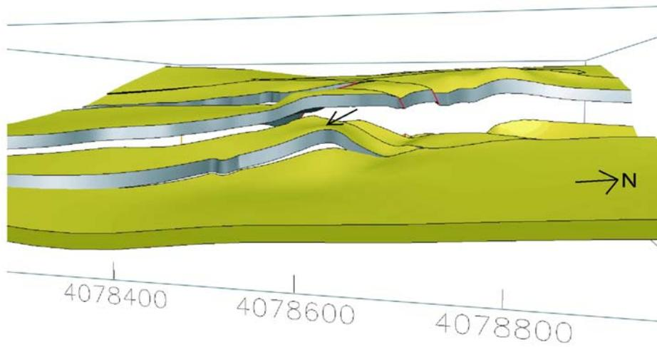
**Figure 2-6. The Structural High Near Fault 12 is Indicated by a Black Arrow. A Fault on Either, or Both, Sides of This Structural High Could Explain its Presence. Stratigraphic Layer Shown is Tpcrn. No Vertical Exaggeration.**
