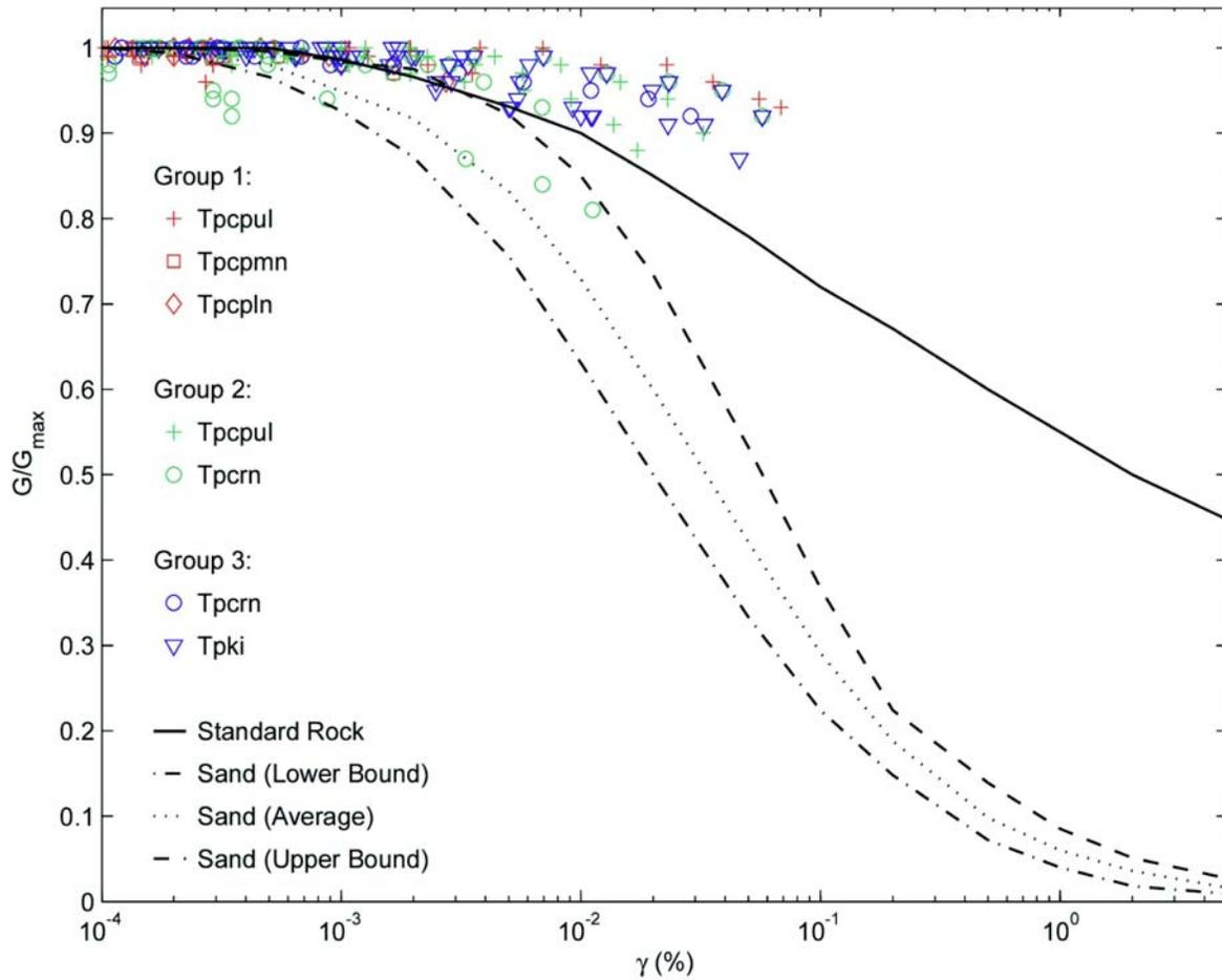
Figure 3-9. Normalized Shear Modulus Data for the Tuff Samples from the Proposed Waste Handling Building (Modified from Bechtel SAIC Company, LLC 2002). Also Shown are Average, Upper, and Lower Bound Sand Curves and a Standard Rock Curve.
