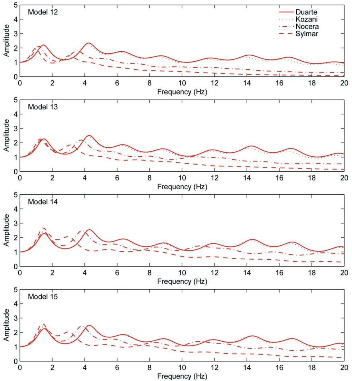
Figure 4-16. Spectral Amplification Functions for Models 12 to 15
