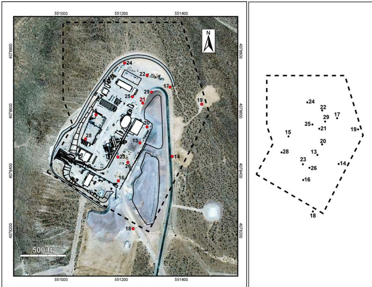
**Figure 3-1. Air Photo of the Proposed Waste Handling Building Site with Overlay That Outlines the Current North Portal Surface Facilities. Dashed Line Outlines the Proposed Waste Handling Building Site. Red Circles Show the Locations of Boreholes Used in the DOE Site Investigation. For Clarity, the Insert to the Right of the Image Also Shows Borehole Locations and the Outline of the Proposed Waste Handling Building Site.**
