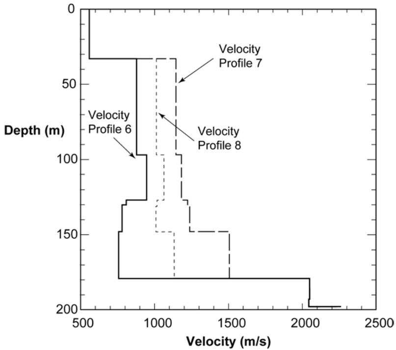
Figure 4-9.  $V_s$  Profiles 6, 7, and 8 Used in the Ground Response Calculations
