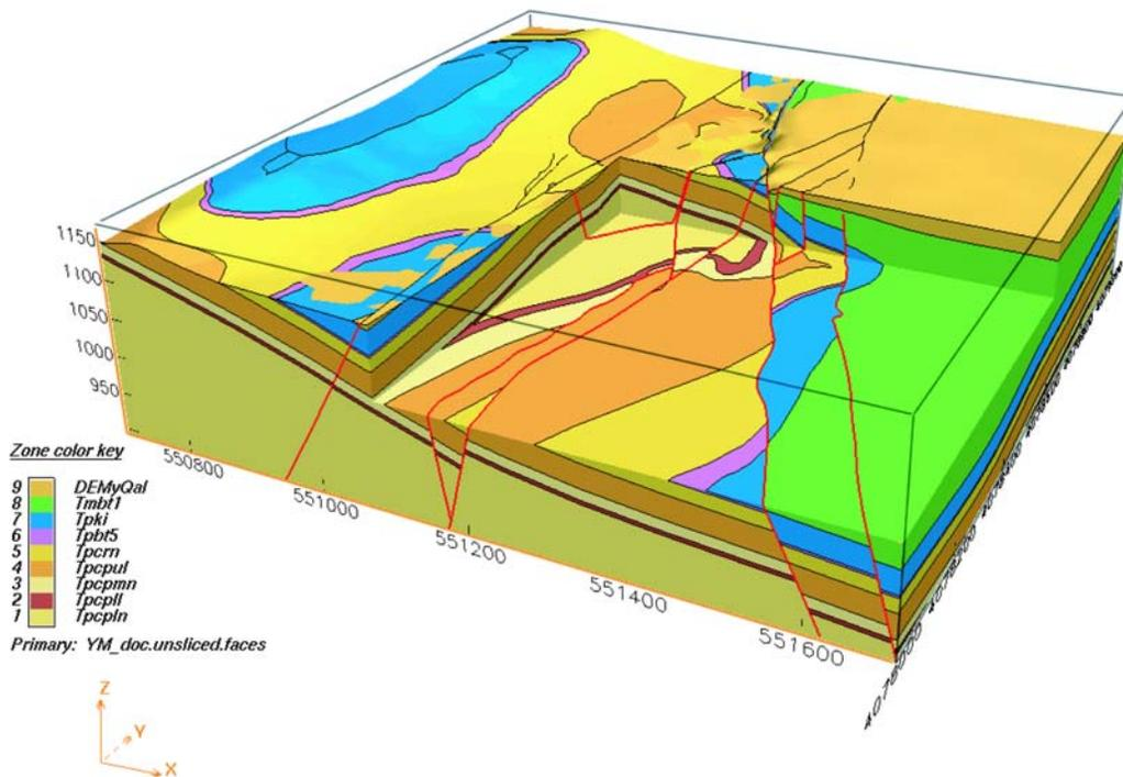
**Figure 2-2. The EarthVision® Model of the Proposed Waste Handling Building Site. No Vertical Exaggeration.**
