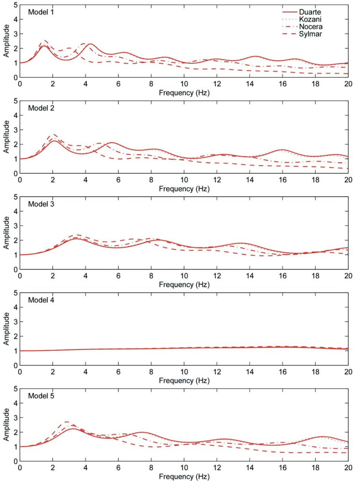
**Figure 4-13. Spectral Amplification Functions for Models 1 to 5**
