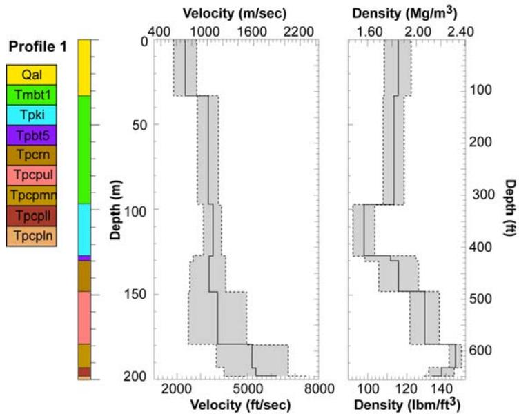
Figure 4-4. Thickness, Velocity, and Density Profile 1 Used in the Ground Response Calculations
