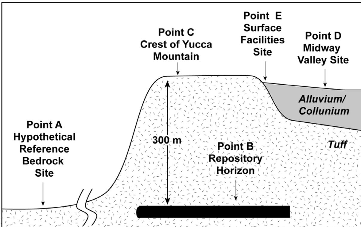
Figure 4-1. Schematic of the Seismic Reference Points At Yucca Mountain (Modified From Stepp, et al., 2001)
