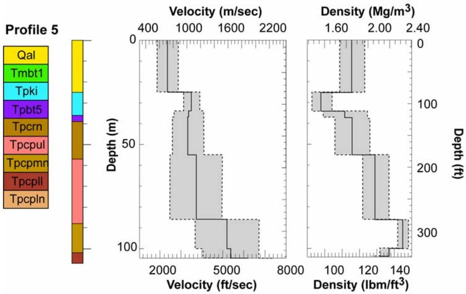
Figure 4-8. Thickness, Velocity, and Density Profile 5 Used in the Ground Response Calculations
