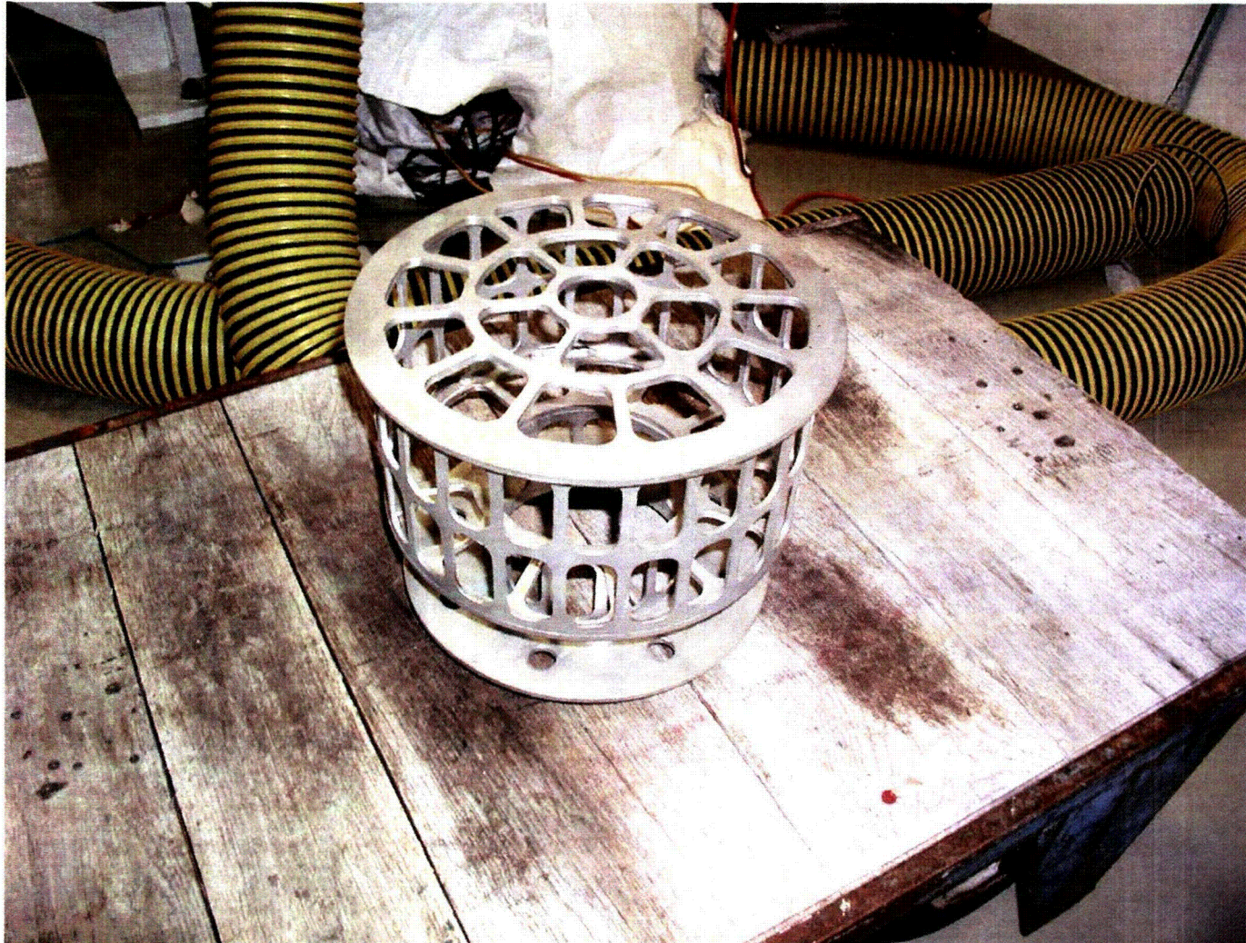
P-3.I.2-2 Six Inch Drain Debris Screen
