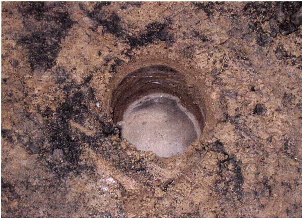
*Figure 7. Photograph of Water Standing in a Test Hole Augered through the CSL and 2 m into Tailings on the Side Slope of the Lakeview Disposal Cell*
