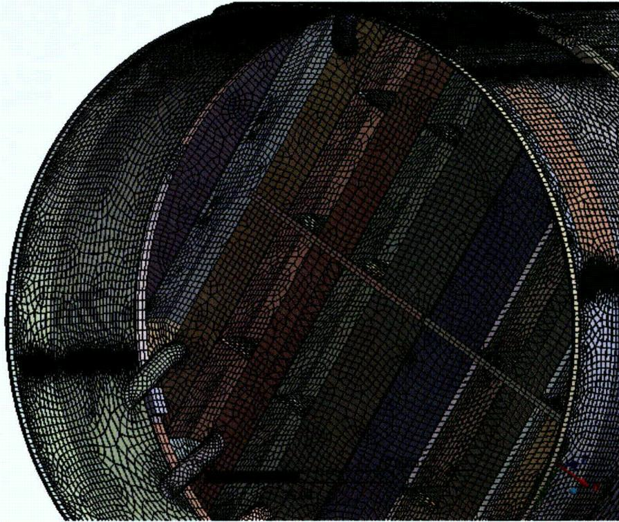
Figure 5c. Close-up of mesh showing drain pipes and hood supports; supporting beams and base plates.
