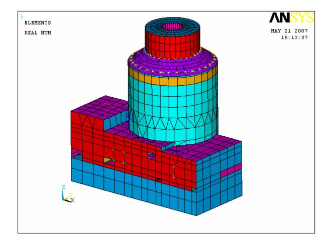
**3D Finite Element Model of Coupled Shield and Auxiliary Building**
