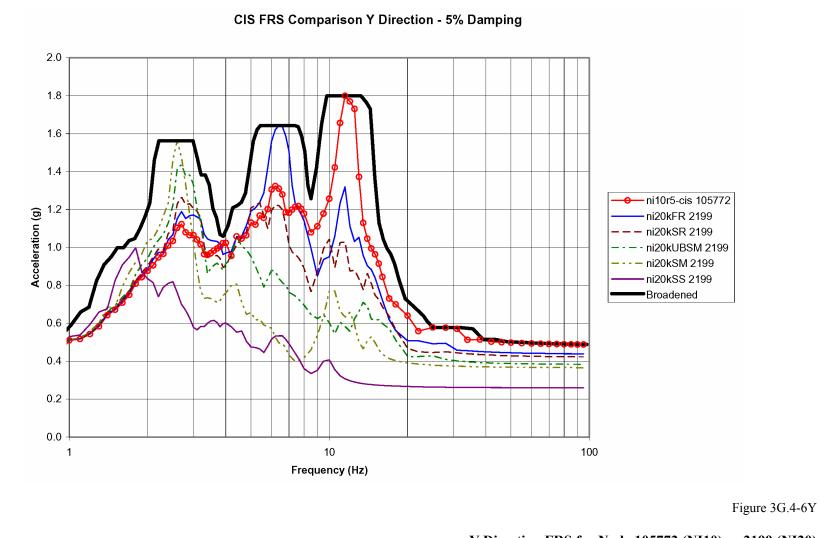
Y Direction FRS for Node 105772 (NI10) or 2199 (NI20) CIS at Operating Deck Elevation 134.25'
