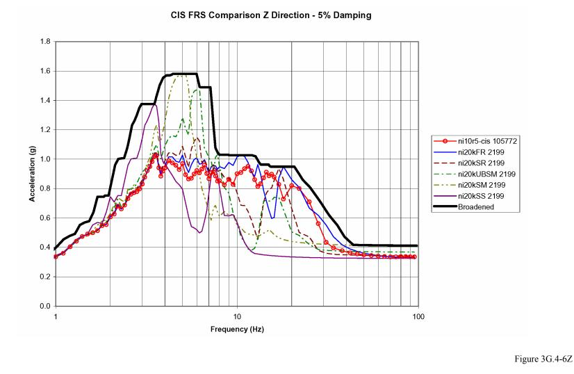
Z Direction FRS for Node 105772 (NI10) or 2199 (NI20) CIS at Operating Deck Elevation 134.25'
