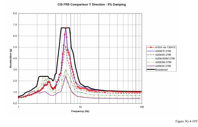
Y Direction FRS for Node 130412 (NI10) or 2788 (NI20) SCV Near Polar Crane Elevation 224.00'
