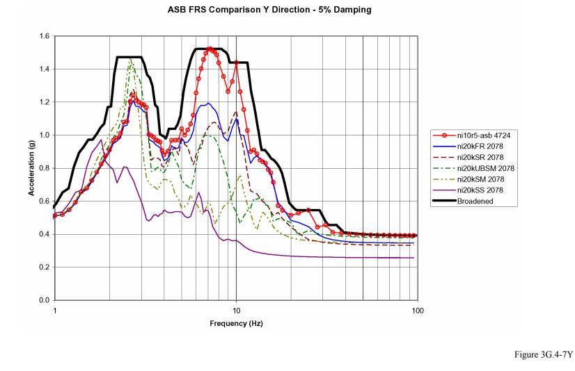
Y Direction FRS for Node 4724 (NI10) or 2078 (NI20) ASB Control Room Side Elevation 134.88'
