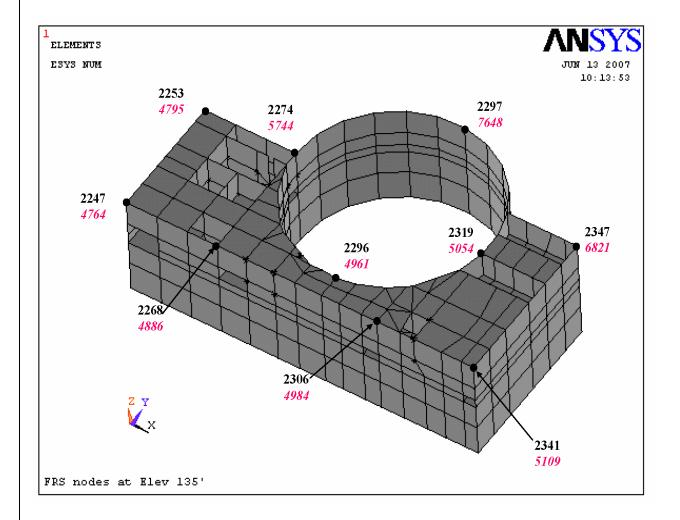
Auxiliary Shield Building "Rigid" Nodes at El. 135'
