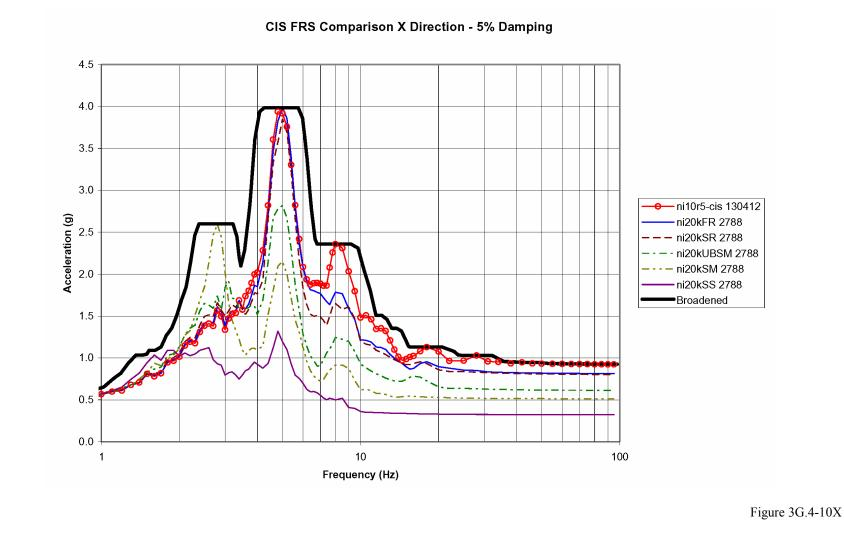
X Direction FRS for Node 130412 (NI10) or 2788 (NI20) SCV Near Polar Crane Elevation 224.00'
