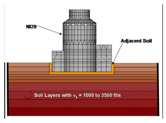
Note: The adjacent soil elements are part of the structural portion of SASSI and have the same material properties as the soil. These elements are used to obtain soil lateral and bearing soil pressures.
