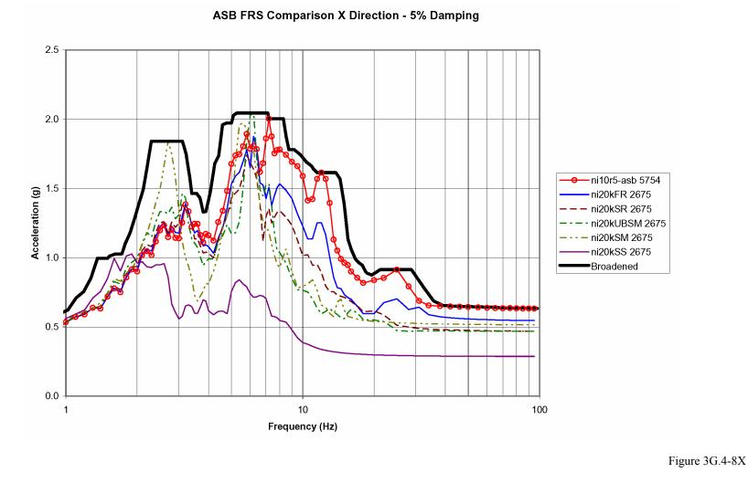
X Direction FRS for Node 5754 (NI10) or 2675 (NI20) ASB Fuel Building Roof Elevation 179.19'
