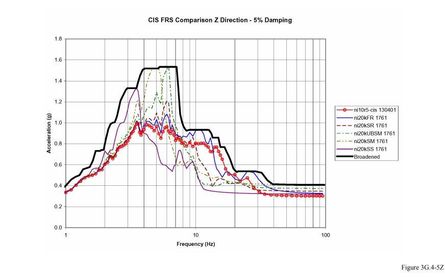
Z Direction FRS for Node 130401 (NI10) or 1761 (NI20) CIS at Reactor Vessel Support Elevation of 100'
