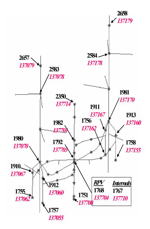
Reactor Coolant Loop Lumped-Mass Stick Model
