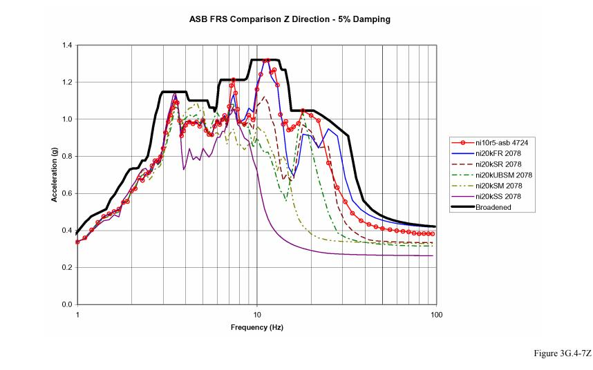
Z Direction FRS for Node 4724 (NI10) or 2078 (NI20) ASB Control Room Side Elevation 134.88'
