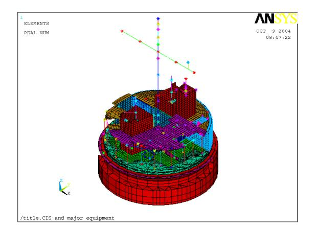
Containment Internal Structure with the SCV, PC, Reactor Coolant Loop, and Pressurizer
