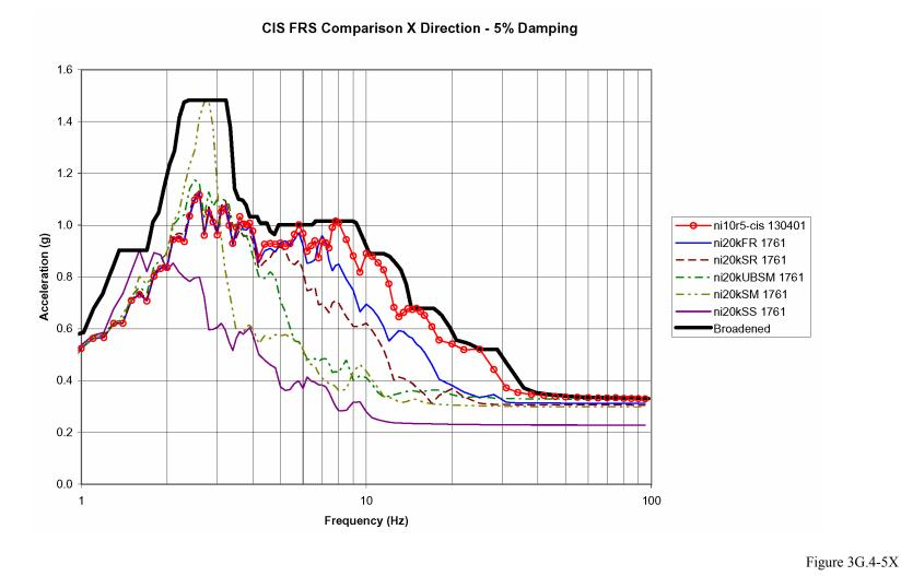
X Direction FRS for Node 130401 (NI10) or 1761 (NI20) CIS at Reactor Vessel Support Elevation of 100'
