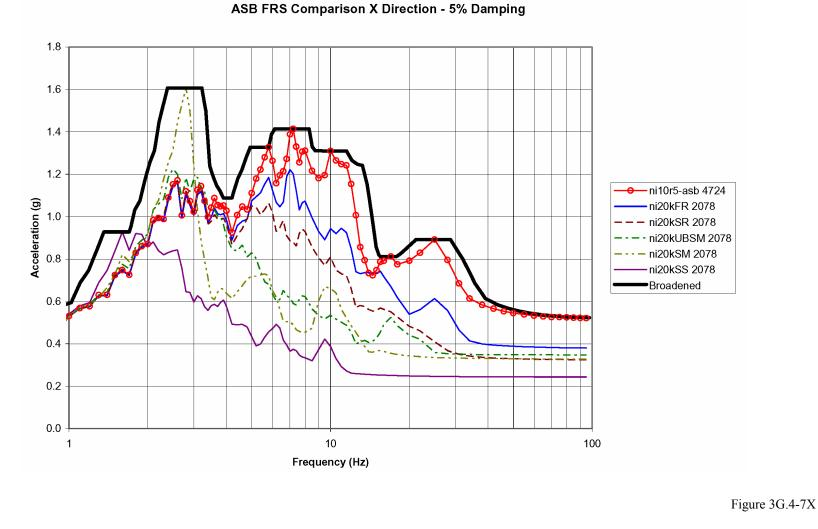
X Direction FRS for Node 4724 (NI10) or 2078 (NI20) ASB Control Room Side Elevation 116.50'
