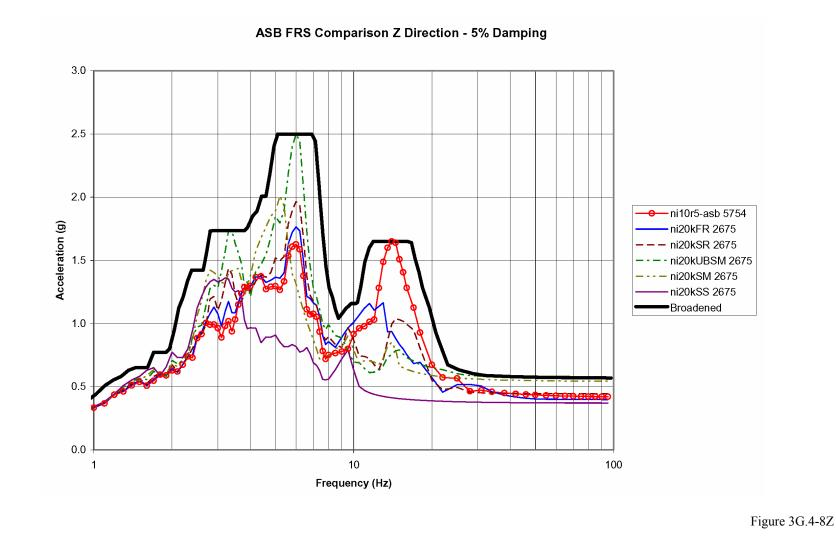
Z Direction FRS for Node 5754 (NI10) or 2675 (NI20) ASB Fuel Building Roof Elevation 179.19'
