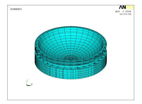
**3D** Finite Element Model of Containment Outer Basemat (Dish)
