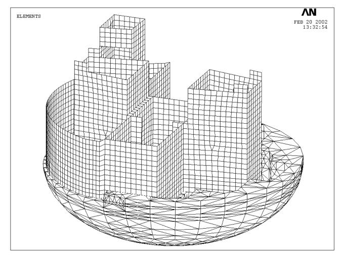
Note: This figure shows the finite element model of walls and basemat inside containment. Floors are not shown.
