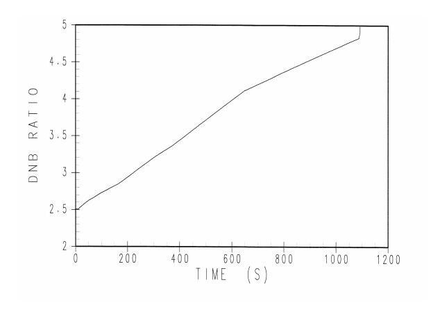
Figure 15.5.2-6 **DNBR Transient for Chemical and Volume Control System Malfunction**
